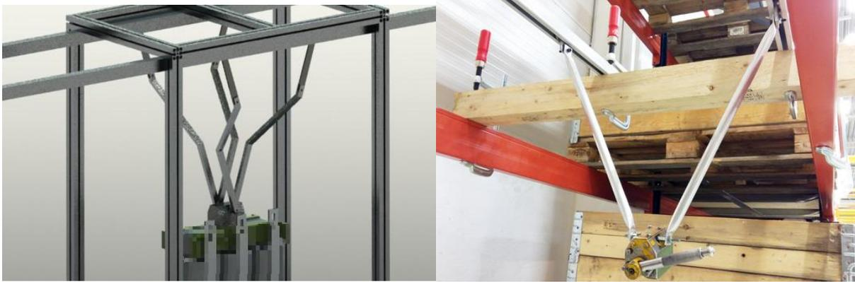
Figure 13. Four-link tipping guard design (on the left) and concept testing rig (on the right)
