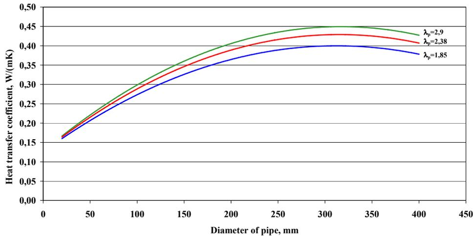
Figure 2.10 Heat transfer coefficient of the underground preinsulated pipe at different heat conductivity of a ground  $\lambda_{pin} = 1,85; 2,38; 2,9 \text{ W/(mK)}$
