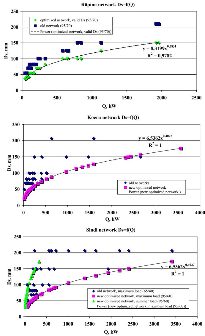
Figure 4.4 Valid and optimal values of internal diameter depending to heat load  $D_s = f(Q)$  (Rápina, Koeru, Sindi)
