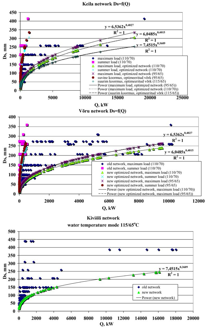
Figure 4.10 Valid and optimal values of internal diameter depending to heat load  $D_s = f(Q)$  (Keila, Võru, Kiviõli networks)
