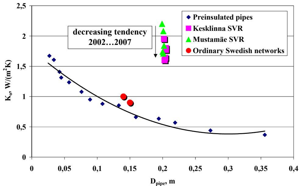
Figure 5.10 The overall heat transfer coefficient reduction tendency in Tallinn DH networks (2002-2007 years)
