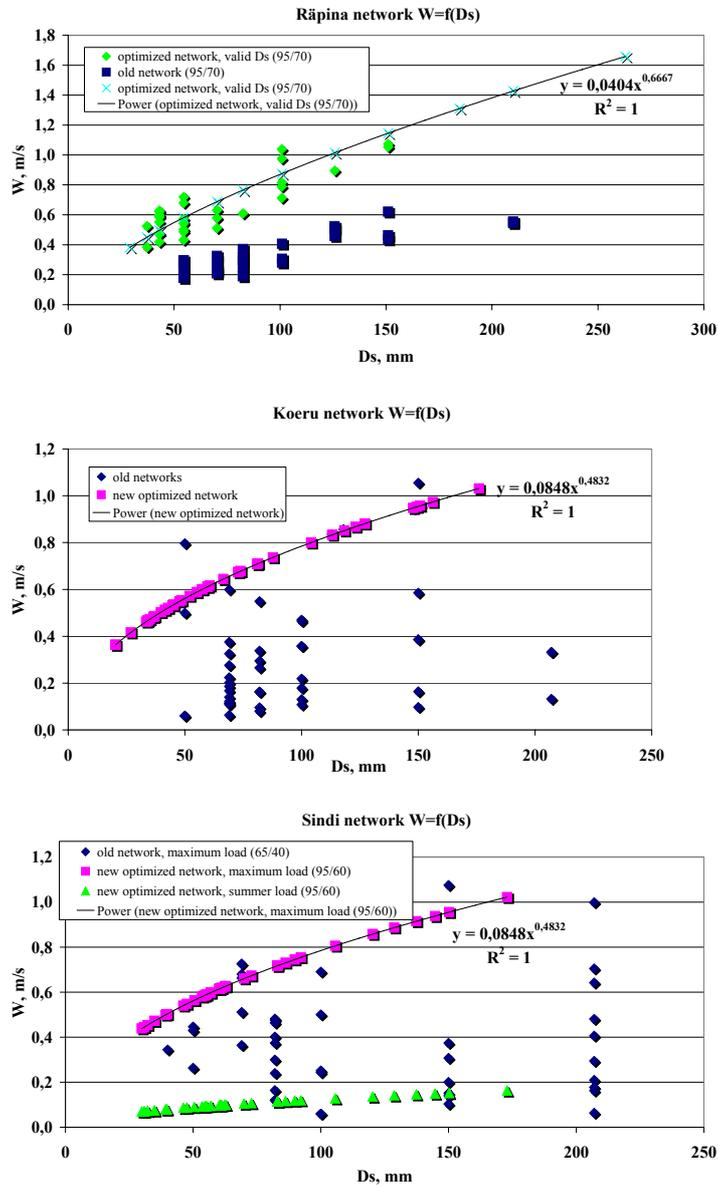
Figure 4.5 Valid and optimal values of water velocity depending to pipe diameter  $W = f(D_s)$  (Rápina, Koeru, Sindi)
