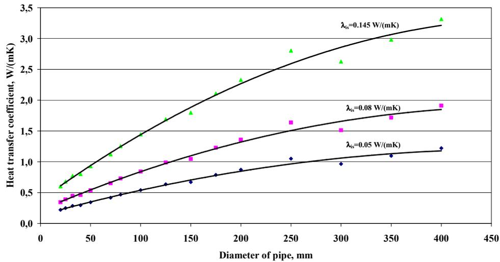
Figure 2.12 Heat transfer coefficient of an air-lining network at different heat conductivity of thermal insulation ( $\lambda_{is} = 0,05; 0,08; 0,145$  W/(mK))
