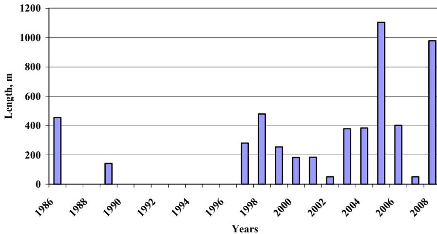
Figure 6.2 Length of the replaced pipelines on years in Lasnamäe network
