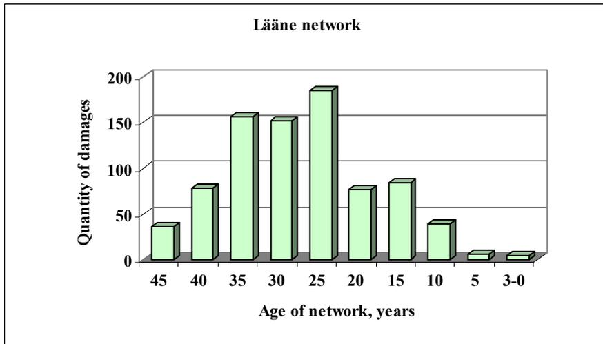
Figure 6.11 Distribution of damages in Lääne district heating network on middle age of a networks sites
