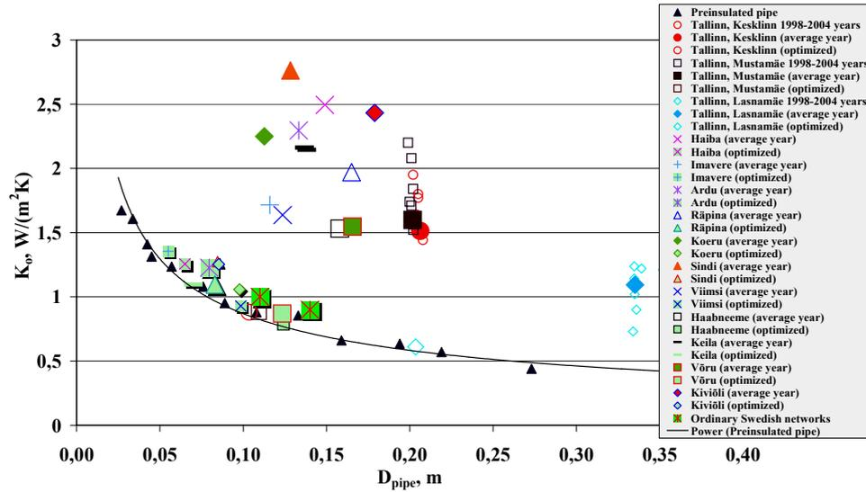
Figure 5.3 Total overall heat transfer coefficient for old and new optimized Estonian district heating systems, depending on the average diameter of the pipes (1998-2009 years)
