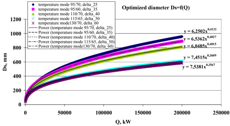
Figure 4.16 Optimal diameter depending to heat load  $D_s = f(Q)$
