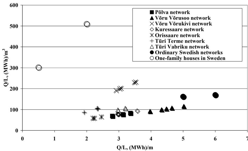
Figure 5.2 The specific volume heat supply for different parts of district heating systems in small Estonian towns depending on the specific heat supply (1998-2002 years)
