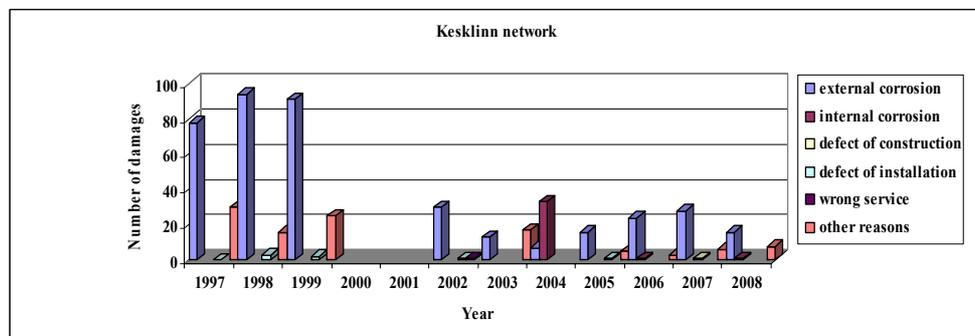
Figure 6.22 The character of damages in Kesklinn network
