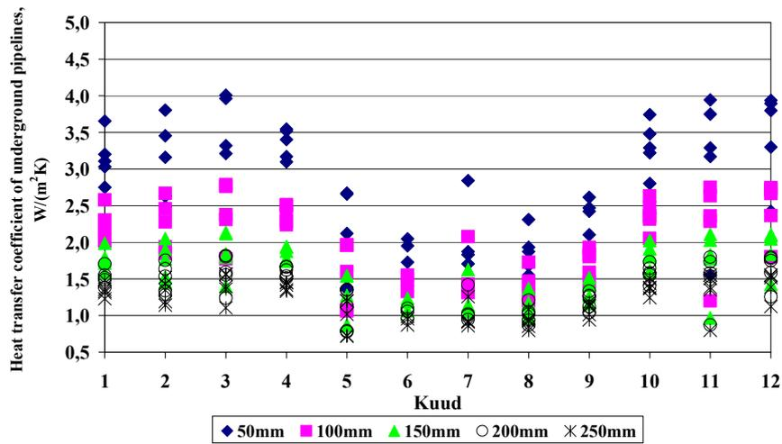
Figure 5.5. Heat transfer coefficient for Võru town Võrusoo network pipes depending on the climate condition differences (rainwater) during the year
