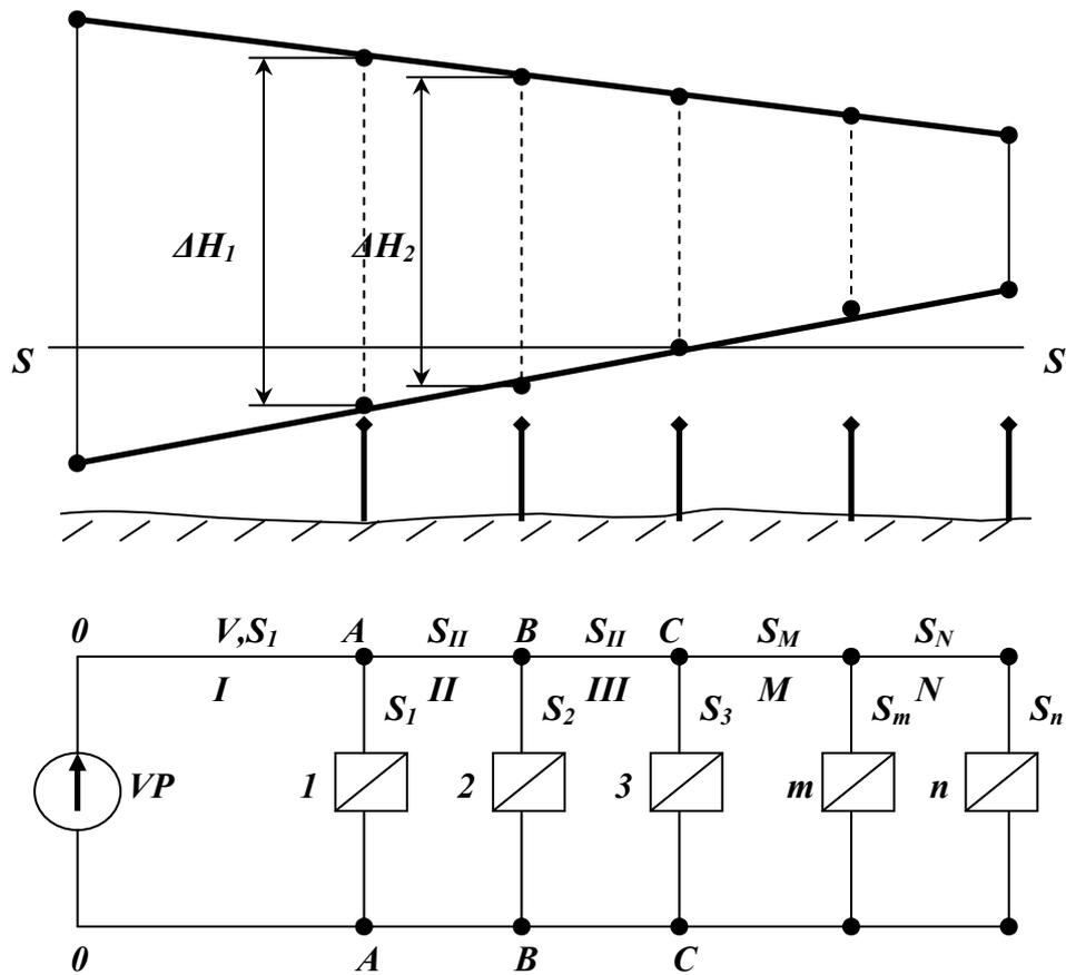
Figure 2.2 The scheme of a DH network with one heat source and piezometric schedule (where  $\Delta H_1$  and  $\Delta H_2$  valid heads of water in  $mH_2O$  accordingly at consumers 1 and 2)
