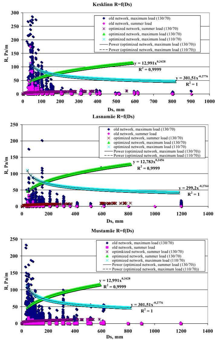
Figure 4.15 Valid and optimal values of friction losses depending to pipe diameter  $R_l = f(D_s)$  ( Kesklinna, Lasnamäe, Mustamäe-Õismäe )
