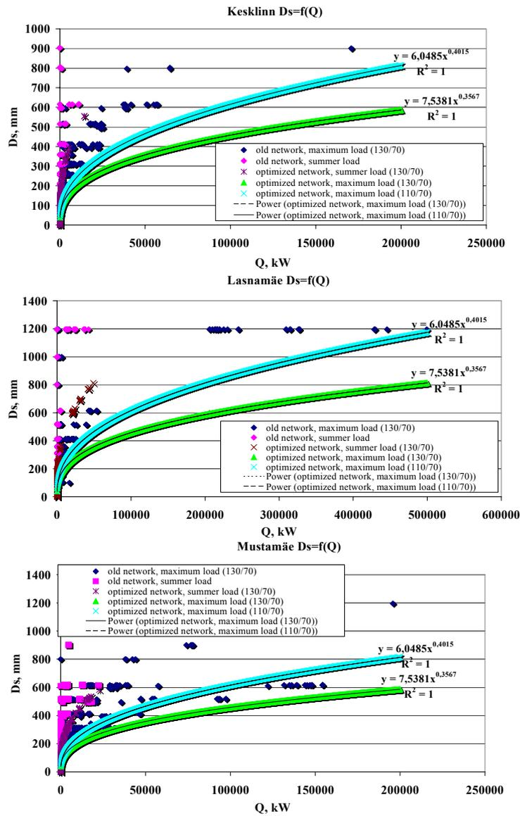
Figure 4.13 Valid and optimal values of internal diameter depending to heat load  $D_s = f(Q)$  (Kesklinna, Lasnamäe and Mustamäe-Õismäe networks)
