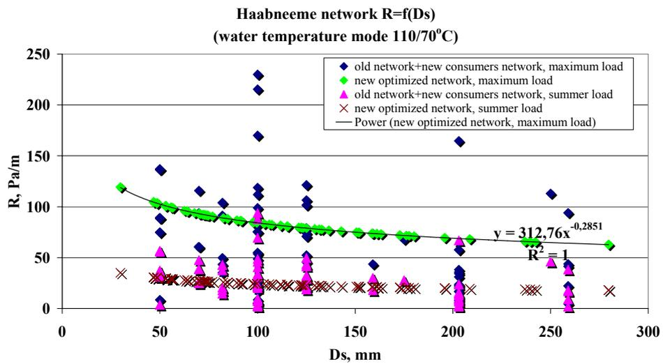
Figure 4.9 Valid and optimal values of friction losses depending to pipe diameter  $R_l = f(D_s)$  (Viimsi, Haabneeme)
