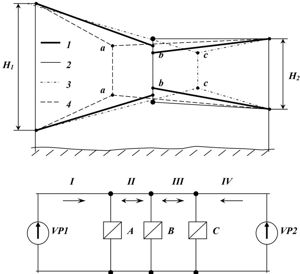
Figure 2.4 The ring network with two heat supply sources and piezometric schedule (1 – at any way chosen watershed in a point B in at  $\Delta P > 0$ ; 2 – at any way chosen watershed in a point B in at  $\Delta P < 0$ ; 3 – at displacement of a watershed in a point C; 4 – at displacement of a watershed in a point A)
