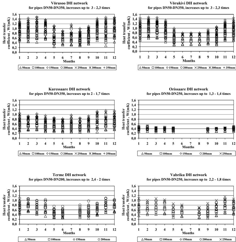
Figure 3.3 Changes in insulation heat transfer coefficient of an old underground network (on a running meter)
