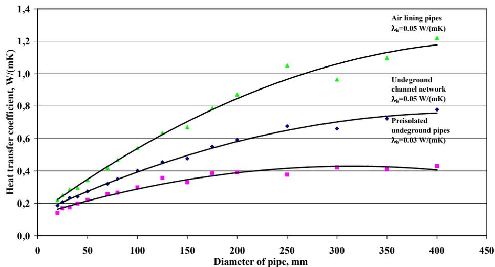
Figure 2.13 Heat transfer coefficient of pipes for various lining
