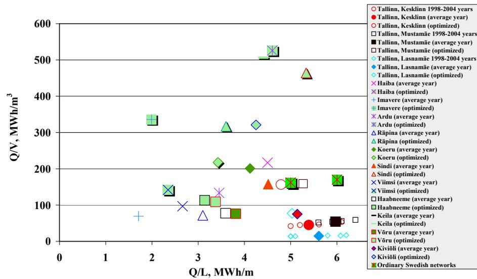
Figure 5.4 The specific volume heat supply for old and new optimized Estonian district heating networks depending on the specific length heat supply (1998-2009 years)
