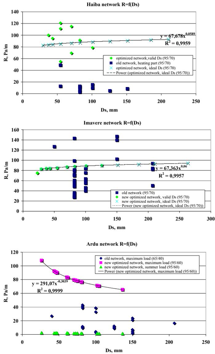
Figure 4.3 Valid and optimal values of friction losses depending to pipe diameter  $R_l = f(D_s)$  (Haiba, Imavere, Ardu)
