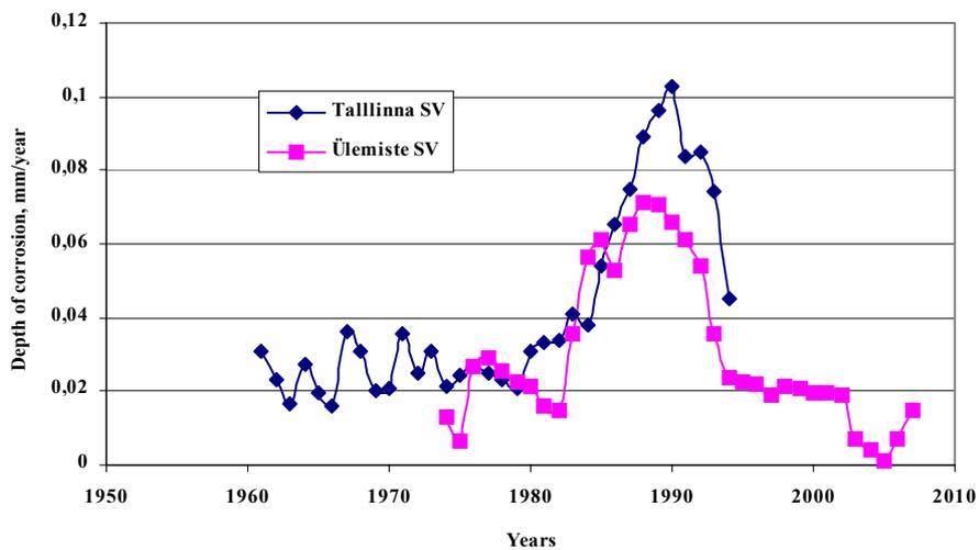
Figure 6.18 Depth of pipes internal corrosion [mm/year] in Tallinn and Ülemiste networks
