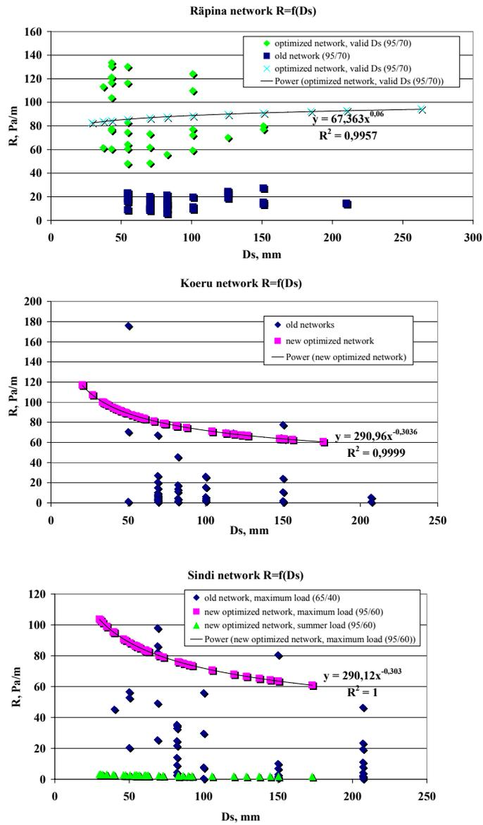
Figure 4.6 Valid and optimal values of friction losses depending to pipe diameter  $R_l = f(D_s)$  (Rápina, Koeru, Sindi)
