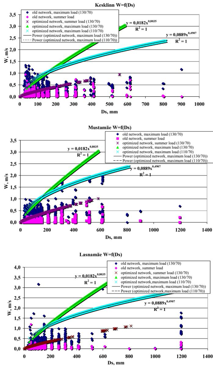
Figure 4.14 Valid and optimal values of water velocity depending to pipe diameter  $W = f(D_s)$  (Kesklinna, Lasnamäe and Mustamäe-Õismäe networks)
