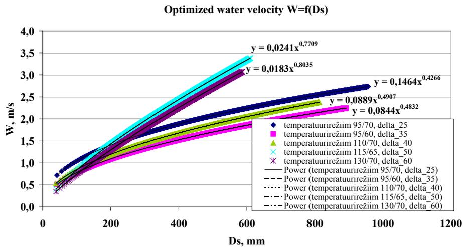
Figure 4.18 Optimal velocity of water depending to pipe diameter  $W = f(D_s)$
