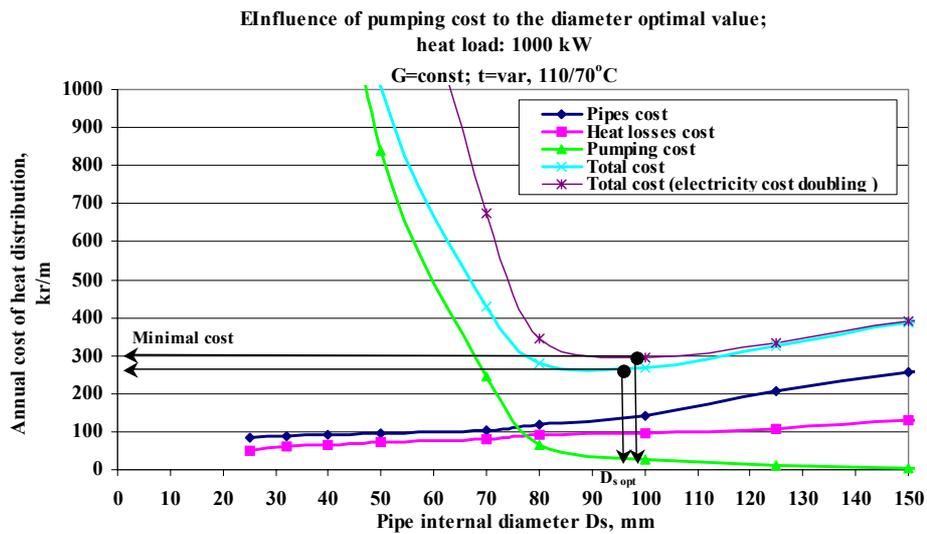
Figure 2.18 Influence of pumping cost to the diameter optimal value
