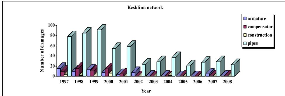
Figure 6.21 The place of damages on elements of a Kesklinn network
