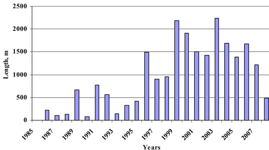
Figure 6.15 Length of the replaced pipelines on years in Kesklinn area network
