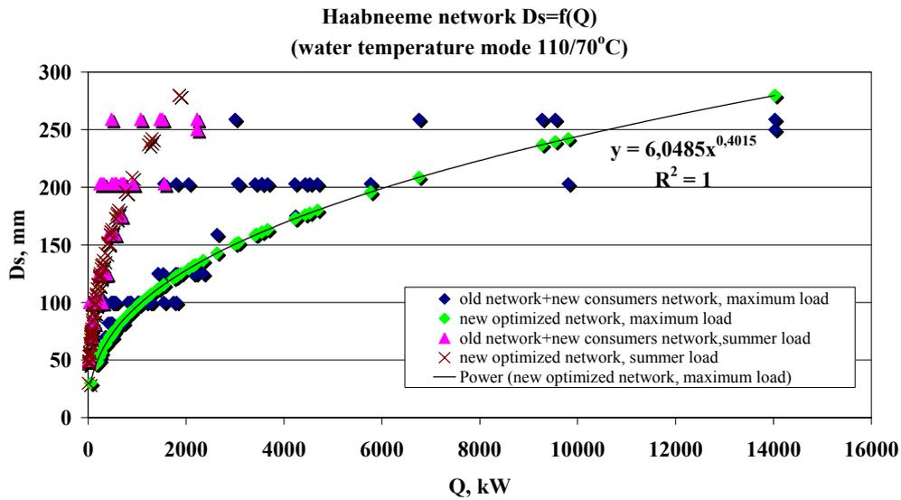
Figure 4.7 Valid and optimal values of internal diameter depending to heat load  $D_s = f(Q)$  (Viimsi, Haabneeme)
