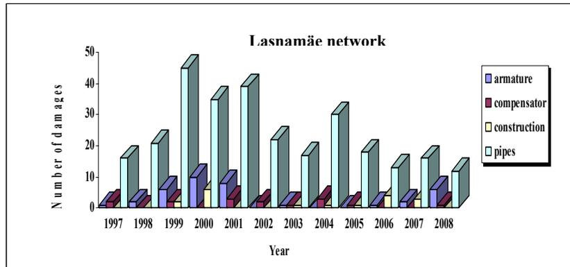
Figure 6.5 The place of damages on elements in a Lasnamäe network
