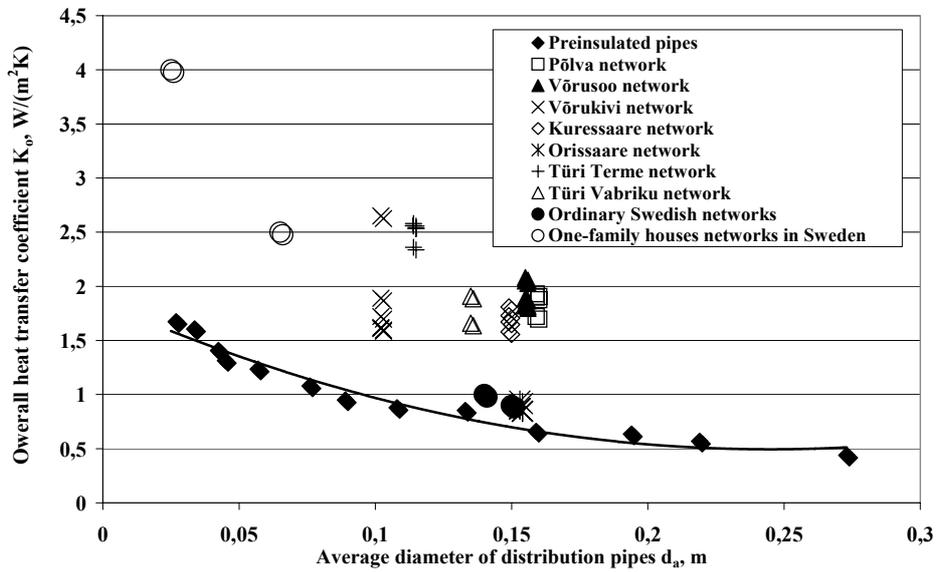
Figure 5.1 Total overall heat transfer coefficient for different district heating systems in small Estonian towns depending on the average diameter of pipes (1998-2002 years)
