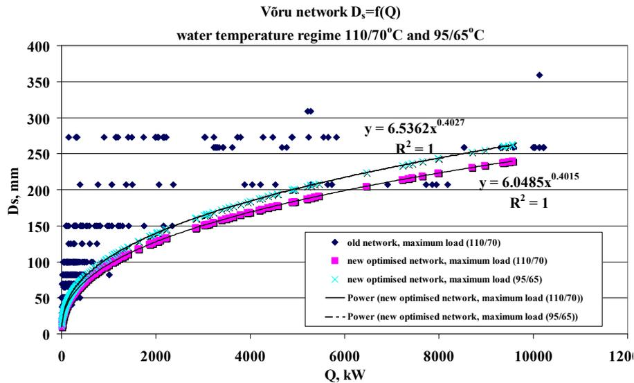
Figure 5.7 Optimal diameter depending to heat load  $D_s = f(Q)$  in Võru town DH network
