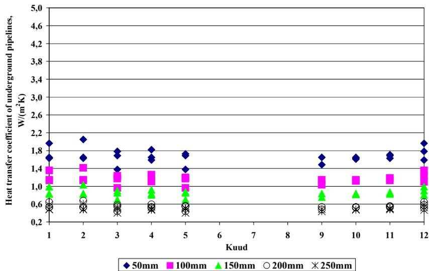
Figure 5.6. Heat transfer coefficient for Orissare town network pipes depending on the climate condition differences (rainwater) during the year
