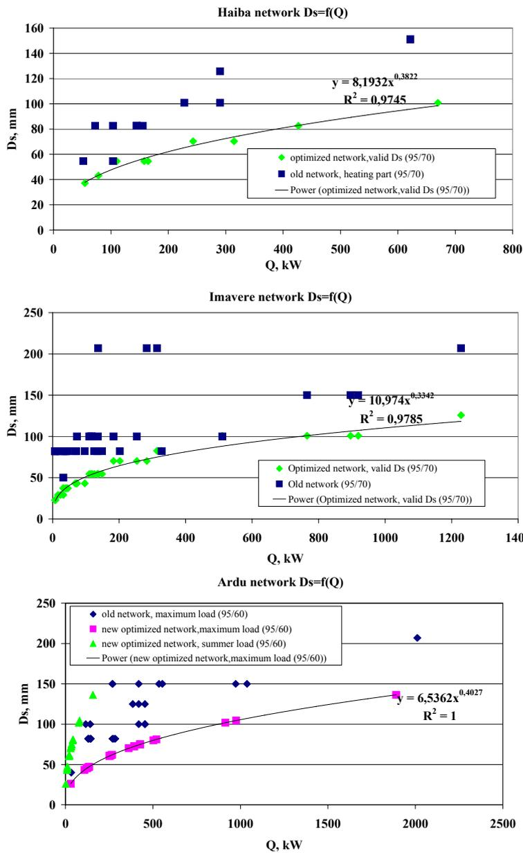
Figure 4.1 Valid and optimal values of internal diameter depending to heat load  $D_s = f(Q)$  (Haiba, Imavere, Ardu)
