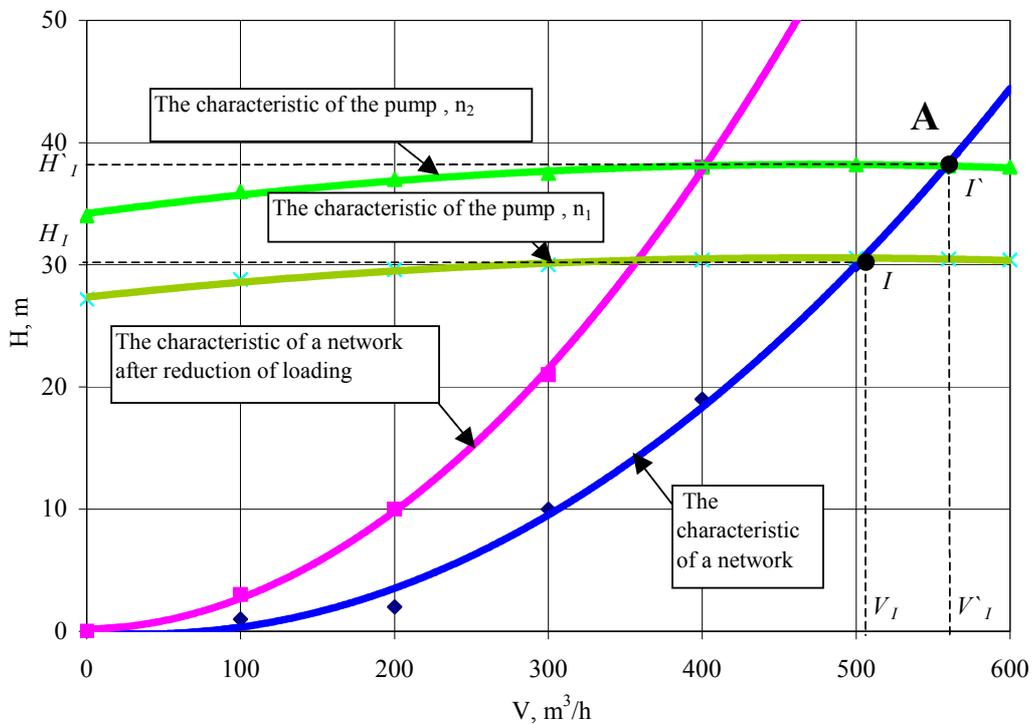
Figure 2.1 The characteristic of a network and the pump
