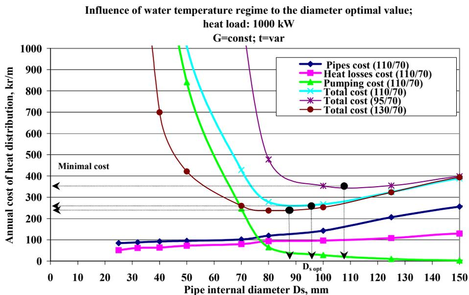
Figure 2.16 Influence of water temperature mode to the diameter optimal value
