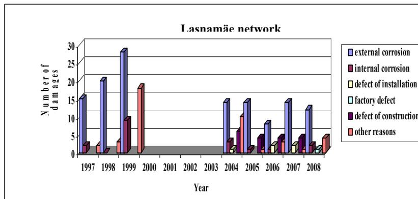
Figure 6.6 The character of damages in Lasnamäe network
