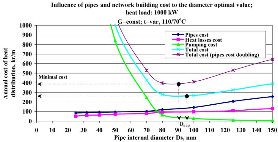
Figure 2.17 Influence of pipes and network building costs to the diameter optimal value
