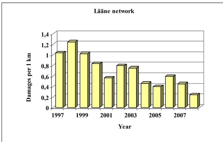
Figure 6.12 Statistics of damages quantity on one kilometre in Lääne network
