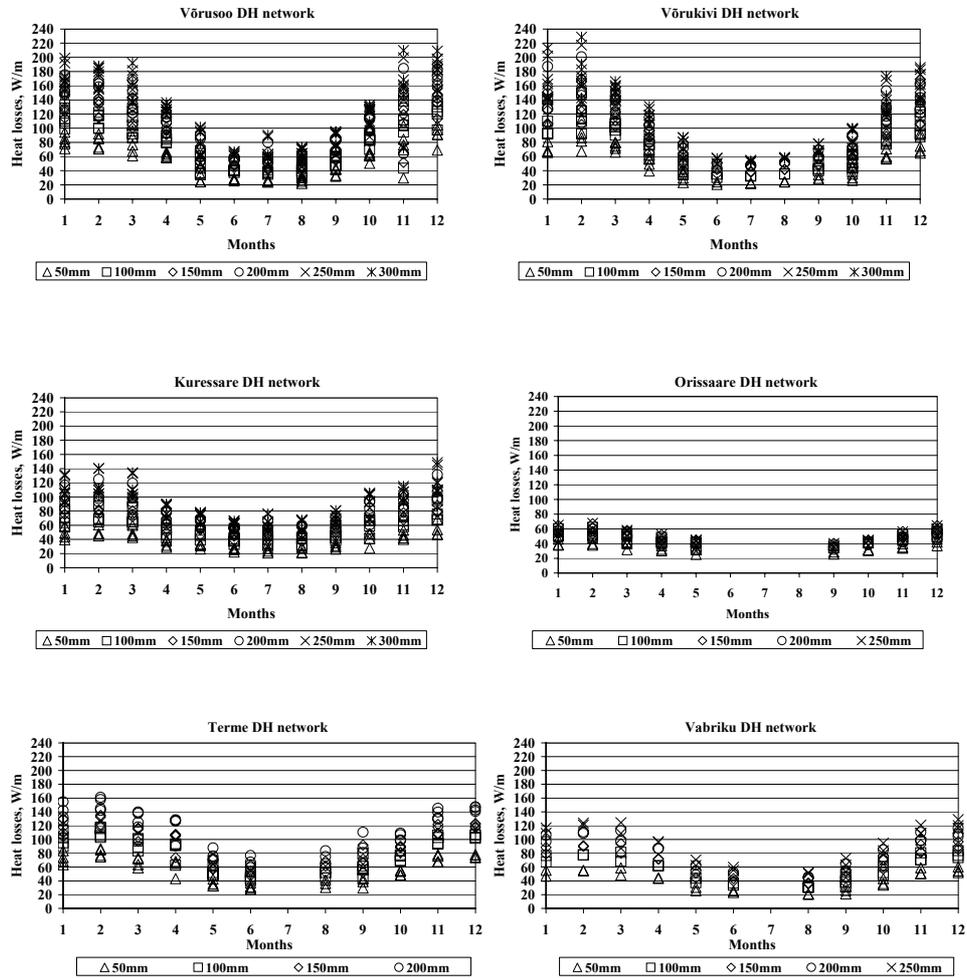
Figure 3.5 Heat losses of an old underground network
