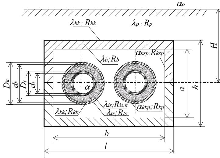
Figure 2.6 The underground network lying in the concrete channel
