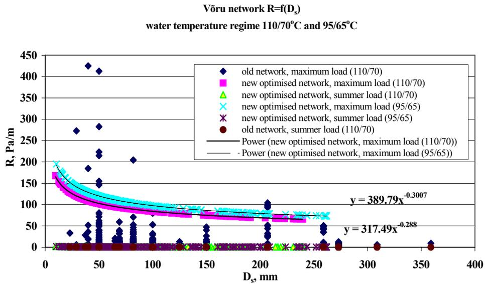
Figure 5.9 Friction losses in Võru town DH network depending to pipe diameter
