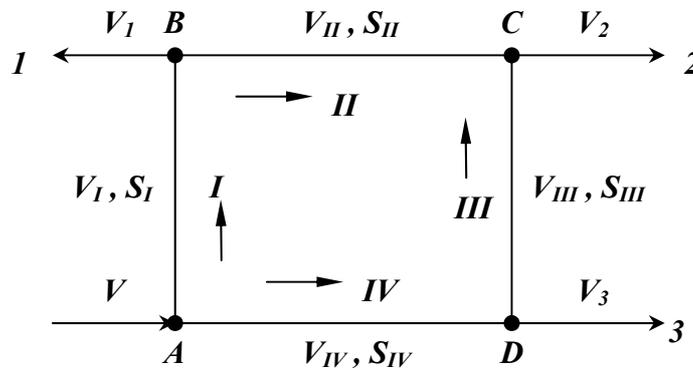
Figure 2.3 The scheme of a ring network with one source of heat
