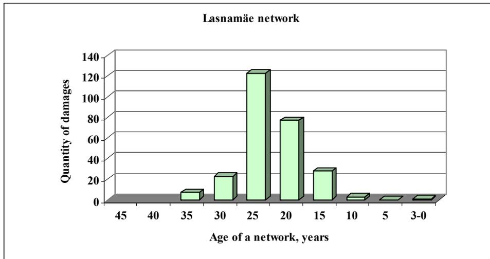
Figure 6.3 Distribution of damages in Lasnamäe district heating network on middle age of a networks sites
