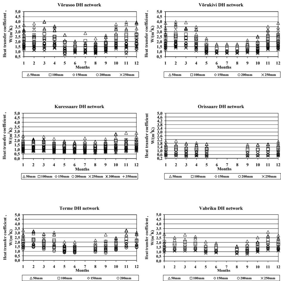
Figure 3.4 Changes in insulation heat transfer coefficient of an old underground network (on square meter)
