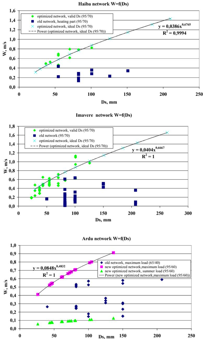
Figure 4.2 Valid and optimal values of water velocity depending to pipe diameter  $W = f(D_s)$  (Haiba, Imavere, Ardu)
