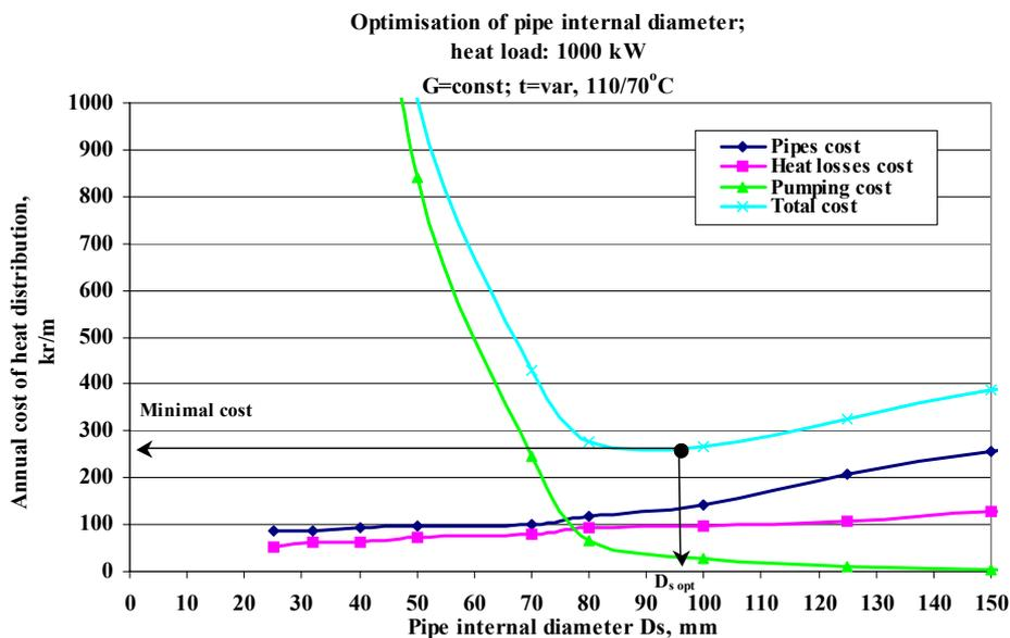
Figure 2.15 Example of pipes diameter optimization
