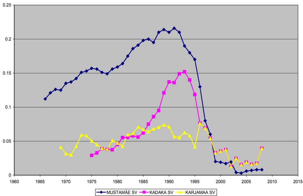
Figure 6.10 Depth of pipes internal corrosion [mm/year] in Mustamäe, Kadaka and Karjamaa networks
