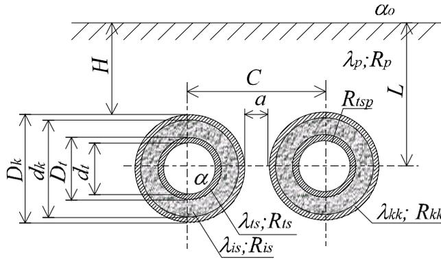
Figure 2.9 Underground network from the preinsulated pipes
