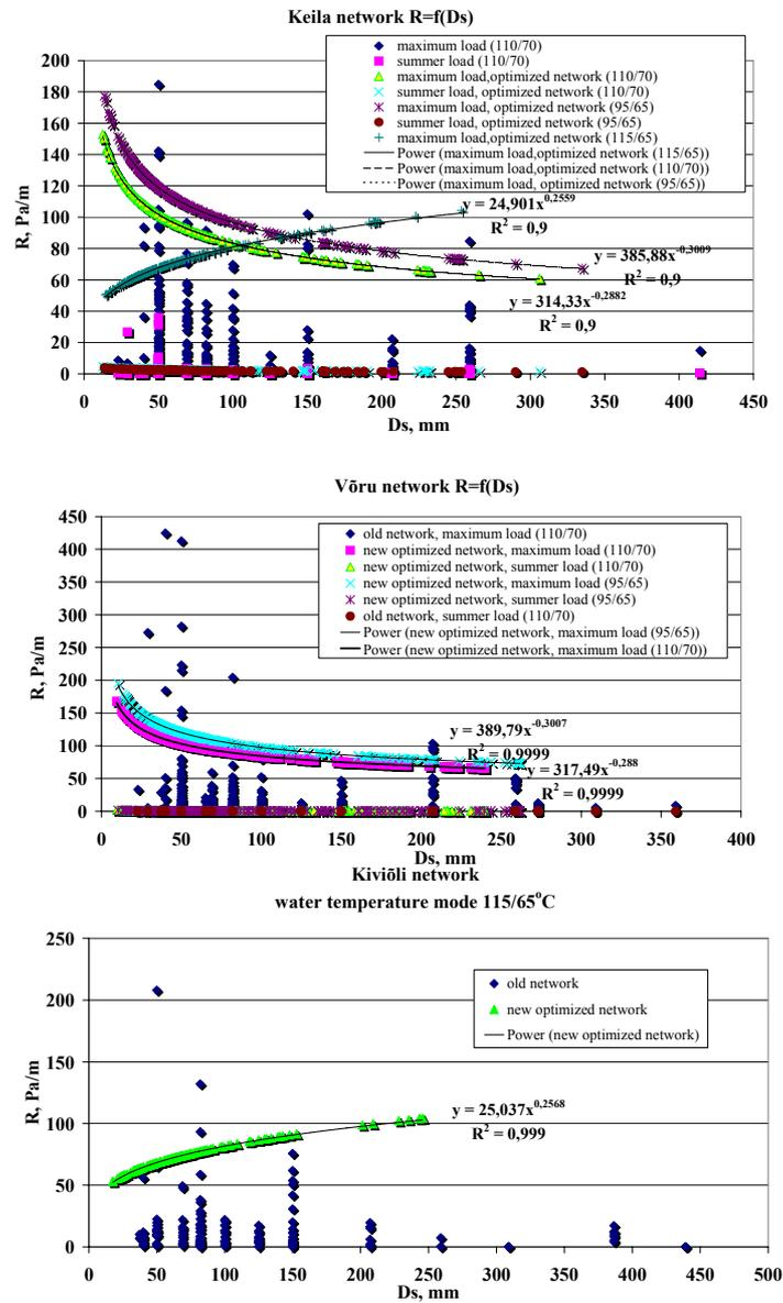
Figure 4.12 Valid and optimal values of friction losses depending to pipe diameter  $R_f = f(D_s)$  (Keila, Võru, Kiviõli networks)
