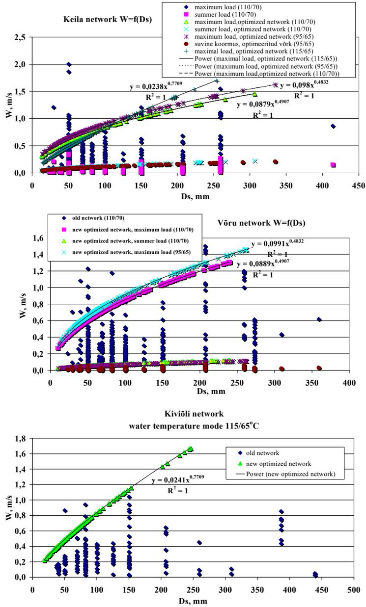
Figure 4.11 Valid and optimal values of water velocity depending to pipe diameter  $W = f(D_s)$  (Keila, Võru, Kiviõli networks)
