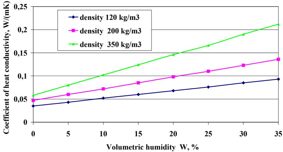
Figure 2.7 Coefficient of heat conductivity of mineral wool depending on volumetric humidity at temperature 30°C [35].
