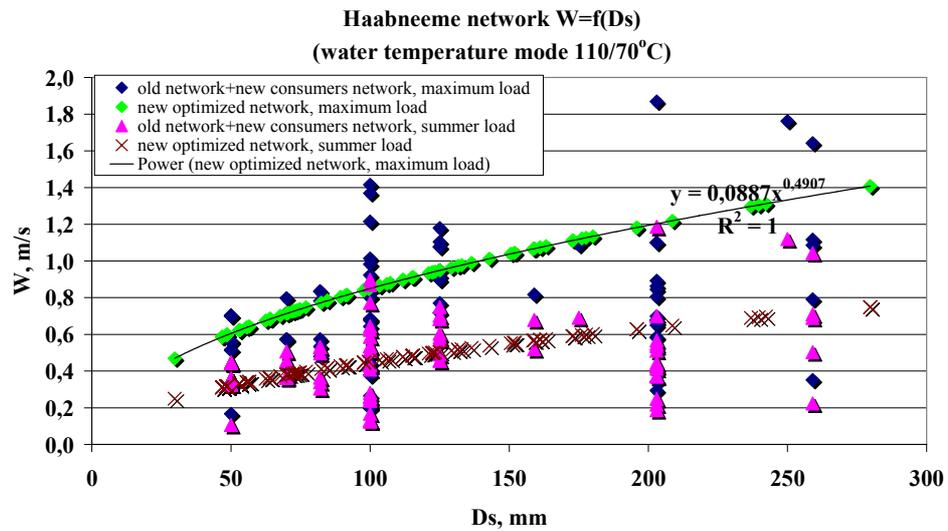
Figure 4.8 Valid and optimal values of water velocity depending to pipe diameter  $W = f(D_s)$  (Viimsi, Haabneeme)
