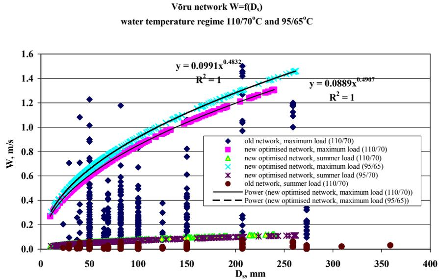
Figure 5.8 Water velocity depending to pipe diameter  $W = f(D_s)$  in Võru town DH network
