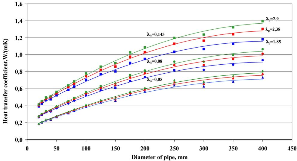
Figure 2.8 The heat transfer coefficient for a pipe of a underground network at different humidity of a ground ( $\lambda_{pin} = 1,85; 2,38; 2,9 \text{ W/(mK)}$ ) and thermal insulation ( $\lambda_{is} = 0,05; 0,08; 0,145 \text{ W/(mK)}$ )
