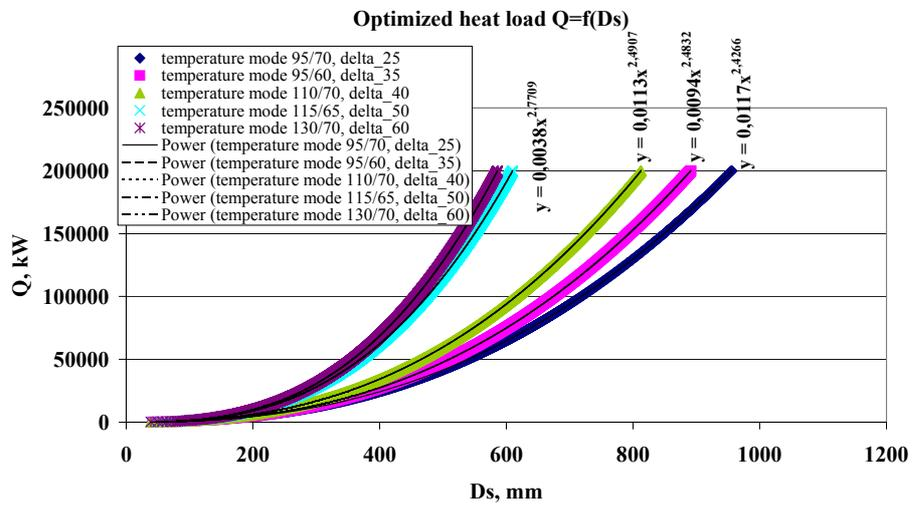
Figure 4.17 Optimal heat load depending to pipe diameter  $Q = f(D_s)$
