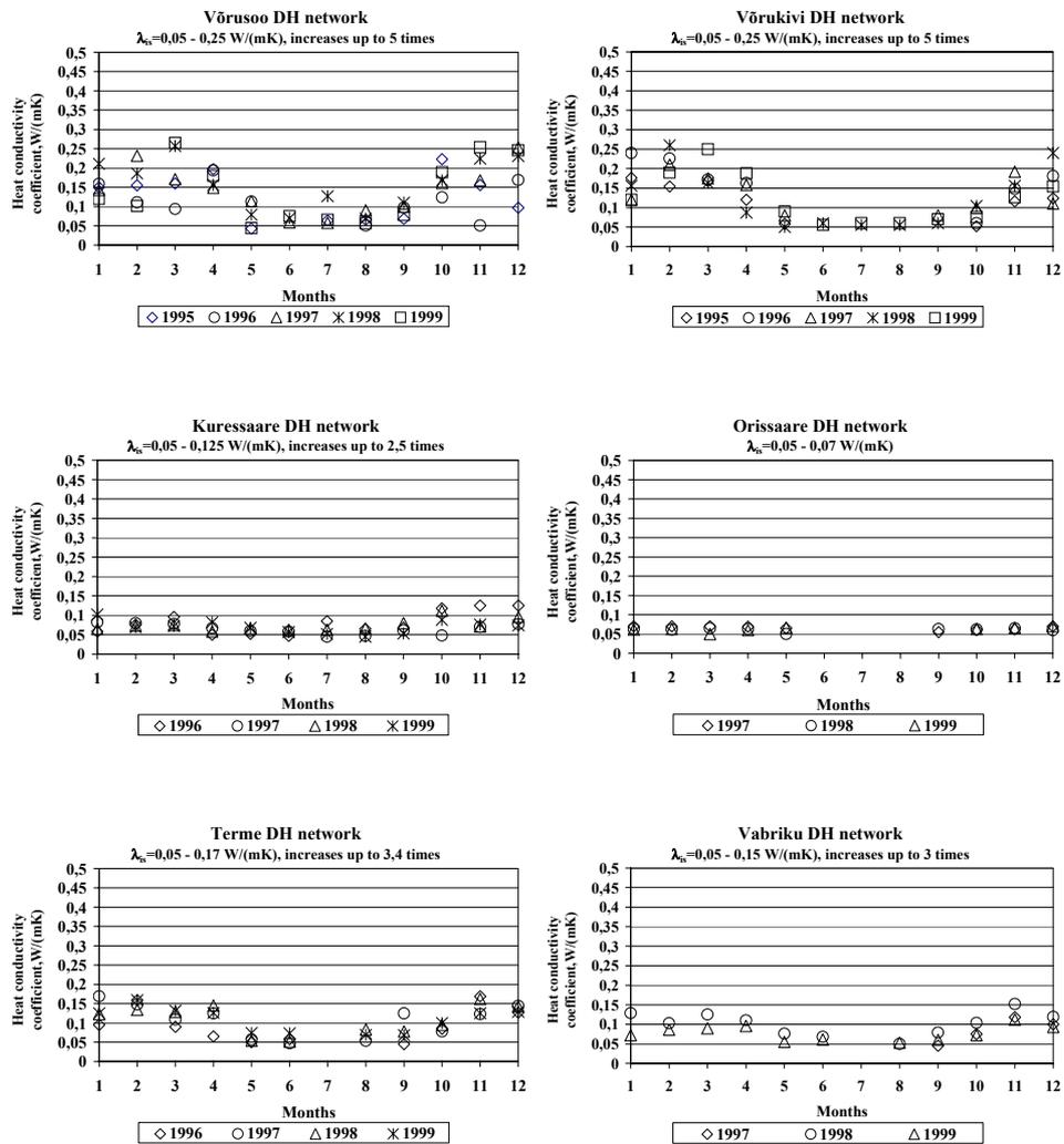
Figure 3.2 Changes in insulation heat conductivity of old underground networks
