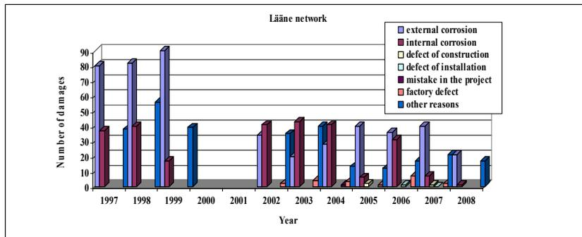
Figure 6.14 The character of damages in Lääne network
