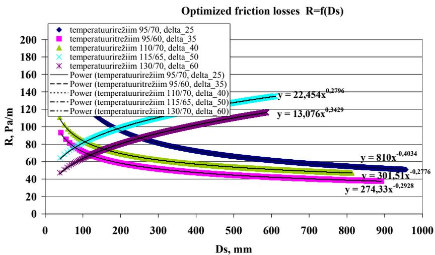
Figure 4.19 Optimal friction depending to pipe diameter  $R_f = f(D_s)$
