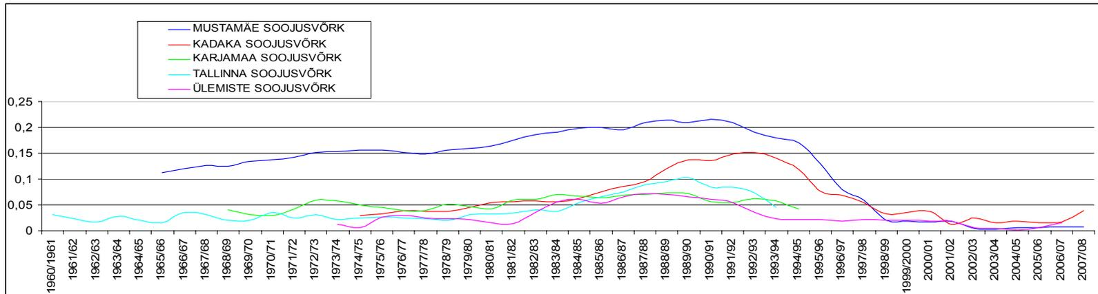
Figure 6.23 Internal corrosion in Mustamäe, Kadaka, Karjamaa, Tallinna and Ülemiste district heating networks in period 1961-2000 years, mm/year
