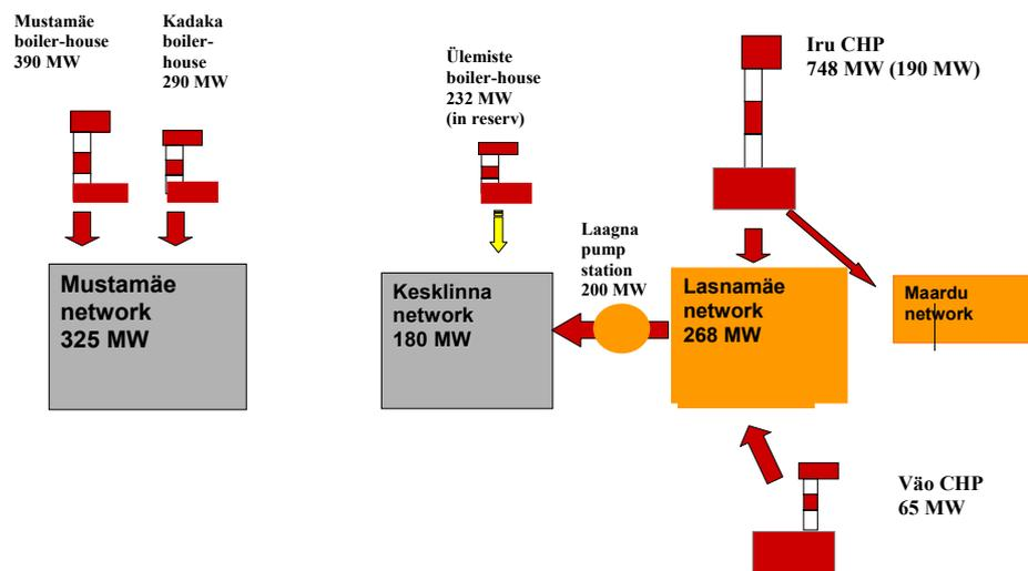
Figure 6.1 The basic scheme of a heat supply in Tallinn and Maardu
