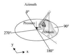
Figure 3. The raw data of each handwriting sample derived from a tablet [26].
