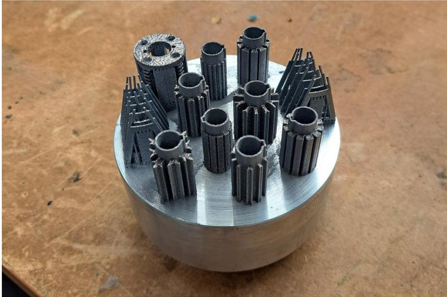
Figure 3.2. SLM printed heatsink designs attached to the build platform.
