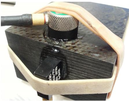
Figure 3 – CFRP block in the test configuration with the transmitting transducer at the side and the receiving transducer on top. Figure from Publication II.
