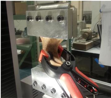
Figure 12 – Skin sample in the loading machine with ultrasonic transducers attached by a hand clamp. Figure from Publication IV.
