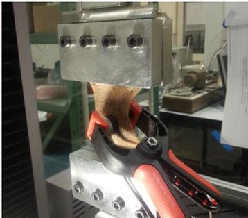
Figure 12 – Skin sample in the loading machine with ultrasonic transducers attached by a hand clamp. Figure from Publication IV.
