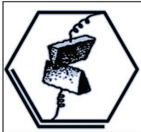
Fig. 1. Some kind of the carborundum wave-responsive devices patented by General H.H.C. Dunwoody [2]
