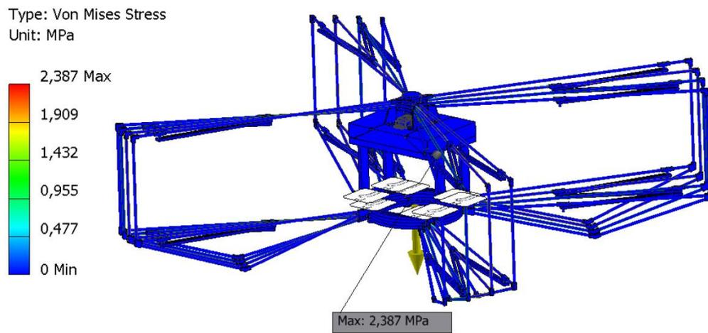
Figure A.3 Simulation results of Von Mises Stress in closed stage without additional load
