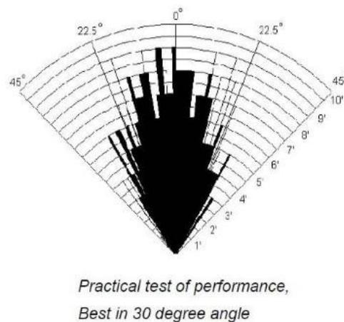
Figure 2.4 Ultrasonic sensor HC-SR04 detection performance. Best performance angle 30-degree [7]
