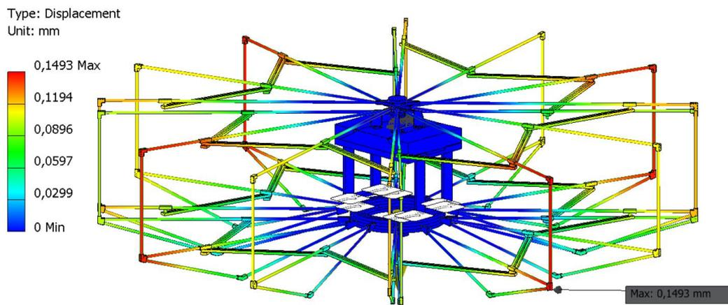
Figure A.1 Simulation results of displacement in opened stage without additional load
