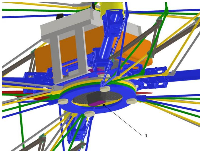
Figure 3.24 View of the sensor paced on the bottom side of the cage 1) TFmini Plus
