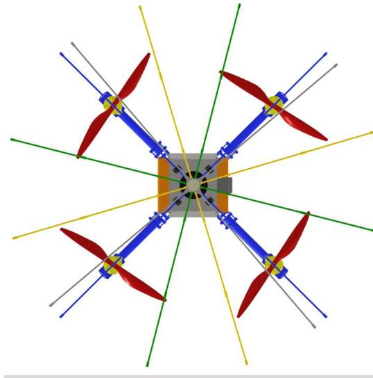
Figure 3.16 Position of frames in open stage. Gray – lead frame, orange, red – ordinary frames, blue – fixed frame
