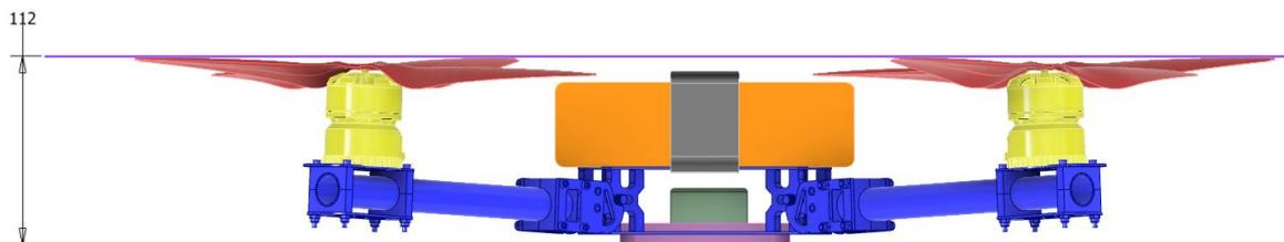
Figure 3.3 Front view of drone with dimension of height from the mounting plate to the ends of propellers in mm
