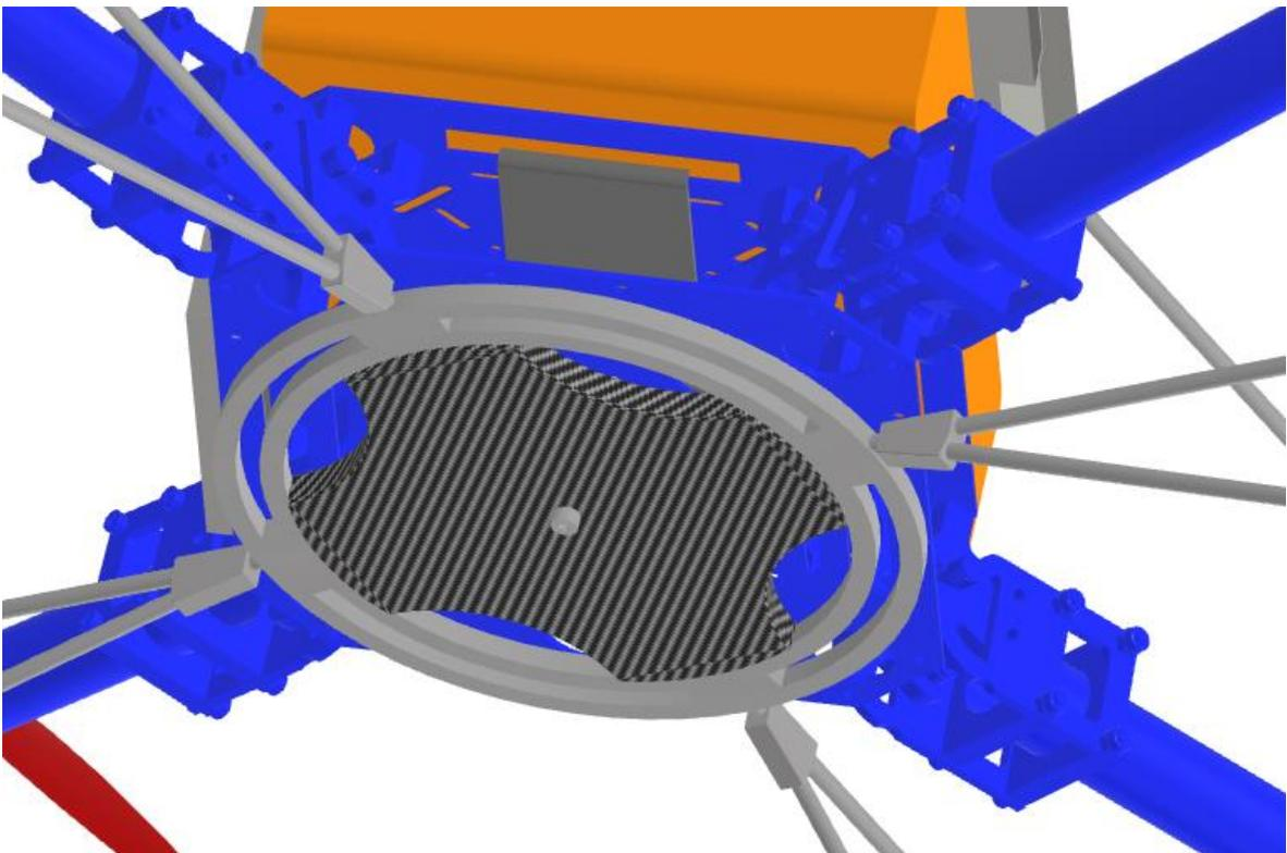
Figure 3.20 Special plate for connection servomotor and movable frame.
