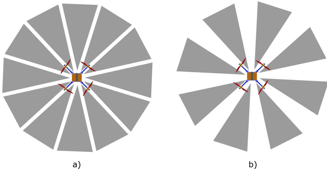
Figure 4.1 Areas of sensors detection around the drone: a) 12 sensors, b) 8 sensors. In case of using 8 sensors case, the detection area will be 33% less than using 12 sensors solution.
