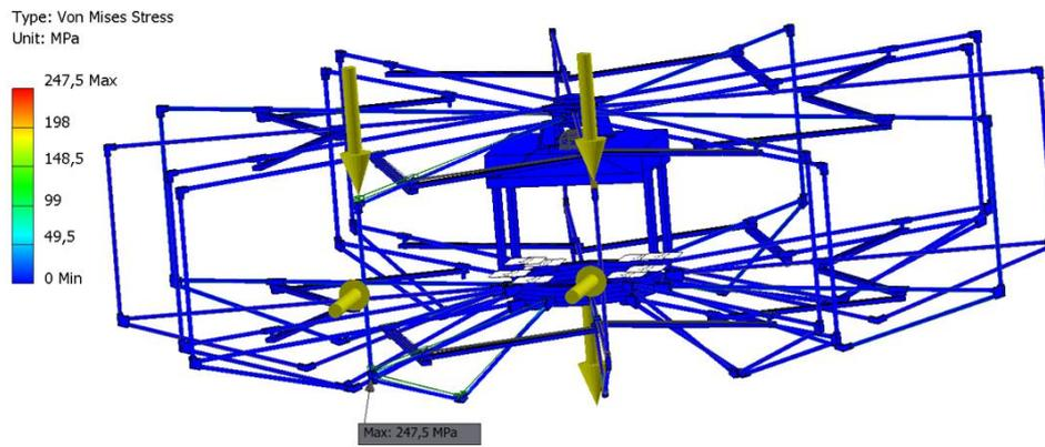
Figure A.7 Simulation results of Von Mises Stress with load applied on the sides
