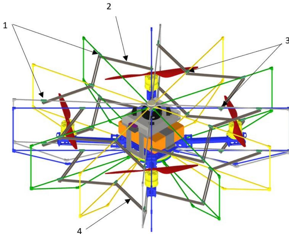
Figure 3.19 Position and connection of plates and connectors on the frame
