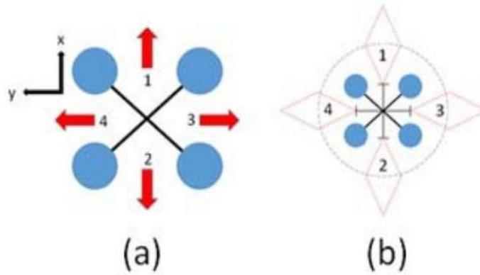
Figure 2.8 (a) Four primary flight directions; (b) Sensor location and obstacle detection directions [12]
