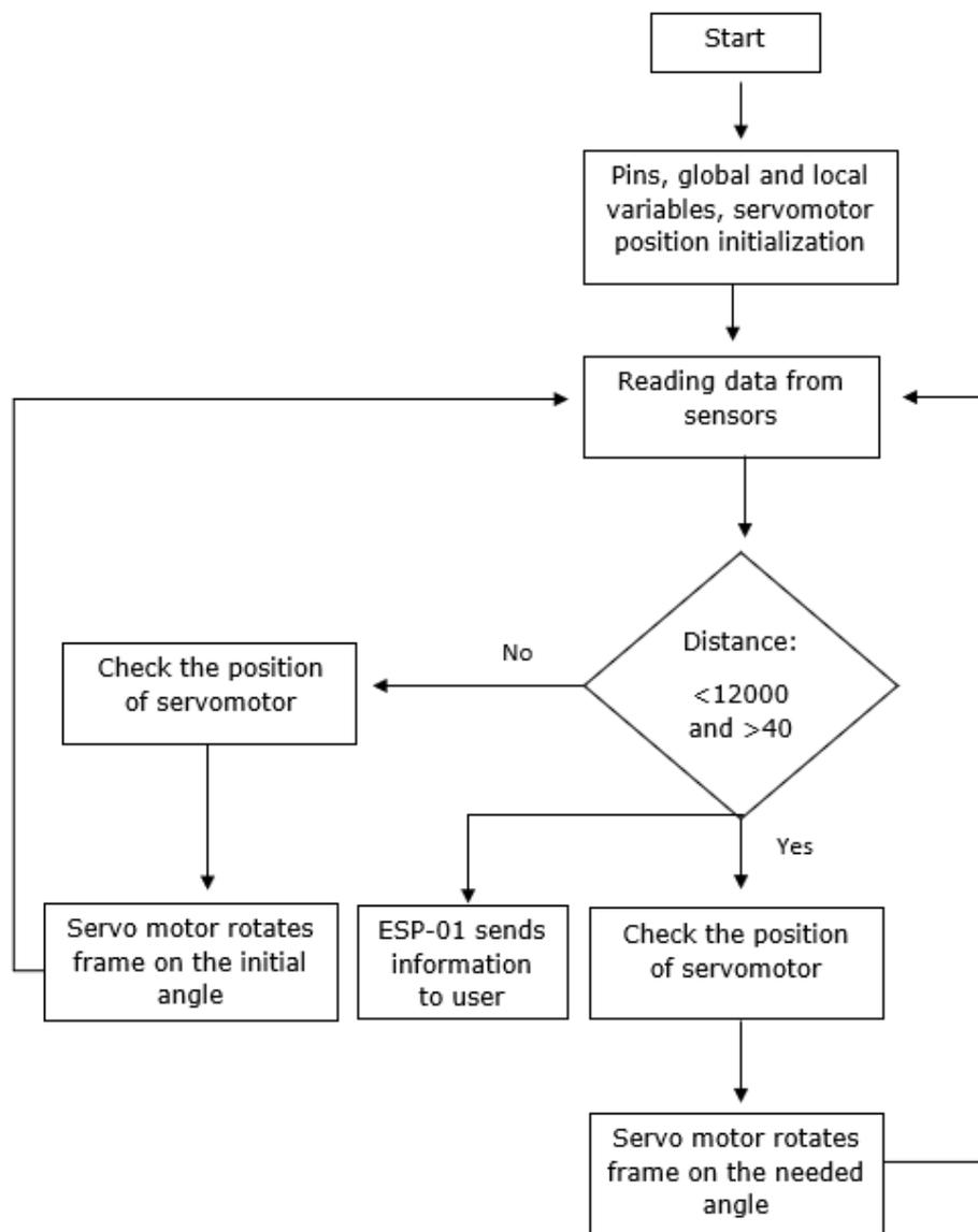
Figure 5.1 Simplified flowchart of the program control
