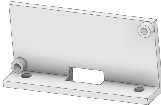
Figure 3.25 TFmini Plus sensor holder
