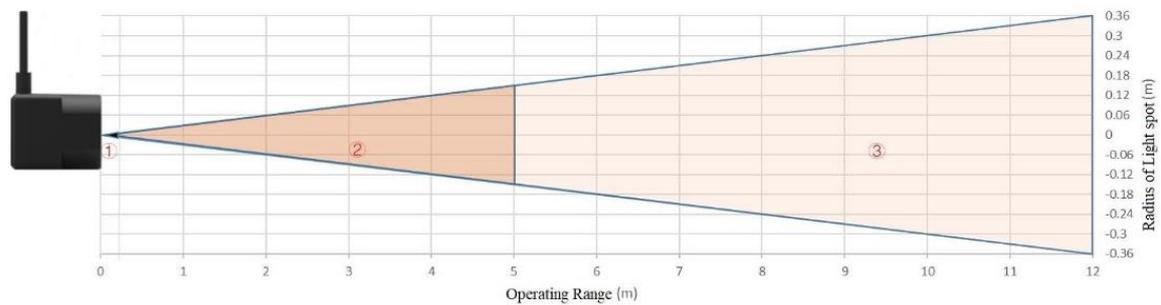
Figure 4.2 Schematic diagram of TFmini Plus distance measurement [23]
