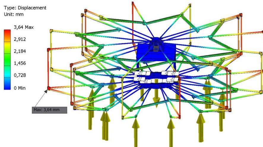
Figure A.9 Simulation results of frame displacement as support of drone
