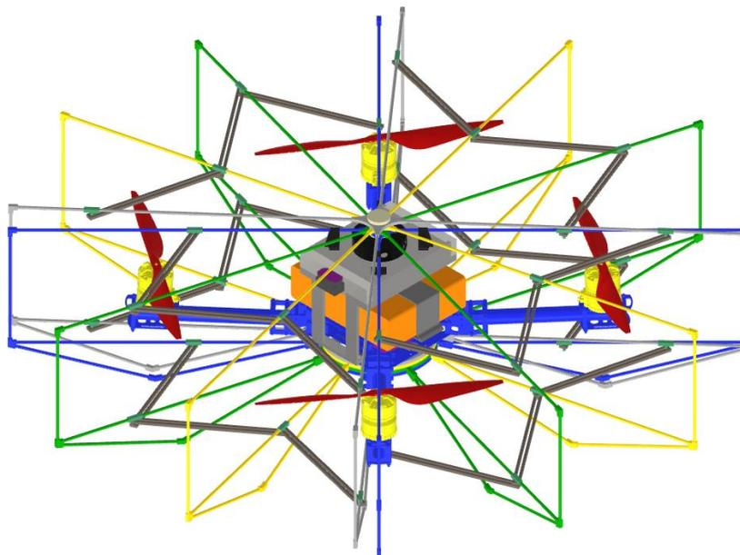
Figure 6.3 Final position of the opened drone cage
