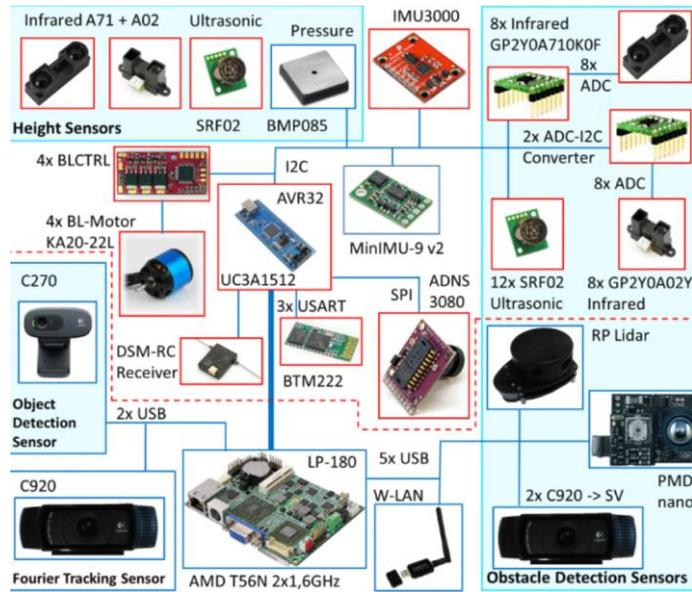
Figure 2.6 Hardware architecture of AQopterI8 [1]
