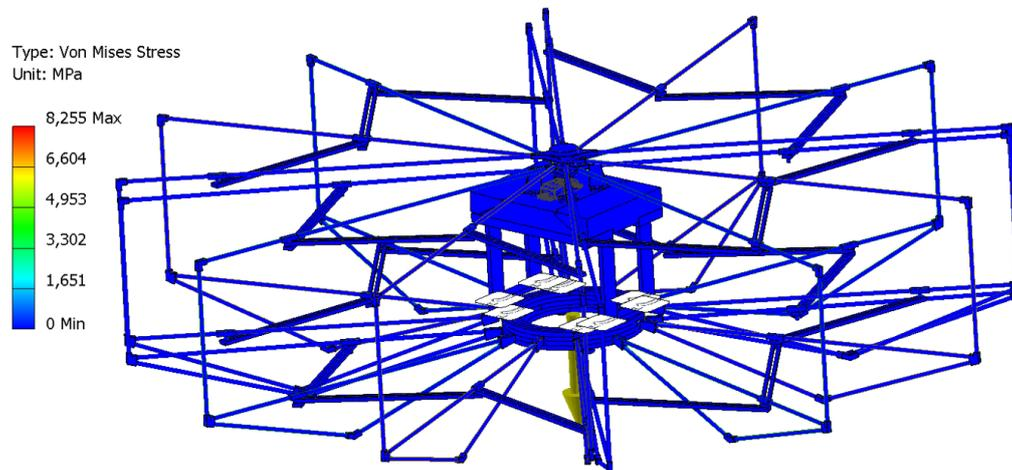
Figure A.2 Simulation results of Von Mises Stress in opened stage without additional load
