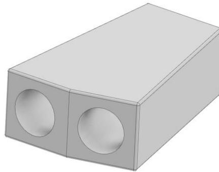
Figure 3.10 Corner for connection bottom and inclined tubes (Type 4)
