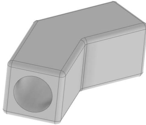
Figure 3.9 Corner for inclined tubes (Type 3)
