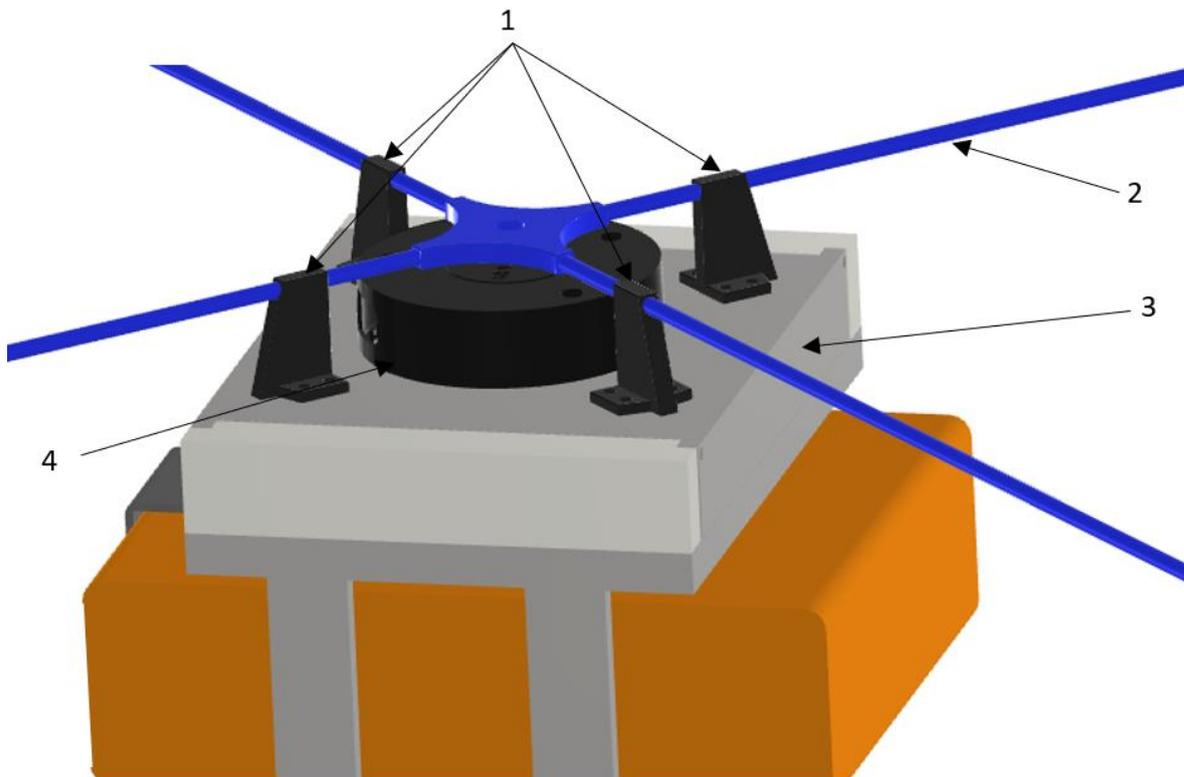
Figure 3.13 Position of fixed frame on the cage holder
