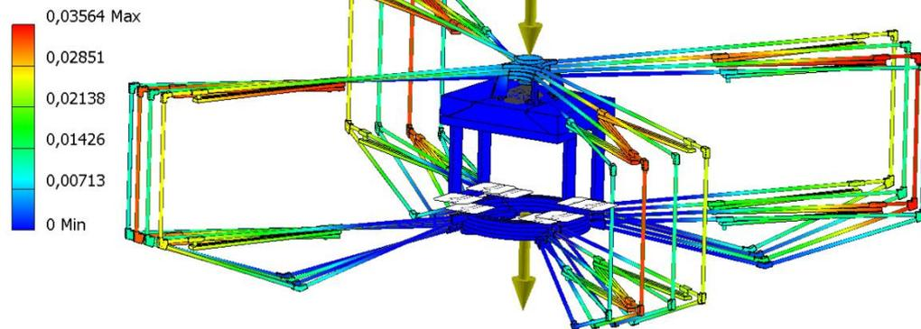
Figure A.6 Simulation results of displacement with load applied on top holder
