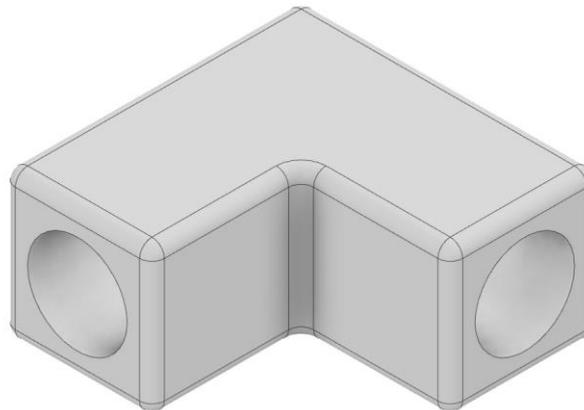
Figure 3.7 Corner for connection upper horizontal and vertical tubes (Type 1)
