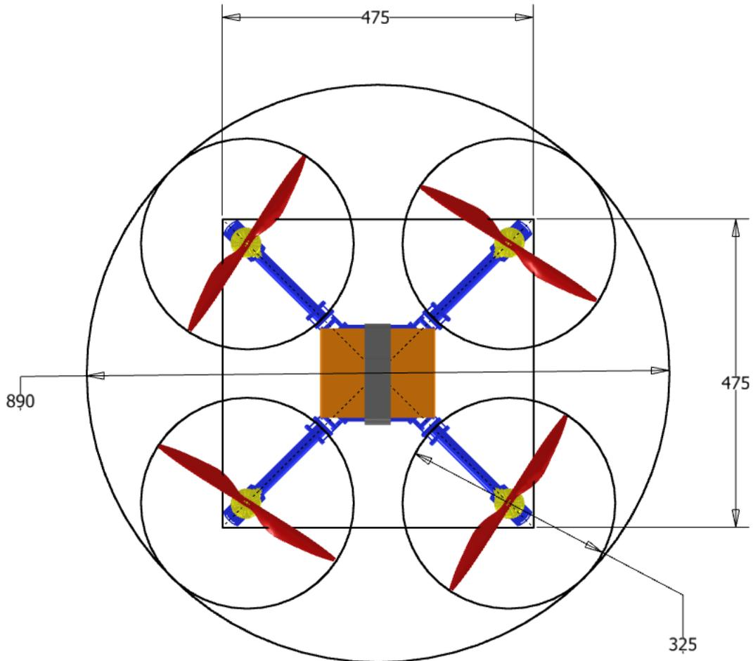
Figure 3.2 Top view of Taltech drone with dimensions in mm
