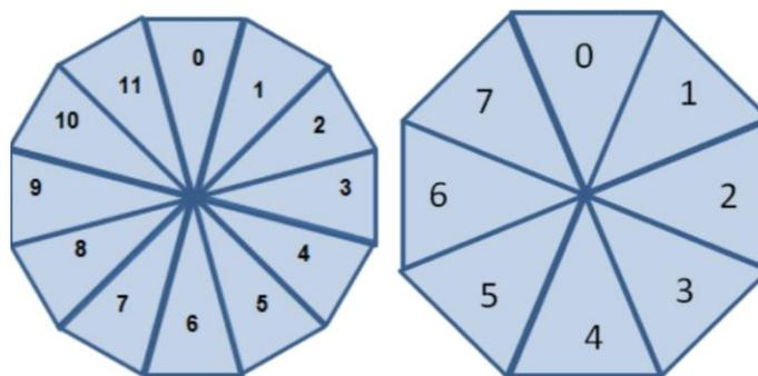
Figure 2.7 Left: the 12 ultrasonic sensors position around the drone. Right: 2x8 sensors position around the drone [1]
