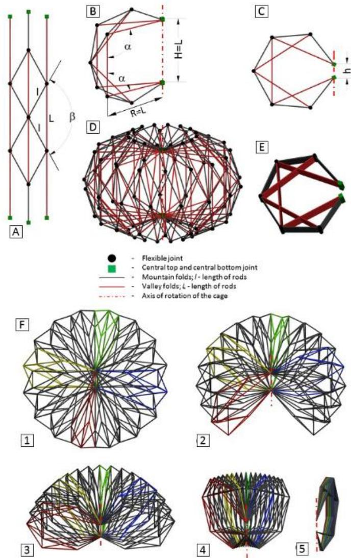
Figure 2.11 A) Top view of the flat pattern of one segment. B) Segment in deployed stage. C) Shape of the folded segment. D) Cage in the fully deployed state. E) Fully folded cage in an isometric view. F) Folding process [16]
