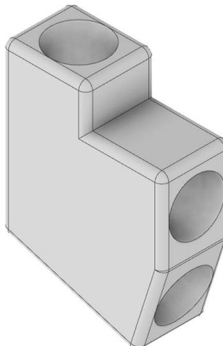
Figure 3.8 Corner for connection of three tubes (Type 2)
