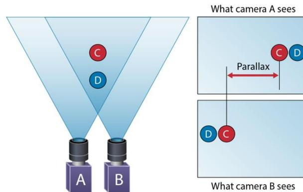
Figure 2.3 Stereo vision sensor setup. View of objects according to the camera position (A, B). D, C points [5]
