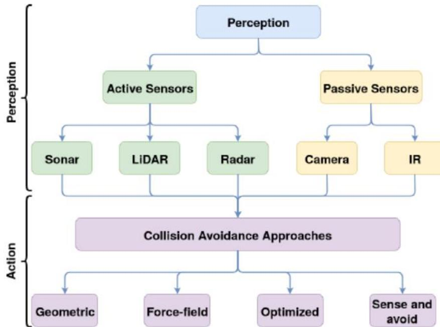
Figure 2.1 Collision Avoidance System Generalised Modules [2]
