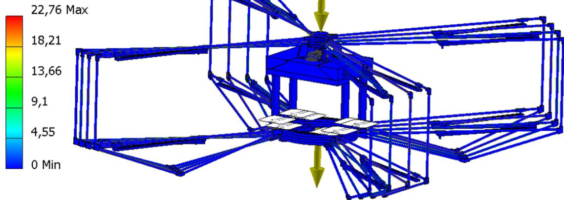
Figure A.5 Simulation results of Von Mises Stress with load applied on top holder
