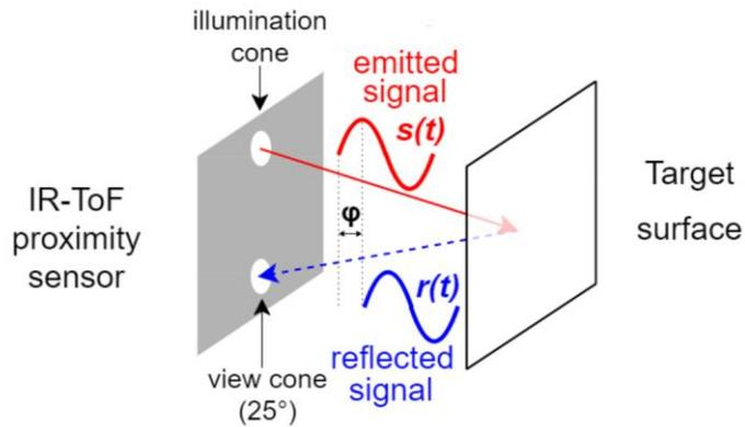
Figure 2.5 The Infrared Time-of-Flight proximity sensor (IR-ToF) provides the distance estimate from the target reflecting surface by measuring the phase shift  $\phi$  between the emitted  $s(t)$  and the reflected  $r(t)$  signals [9]
