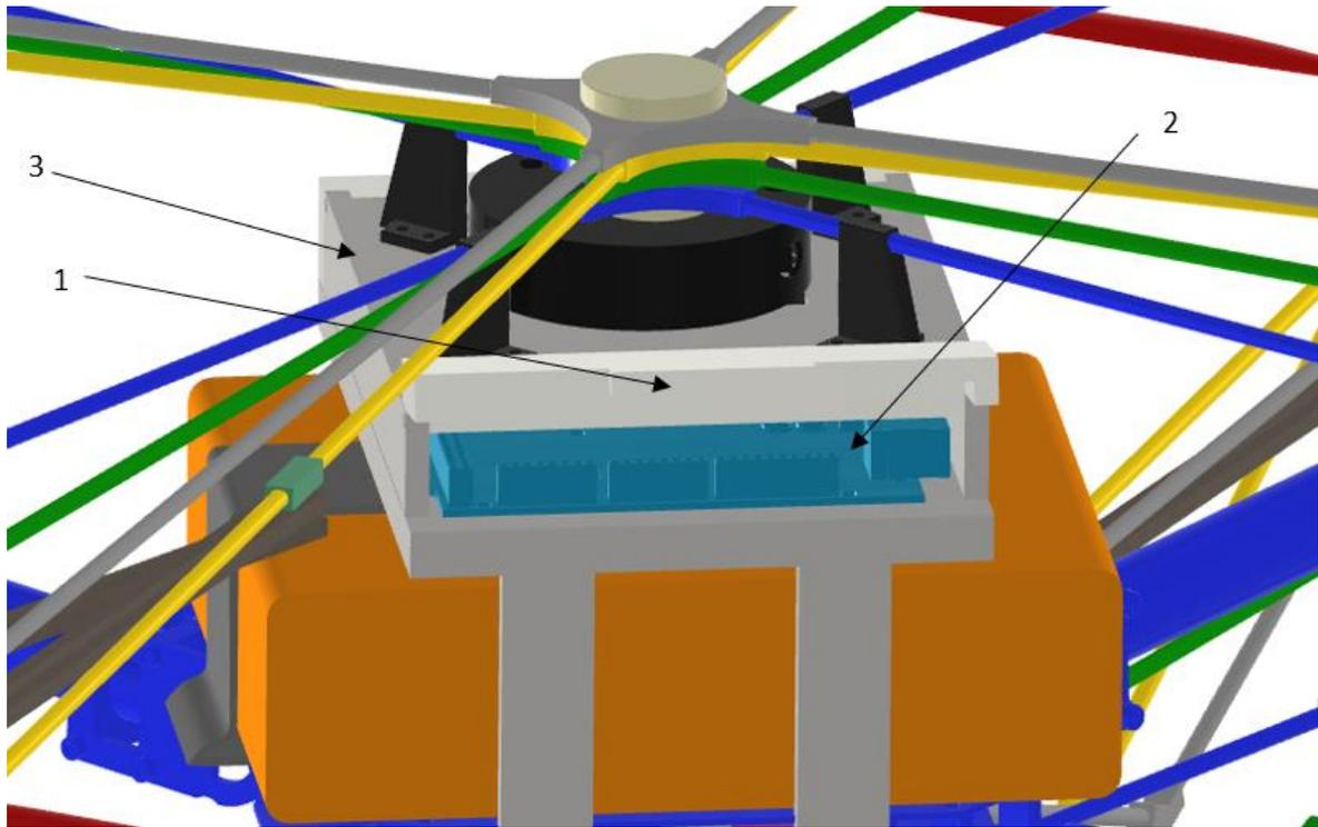
Figure 3.22 View of opened cover, Arduino Mega2560 position inside the box
