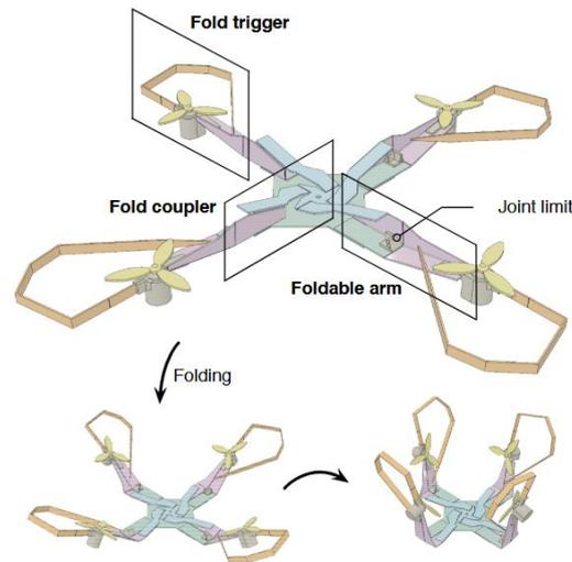
Figure 2.10 An illustration of the three major components (foldable arm, fold coupler, and fold trigger), joint limits, and the folding sequence [15]
