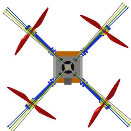
Figure 3.17 Cage in closed stage. All 4 frames are placed over the drone motors
