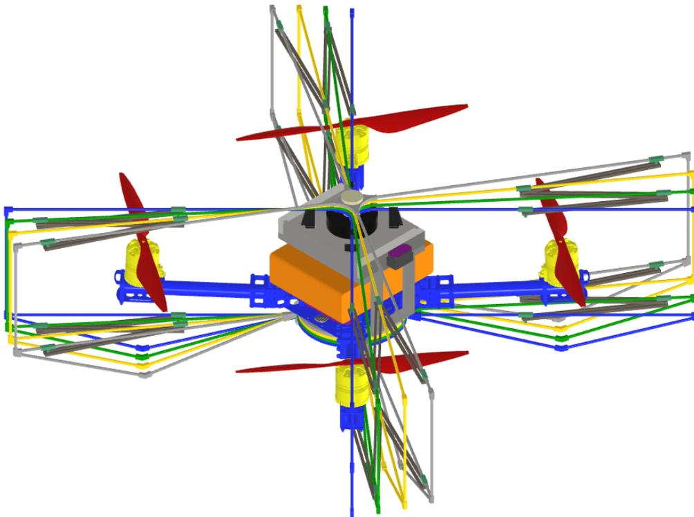
Figure 6.1 Initial position of drone cage before rotation in simulation mode
