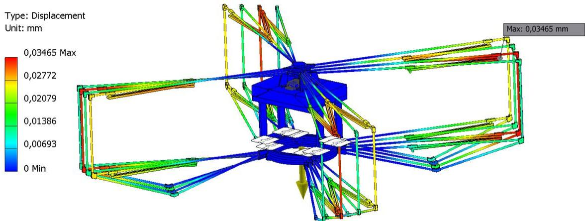
Figure A.4 Simulation results of displacement in closed stage without additional load
