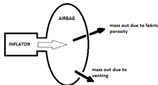
Figure 2.9 Schematic illustration of the gas leakage from the airbag through the fabric porosity and venting [14]
