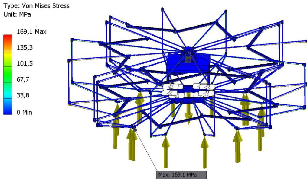
Figure A.10 Simulation results of Von Mises Stress frame as support for drone
