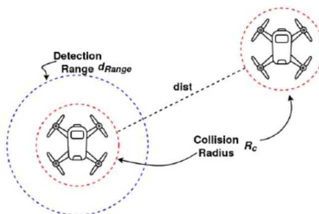
Figure 2.2 Detection Range ( $d_{Range}$ ), Collision Radius ( $R_c$ ) and distance between them [2]
