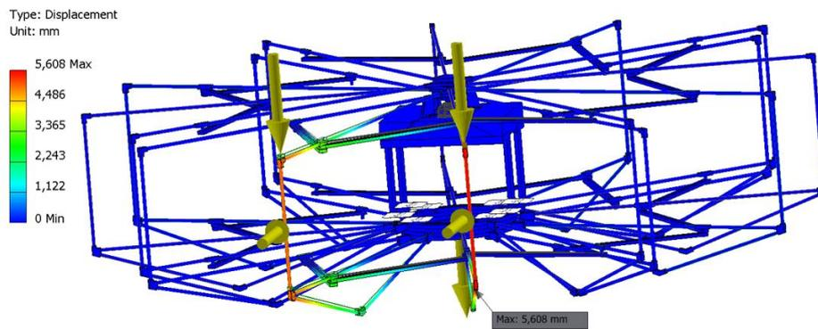
Figure A.8 Simulation results of displacement with load applied on the sides
