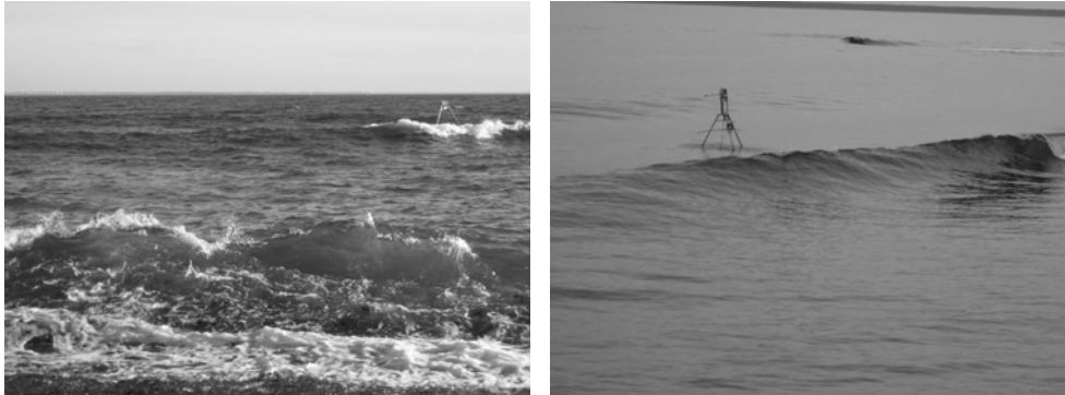
Fig. 5.2. Plunging waves from the Nordic Jet wake approaching the coast on 27 June, 20:00 (left) and spilling waves from the wake from Star approaching the coast on 14 July, 11:24 (right).
