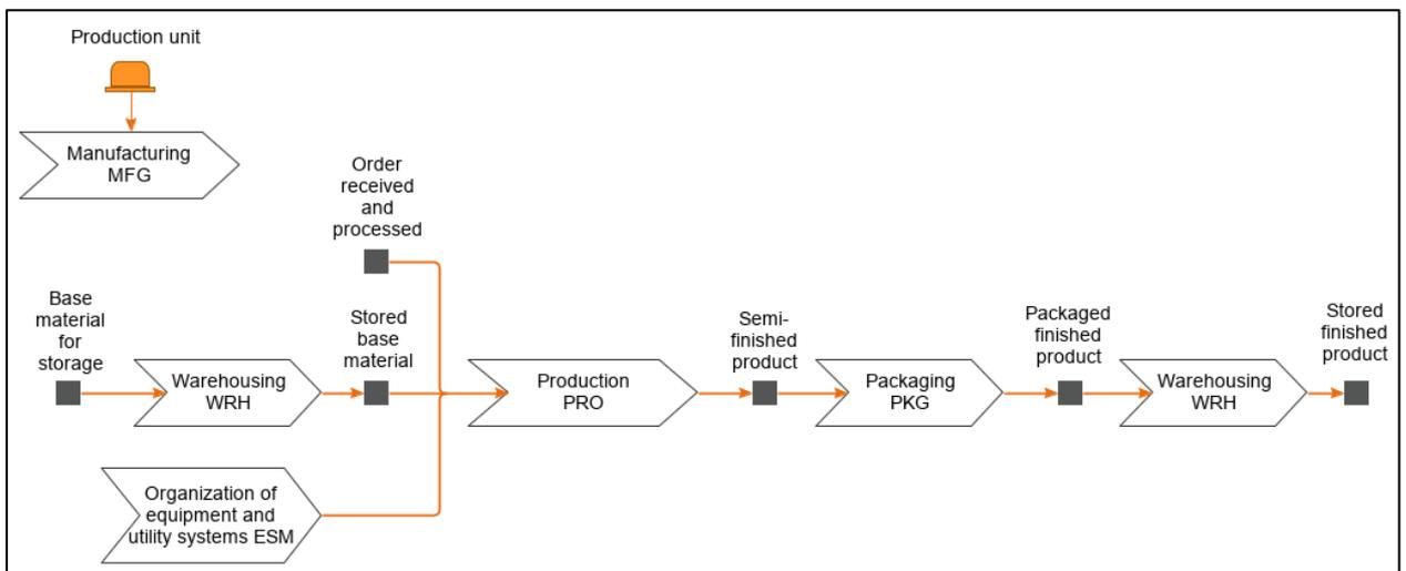
Figure 4. Manufacturing process of Vipis OÜ.
