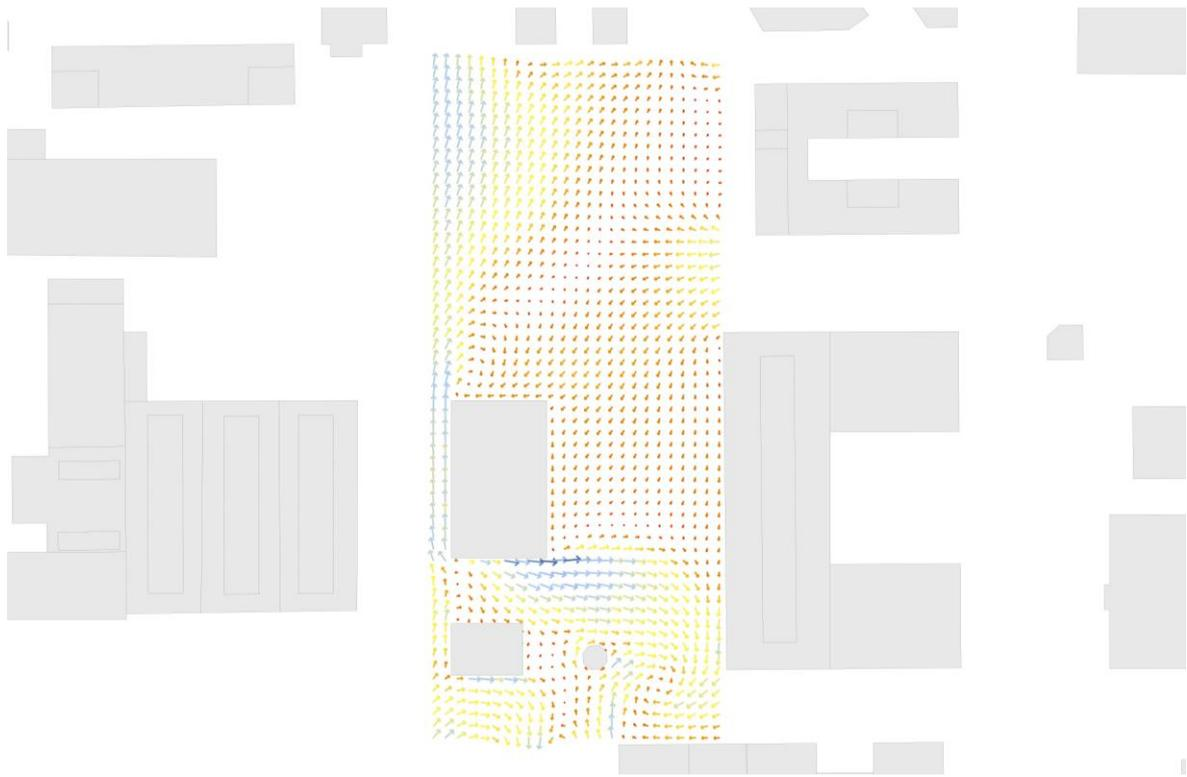
*Figure 15. Wind flow and velocity plot in Lõdtsa park 180°*
