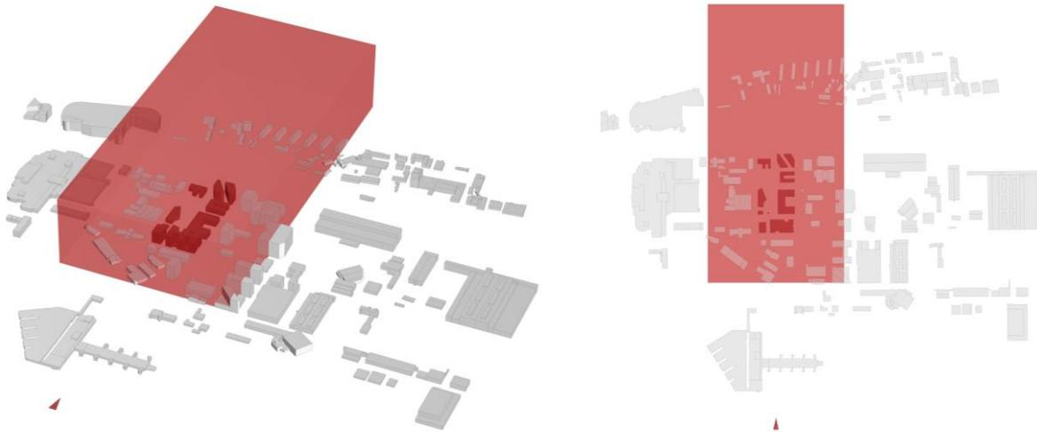
Figure 13. Rectangular wind tunnel for Lõõtsa park, red building are considered into simulation
