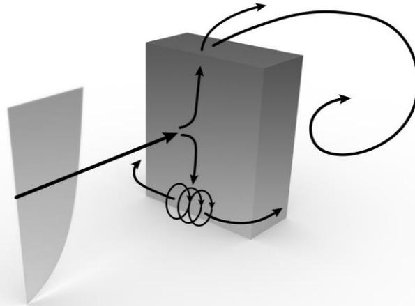
*Figure 2. A schematic representation of wind flow around a single wide high-rise rectangular building*
