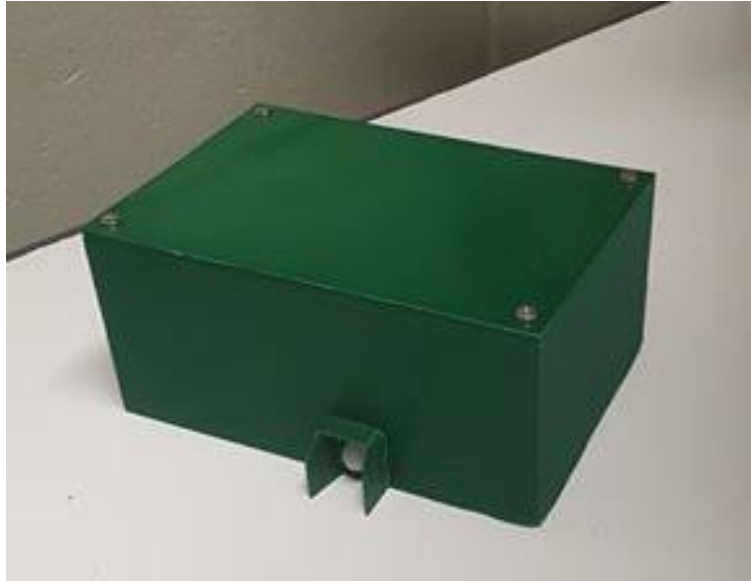
Figure 8. 3D printed casing for the IoT device.
