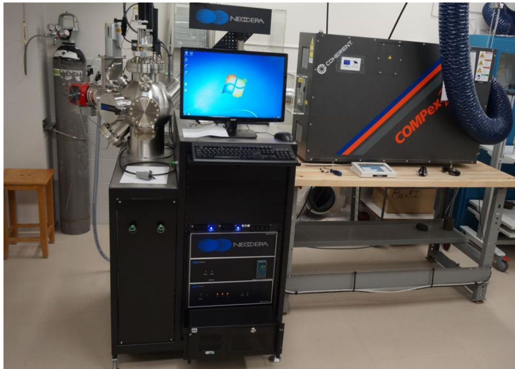
Figure 2.1: photograph image of Neocera Pioneer-120 PLD system.
