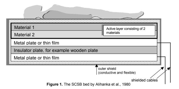
The signals recorded with SCSB are best explained in 2 earliest articles(Alihanka and Vahtoranta, 1979; Alihanka et al., 1981). The SCSB system has 2 drawbacks, first, because of the high measurement sensitivity the mattress records movements of people moving nearby (Alihanka and Vahtoranta, 1979) and secondly, the SCSB is not able to differentiate between different movement localisations(Rauhala et al., 1996).
