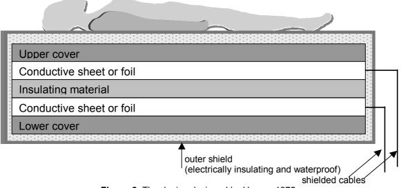
Figure 2. The device designed by Hanna, 1975.
