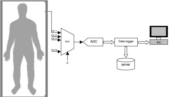
Figure 2. A typical use of FSR sensors in matrix layout
