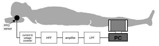
Figure 4. The principle of PPG method based pillow designed by Cha and colleagues.
