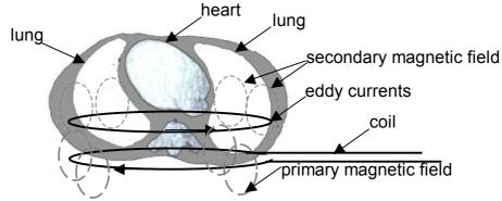
Figure 1. The generation of eddy currents inside the thorax
