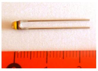
**Figure 1**. A photo of a typical NTC thermistor.
