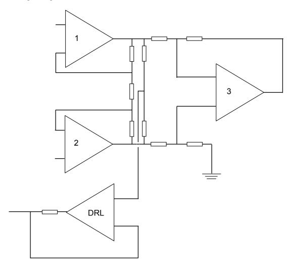
Figure 12. The instrumentation amplifier with Driven Right Leg circuit
