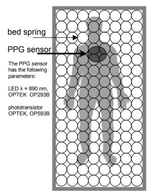
**Figure 3.** A setup there the PPG sensor is placed between the spring coils of the mattress.
