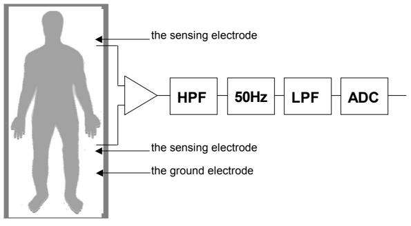
Figure 2. The typical capacitance measurement setup.
