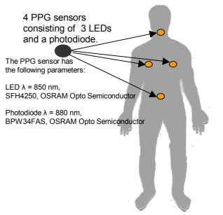
Figure 2. 4 PPG sensor layout
