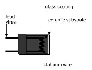
Figure 1. The structure of the RTD sensor.
