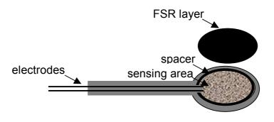
Figure 1. The structure of the typical FSR sensor.
