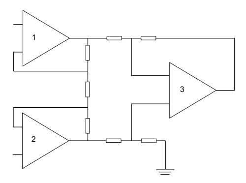
Figure 11. A typical 3 amplifier based instrumentation amplifier.
