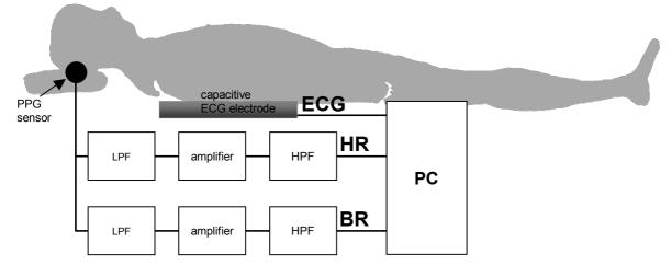
Figure 5. The principle of PPG method based pillow designed by Lee and colleagues
