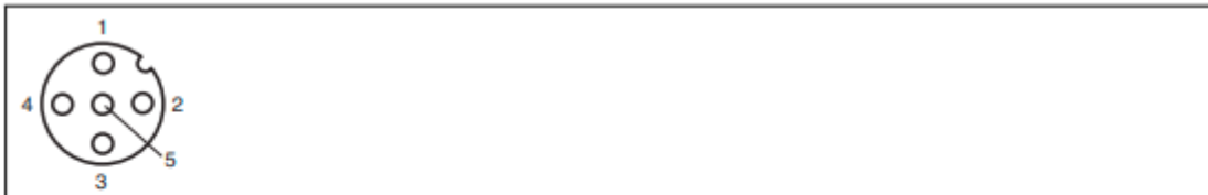
Pin assignment of the M12 socket for RS 232
