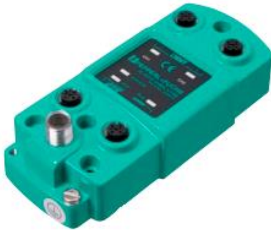
Figure 3-7 Control Interface IC-KP2-2HRX-2V1.[30]
