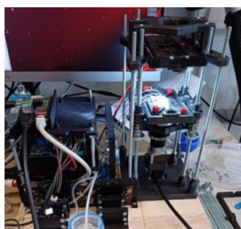
Figure 1: Integrated droplet imaging module of the CogniFlow platform. The mechanical frame and enclosure (not shown here) are shared between all platform modules, optics and electronics stages are changed according to the purpose.
