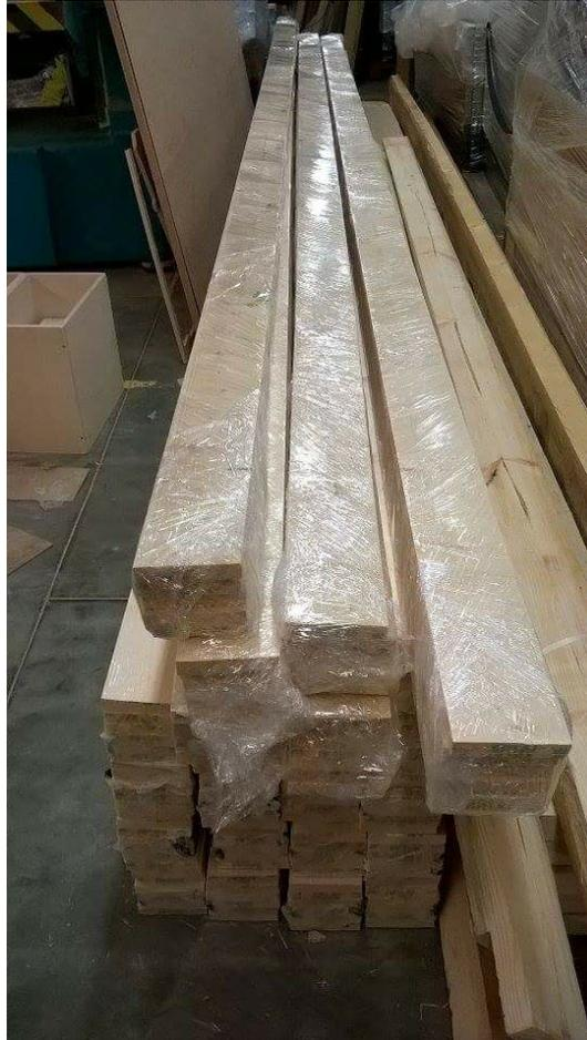
Figure 7 Boards with cross-section of 18x100mm
