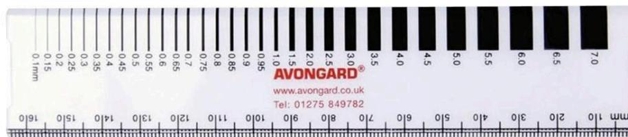
Figure 18 Crack Width Gauge for measuring cracks in CLT panels [13]
