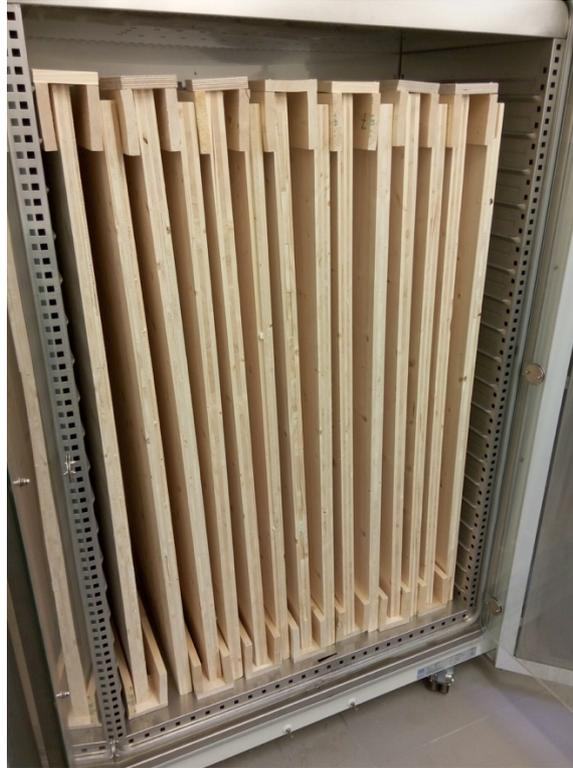
Figure 14 Panels with dimensions of 1300x460x40mm inside climate chamber Climacell 707
