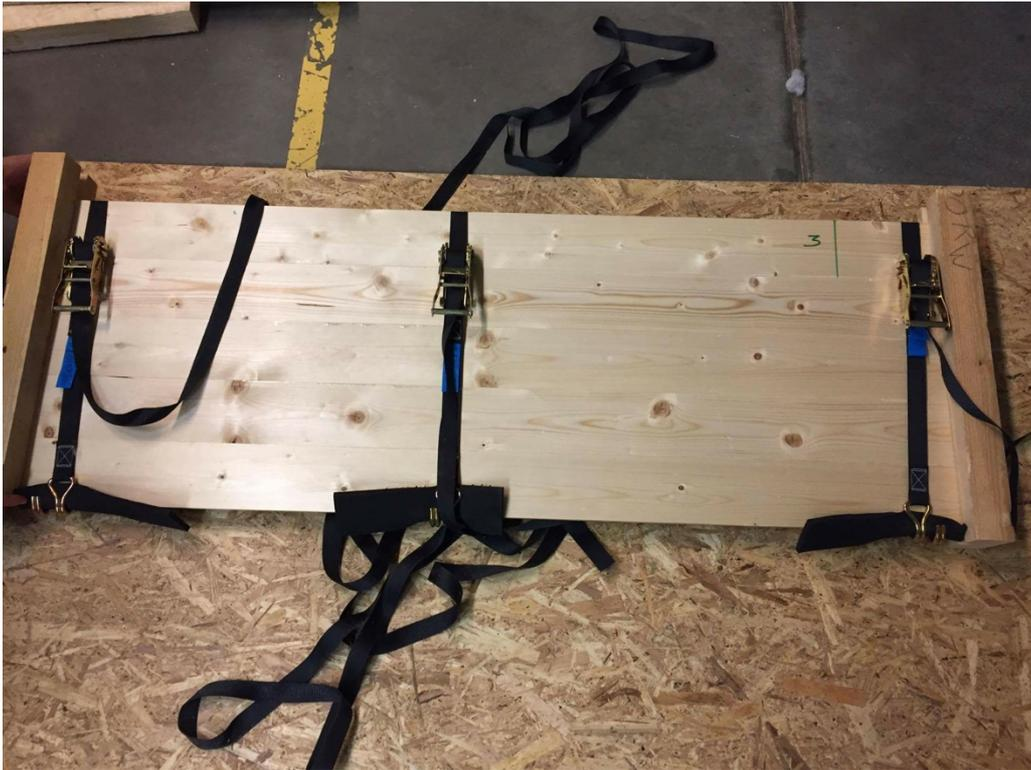
Figure 9 Jig with loading straps to add sufficient pressure
