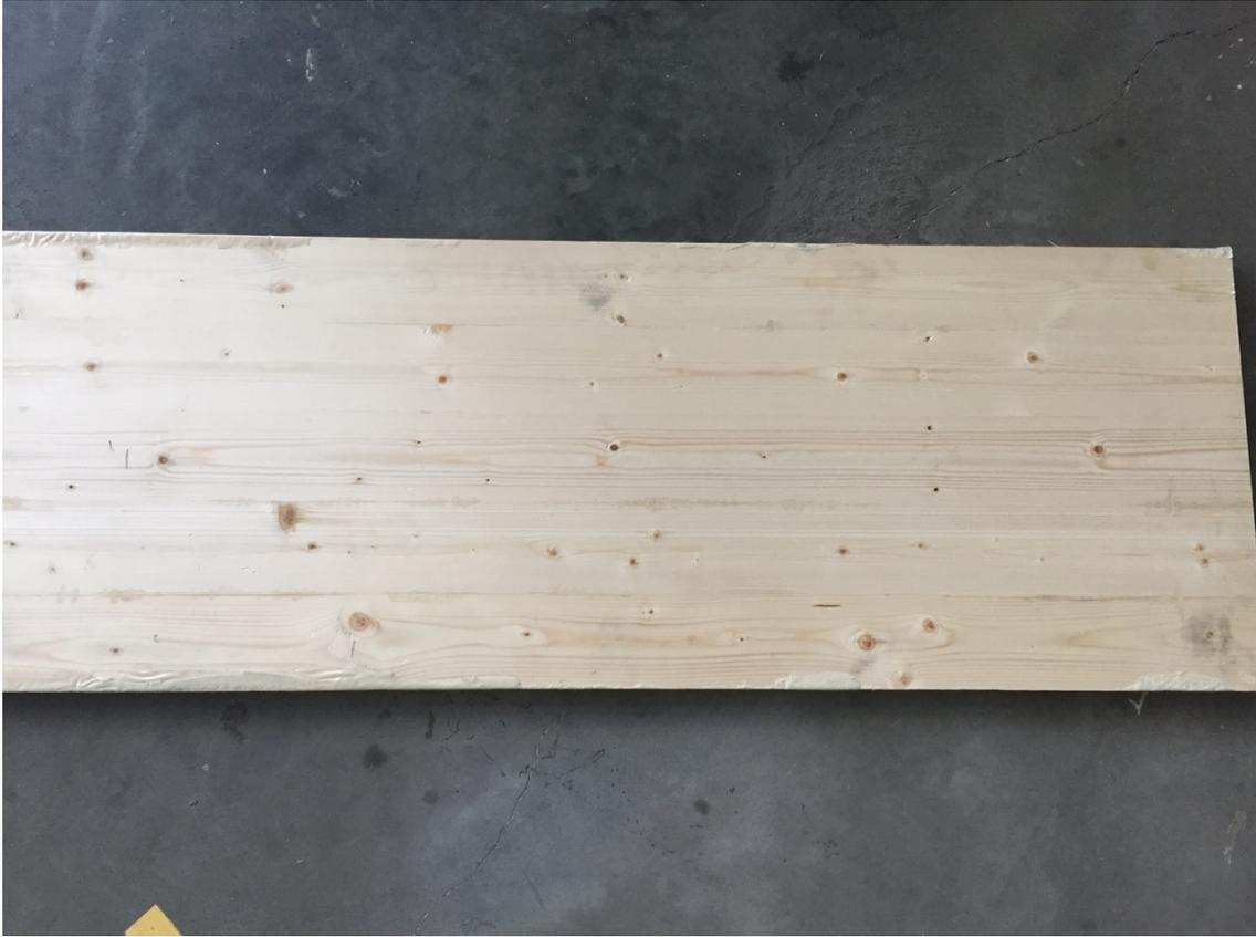
Figure 25 Surface of specimen with bonded edges after conditioning
