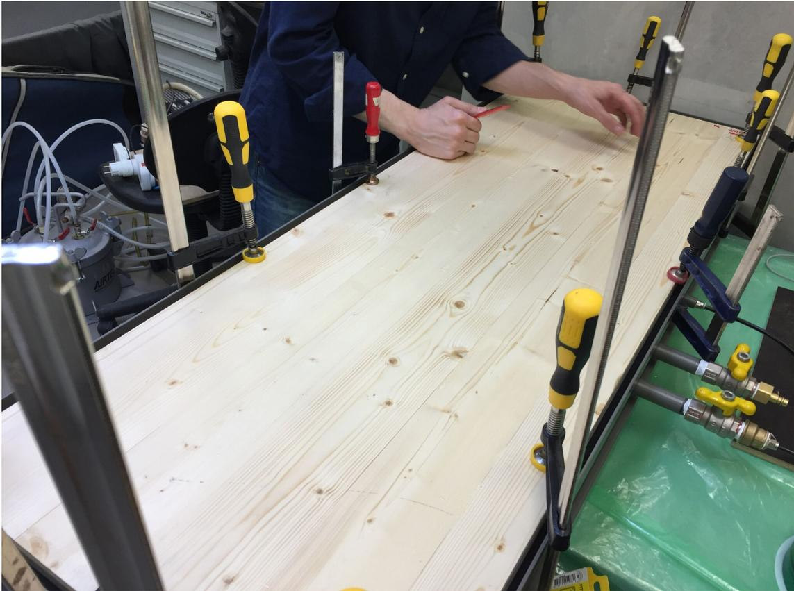
Figure 29 Clamping system for fastening the panel
