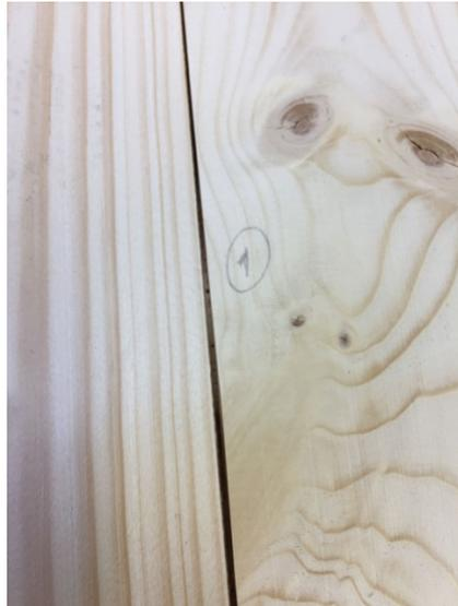
Figure 3 Gap between lamellae's of CLT panel prepared without bonded edges
