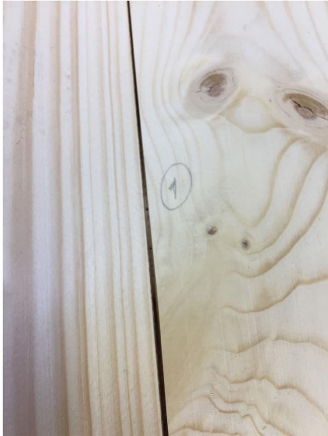
Figure 17 Marked crack between laminations
