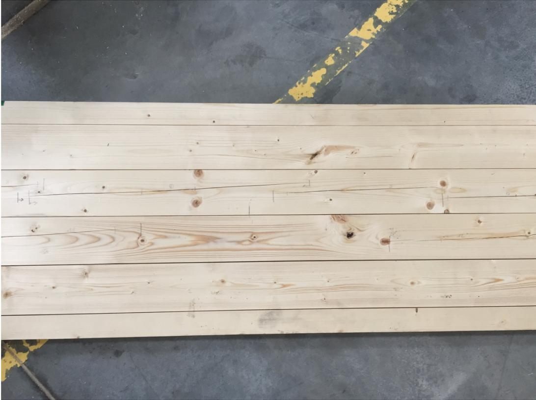
Figure 23 Surface of specimen without bonded edges after conditioning
