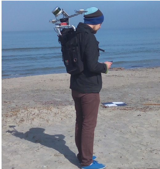
Fig. 5 MLS sensors on a purpose-built frame mounted on car's rear-side (above) and a backpack (below). The car-mounted LIDAR device is in the center, on top of the GNSS/INS unit, dual GNSS antennae are located on the sides. (Paper I)
