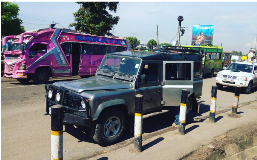
Fig. 9 The MLS system combined with Ladybug 5 panoramic camera of Reach-U during 2016-2017 field surveys in Hanoi, Vietnam (above) and Nairobi, Kenya (below).
