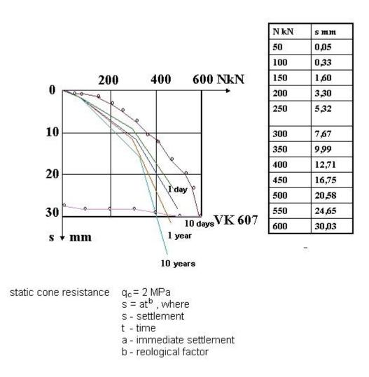
Figure 12. The dependence of the settlement of the wedge shape pile on the load.
