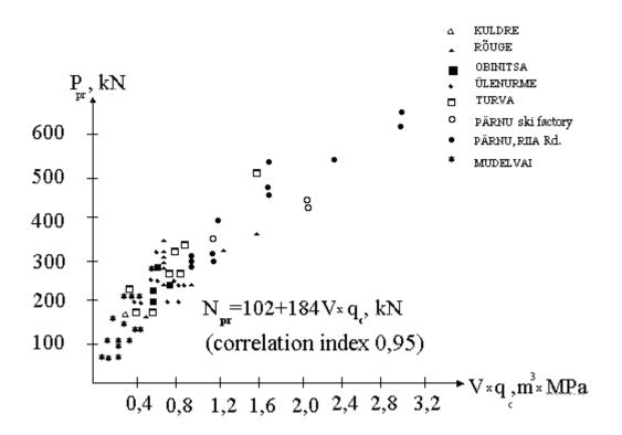
Figure 14. The dependence of wedge shape pile  $P_{pr}$  on the pile's capacity and on the average value of static cone resistance on the extent of the length of the pile (Tammemäe, 2003).
