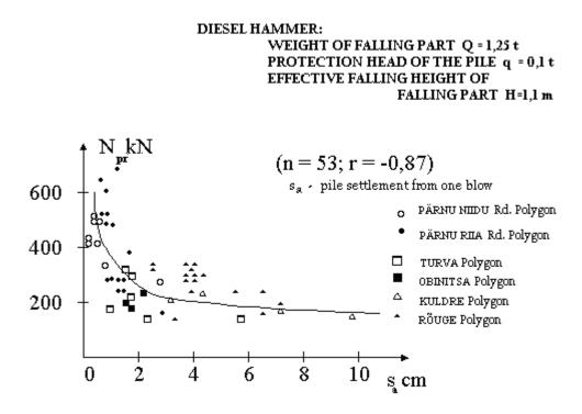
Figure 13. Dependence of wedge shape pile N<sub>pr</sub> on equivalent of pile S<sub>a</sub>
