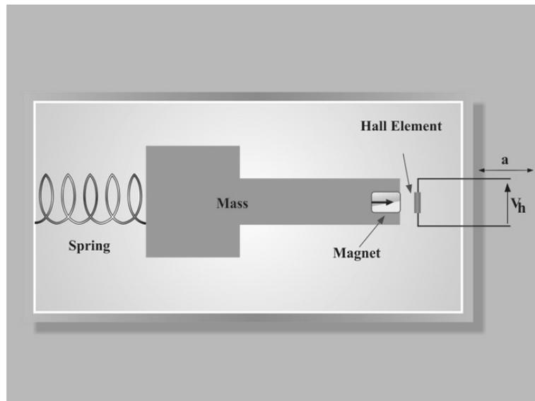
Figure 6. hall effect accelerometer, source: [9]
