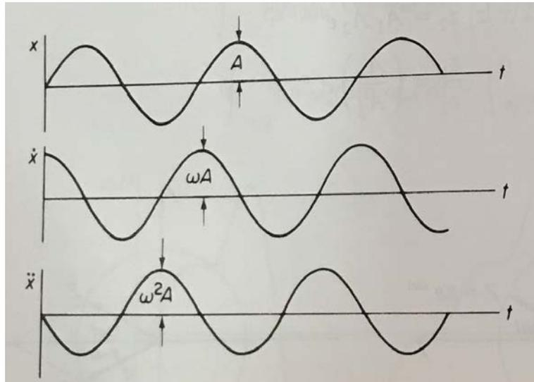
Figure 7. distance, velocity, and acceleration of simple harmonic oscillation, source [1]
