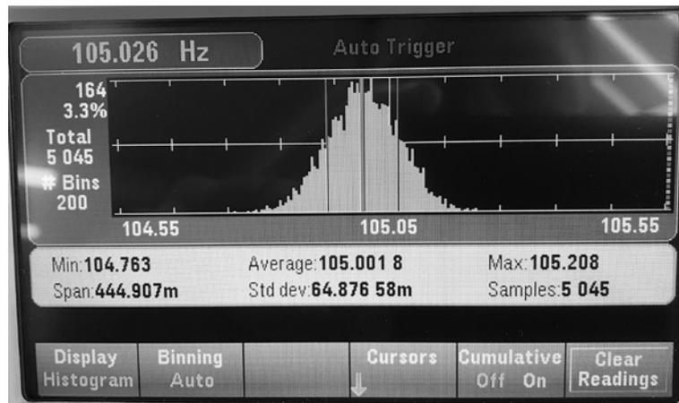
Figure 13. sensor ODR of 105 Hz (1), source: DMM output
