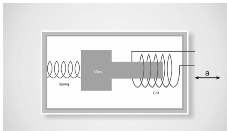
Figure 5. variable inductance accelerometer, source: [9]
