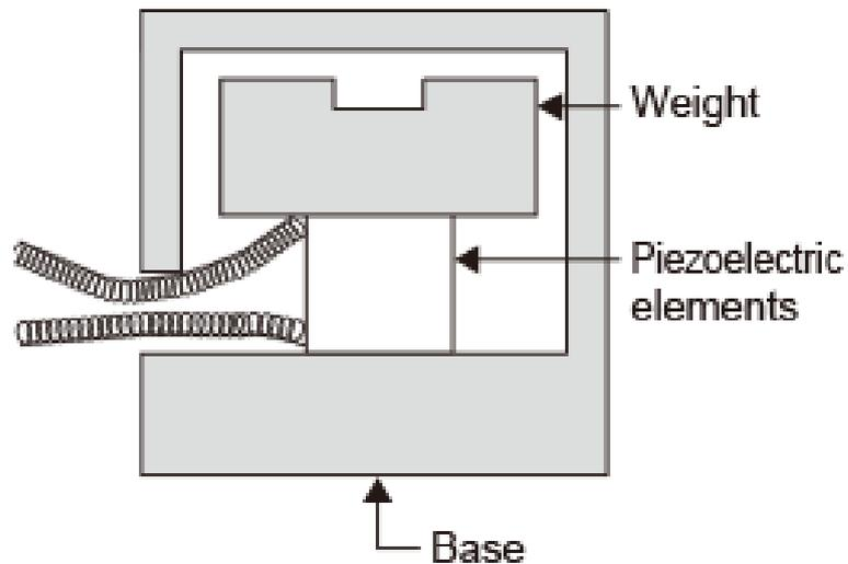
Figure 3. piezoelectric accelerometer, source: [9]
