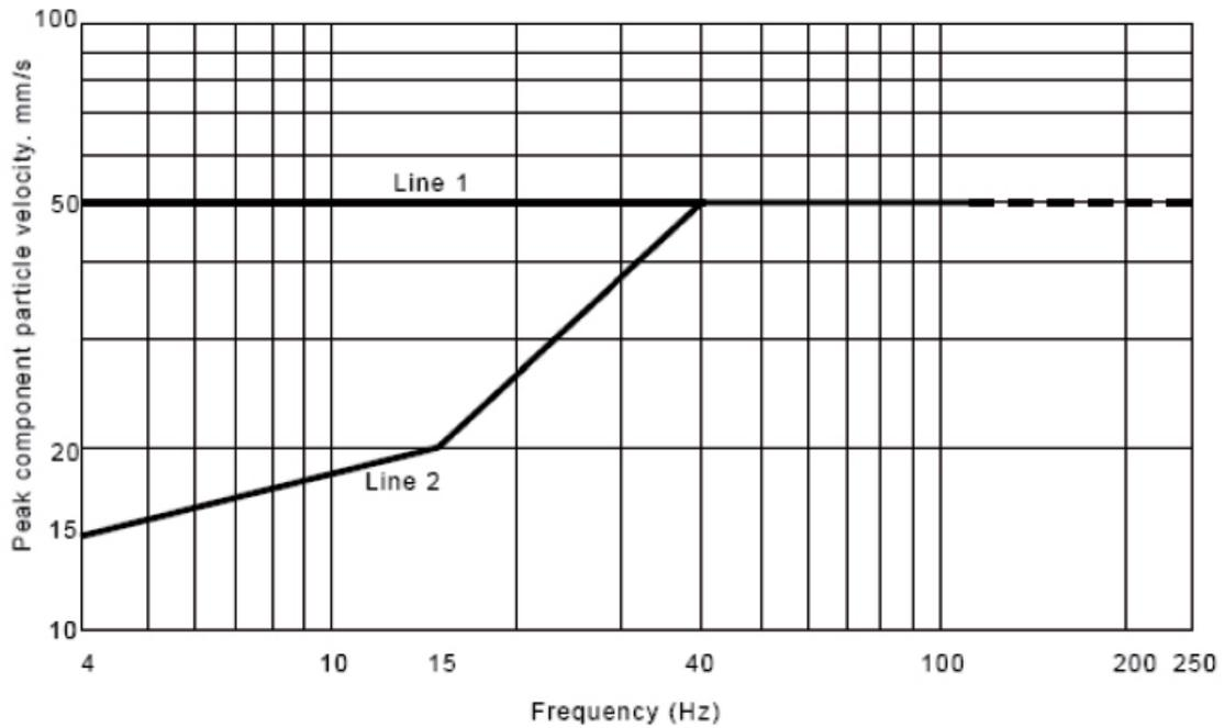
Figure 1. Transient vibration guide values for cosmetic damage, source: BS 7385-2
