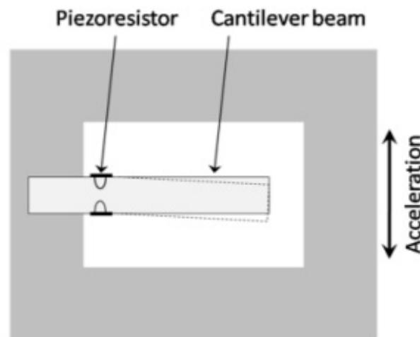
Figure 4. piezo resistive accelerometer, source: [9]
