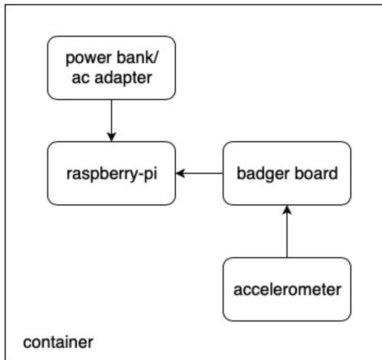
Figure 11. sensor container schematic, source: created via draw.io
