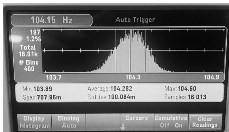
Figure 14. sensor ODR at 105 Hz (2), source: DMM output
