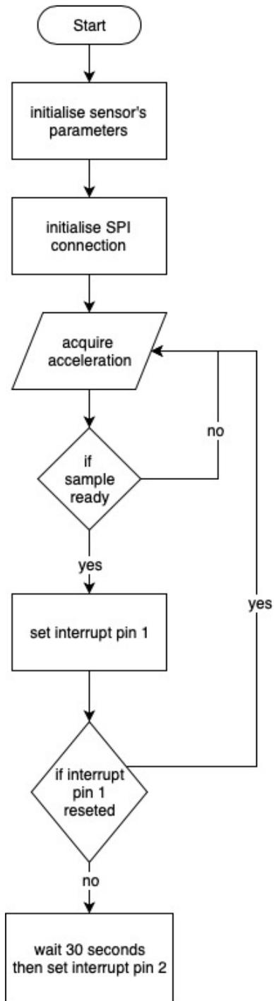
Figure 12. acquisition program flow chart, source: created via draw.io
