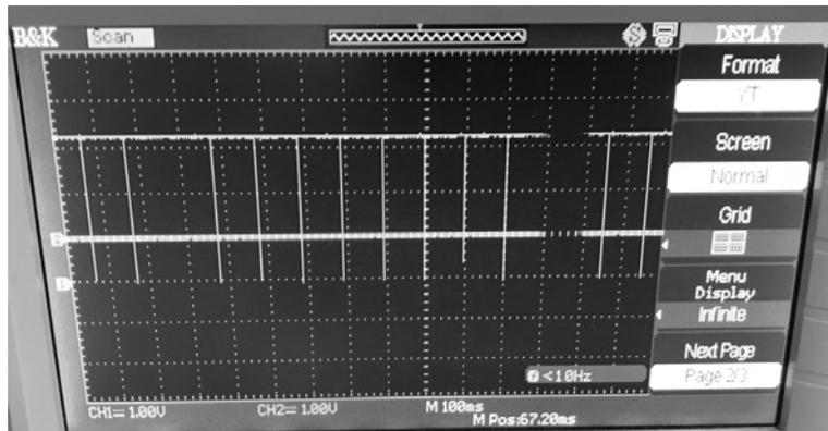
Figure 8. sensor's SPI MOSI signal, source: oscilloscope output
