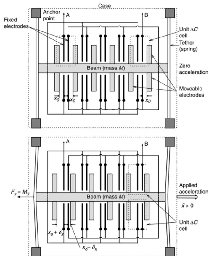
Figure 2. simplified top view of the Analog Devices ADXL50 MEMS sensor a passive, linear accelerometer, source: [8] chapter 7- 7.3.1.14 micromachined IC accelerometer
