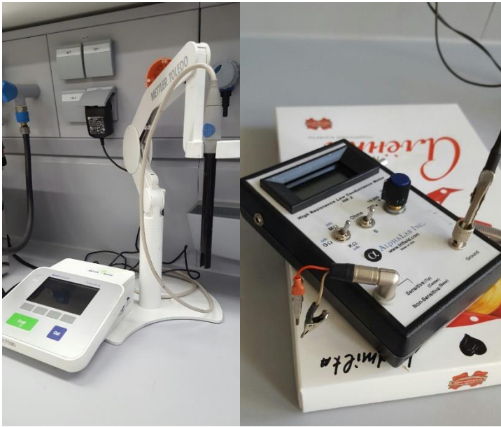
Figure 5 Conductivity meter of solutions (left) and electrospun mats (right)
