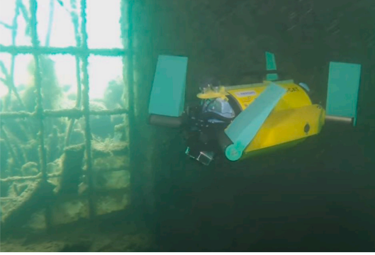
Fig. 1. View of U-CAT robot during an inspection mission in a submerged structure.
