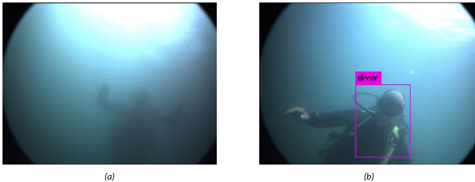
Figure 6: Underwater images from U-CAT's camera in open water conditions (a) Frame example where visual detection is unsuccessful due to poor visibility conditions. (b) Frame example where the diver is successfully detected when close enough. ([Publication 1] ©2020 Wiley Periodicals LLC).
