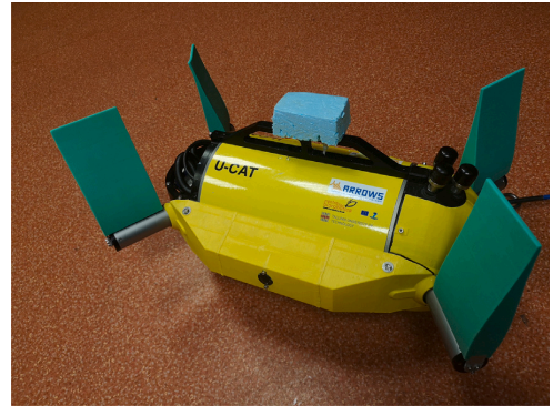
Fig. 14. U-CAT pictured with an added buoyancy foam fixed on its top.
