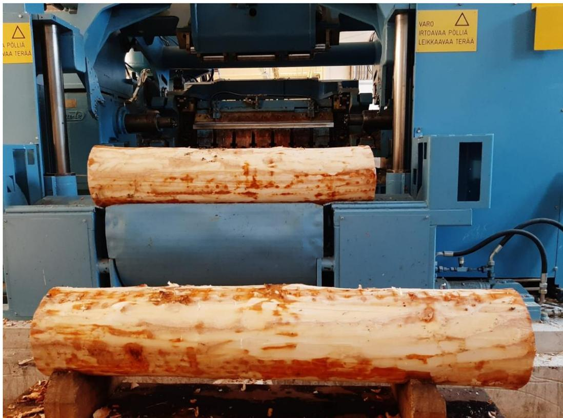
Figure 2.1 Debarked logs fed into the rotary veneer peeling lathe
