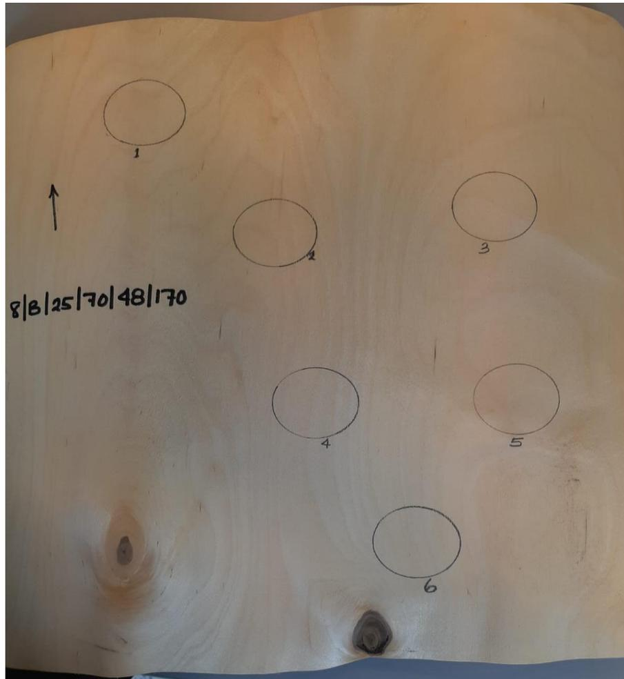
Figure 2.7 Birch veneer sheet with 6 measurement points
