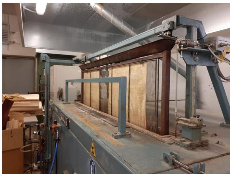
Figure 2.4 Veneer sheets stacked up in the steam veneer dryer for drying
