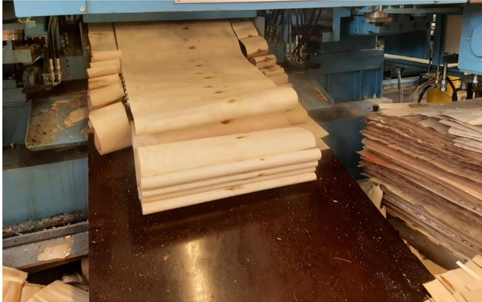
Figure 2.3 Peeled veneer mat from rotary veneer peeling lathe
