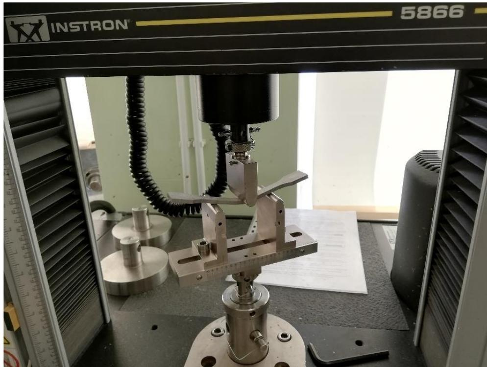
Figure 2.10 Flexural test with Instron 5866
