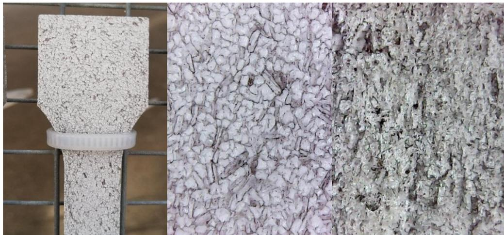
Figure 3.2 Left - WPC surface; centre WPC front side; right - WPC backside after weathering
