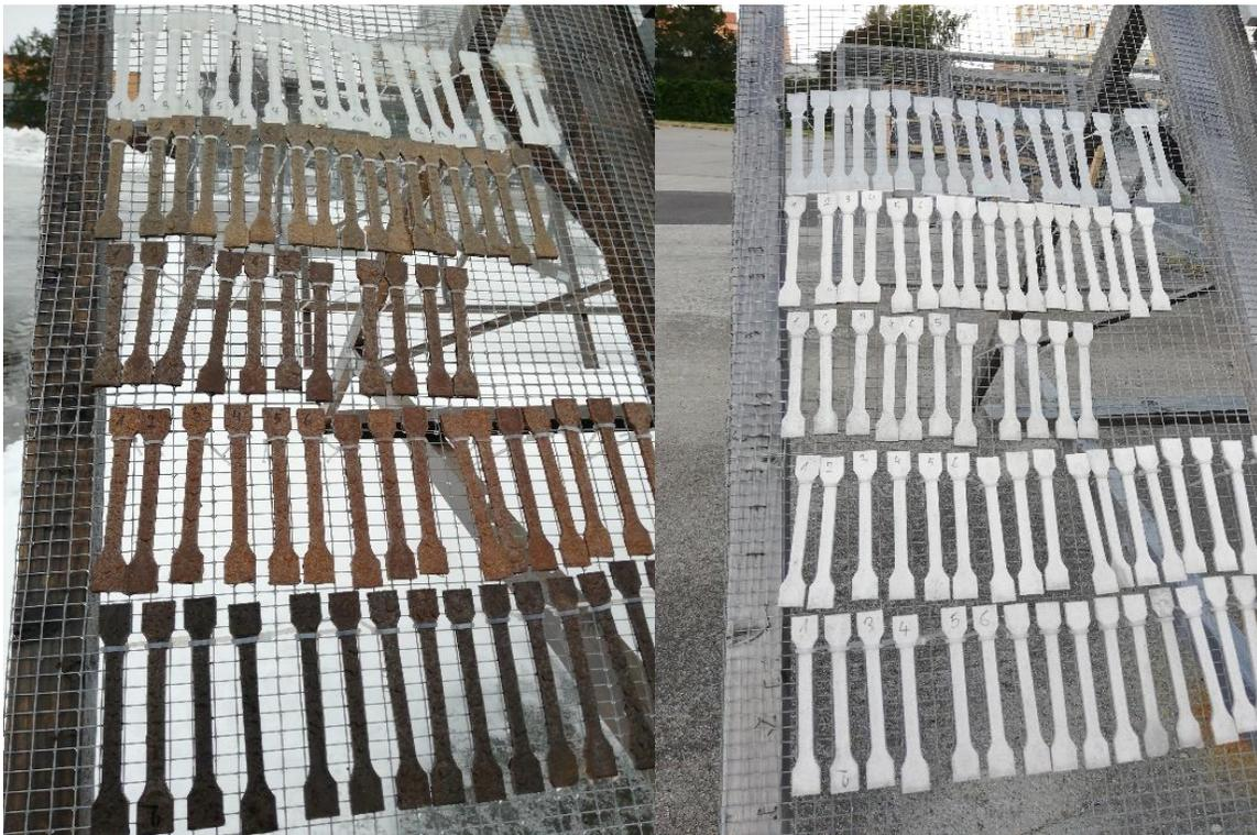
Figure 3.1 Left - test specimens before weathering; right - after weathering
