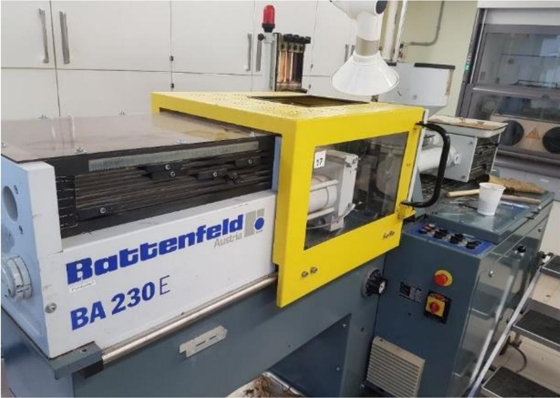
Figure 2.3 Battenfeld BA 230E used for injection moulding
