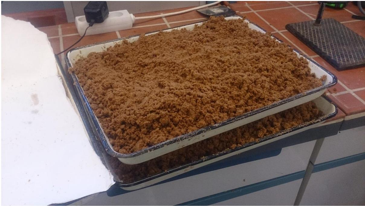
Figure 2.2 Wooden filler during modification with APTES
