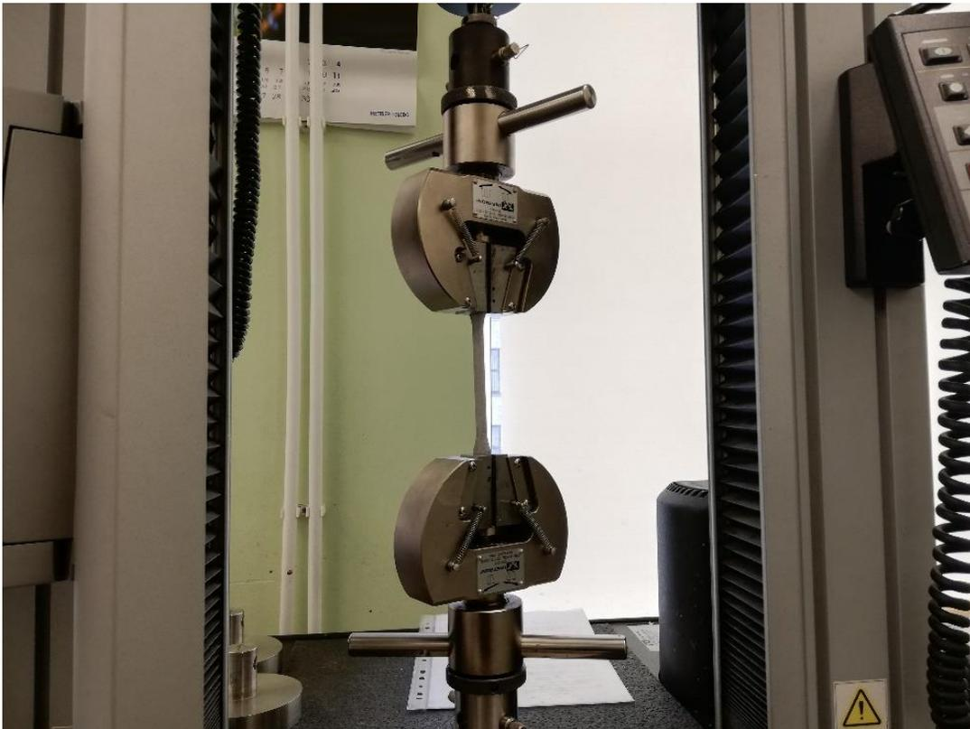
Figure 2.9 Tensile test with Instron 5866
