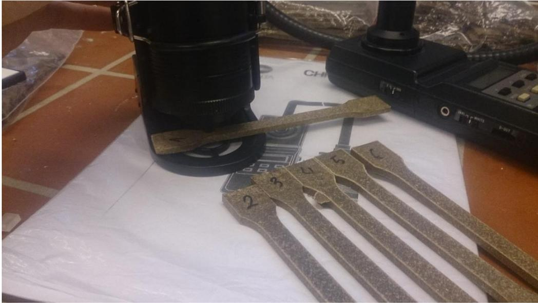
Figure 2.7 Colouration measurement with Minolta CR-121
