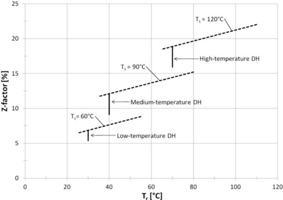
Figure 3.4 Relation between z-factor and the DH operating temperatures in a condensing steam turbine of CHP [14].
