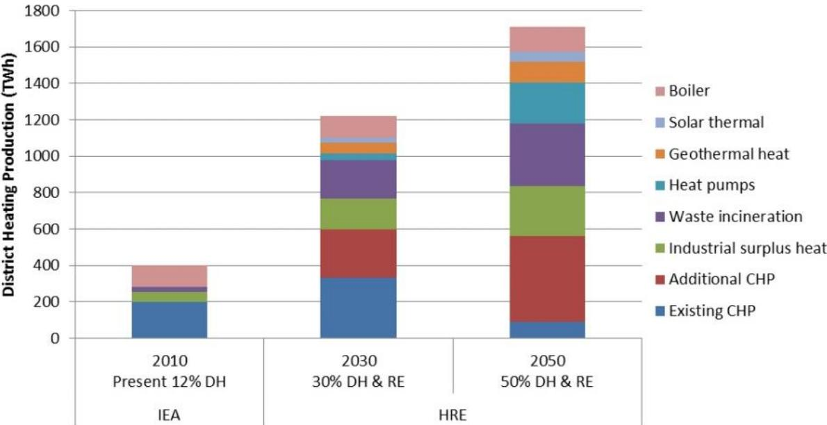
Figure 3.7: DH predictions for the EU27 energy system in 2030 and 2050 along with the production in 2010 [18]
