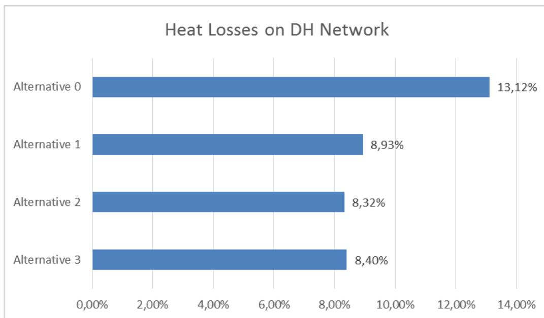
Figure 4.8: Rates of annual heat losses on Jõgeva DH network
