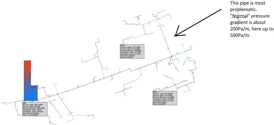
Figure 4.4. Possible excessive pressure failure on the Jõgeva DH network at the conditions of Alternative 1.
