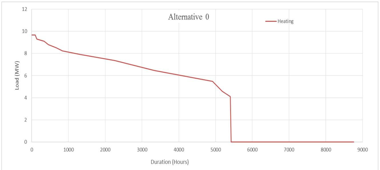
Figure 4.3. Load-duration graph of *Alternative 0*.
