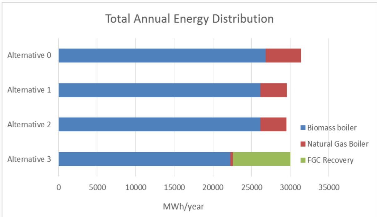
Figure 4.7: Total annual energy distribution from Jõgeva boilerhouse
