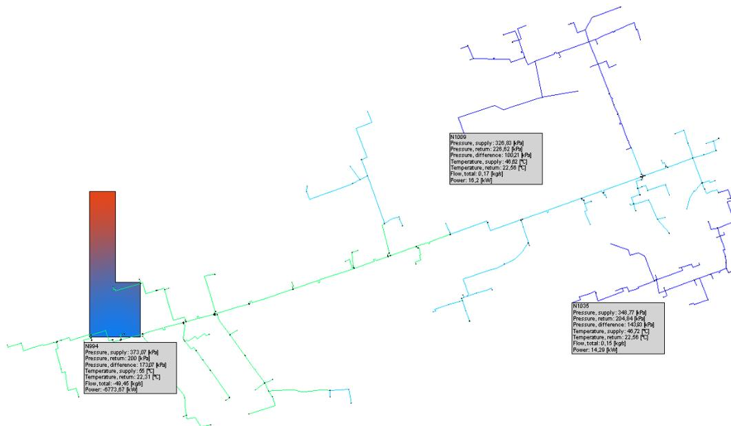
Figure 4.9: Plan of Jõgeva DH network with the simulation Alternative 2 at 0°C outdoor temperature
