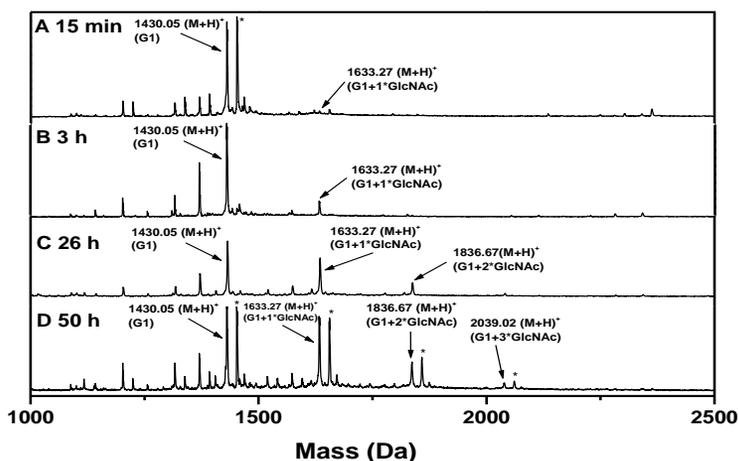
**Figure 15.** MALDI-TOF MS spectra of samples taken at different times during the reaction that show the establishment of the equilibrium between the first generation PAMAM dendrimer and GlcNAc. \* - corresponding sodium ion.
