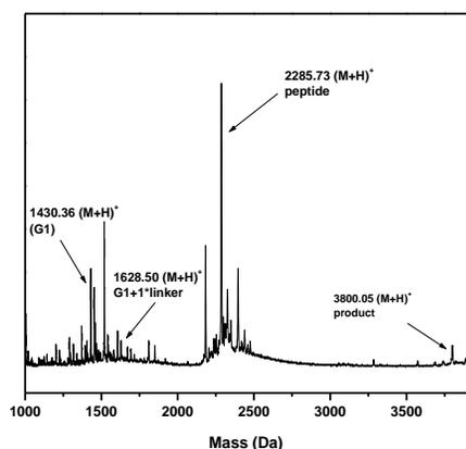
**Figure 27.** MALDI-TOF MS spectrum that shows the ratios of the product (G1 dendrimer+SPDP+Peptide-Cys) and various impurities in the reaction mixture.
