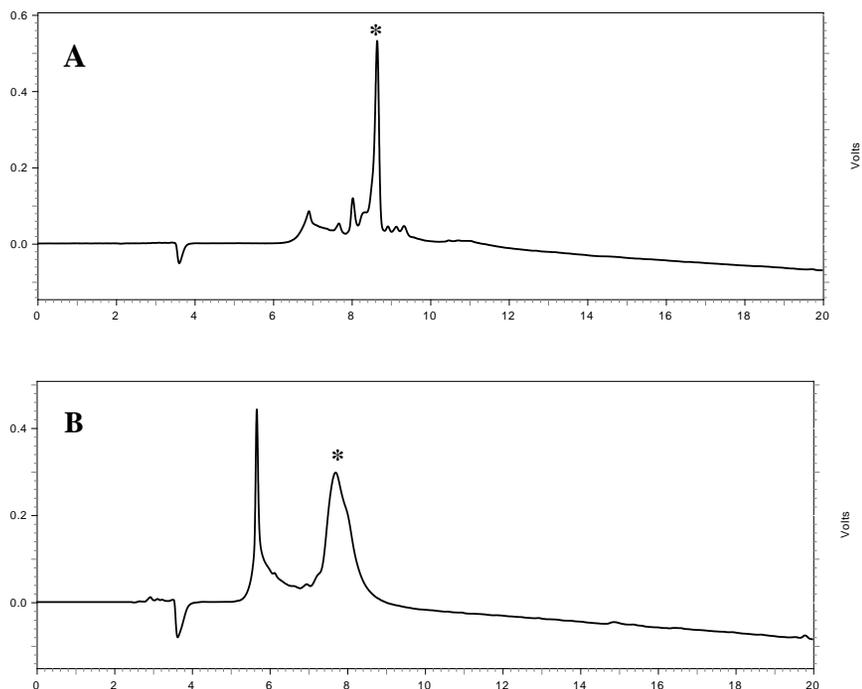
**Figure 6.** **A** - RP-HPLC chromatogram of the first generation G1 dendrimer. **B** - RP-HPLC chromatogram of the fifth generation G5 dendrimer. The eluent system was: **A** - 0.1% trifluoroacetic acid in water, **B** - acetonitrile. The linear gradient 0-50% of **B** in 20 min was used (1 ml/min).
