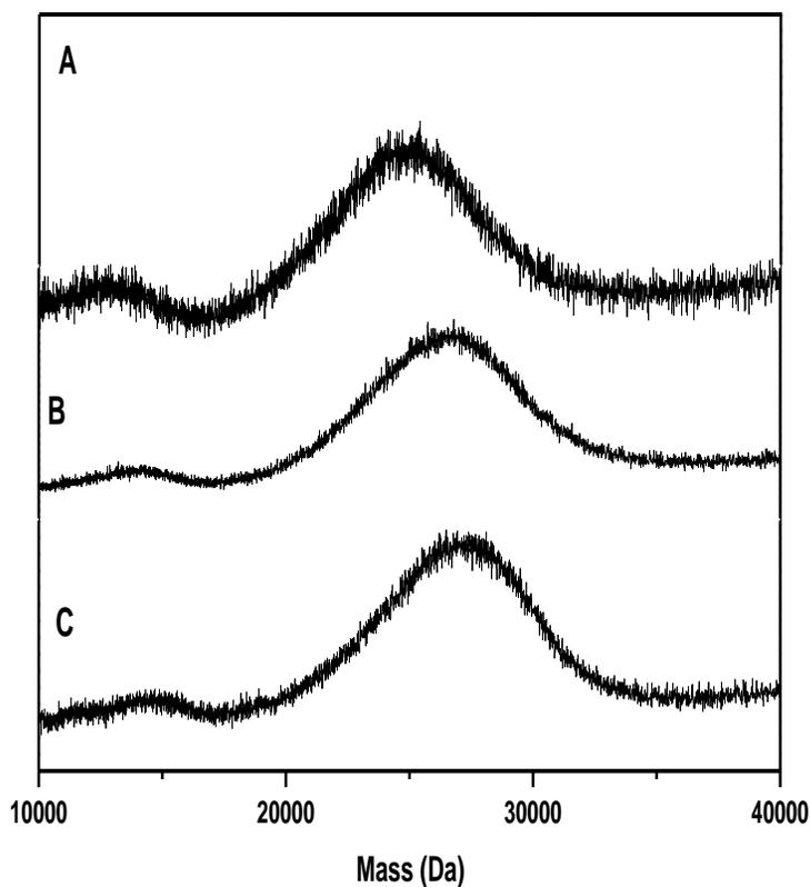
**Figure 11.** MALDI-TOF MS spectra of the fifth generation of PAMAM dendrimers (A), dendrimers modified with *N*-methylethylenediamine (B) and dendrimers modified with *N,N*-dimethylethylenediamine (C).
