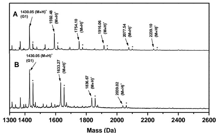
**Figure 14.** MALDI-TOF MS spectra. **A** – the reaction mixture of the first generation of PAMAM dendrimer and Glc in water solution, **B** - the reaction mixture of the first generation of PAMAM dendrimer and GlcNAc in water solution. \* - corresponding sodium ion.
