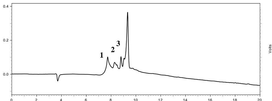
**Figure 19.** RP-HPLC chromatogram of the reaction mixture containing 16-mer oligosaccharide of HA (**1**), G1 dendrimer (including defective molecules) (**2**), corresponding conjugate of G1 dendrimer and oligosaccharide (**2**) and modifications of oligosaccharide (**3**) (Scheme 20).
