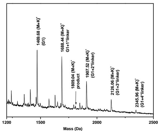
**Figure 25.** MALDI-TOF MS spectrum that shows the ratios of the product (G1 dendrimer+SMCC+Cys) and various impurities in the reaction mixture.
