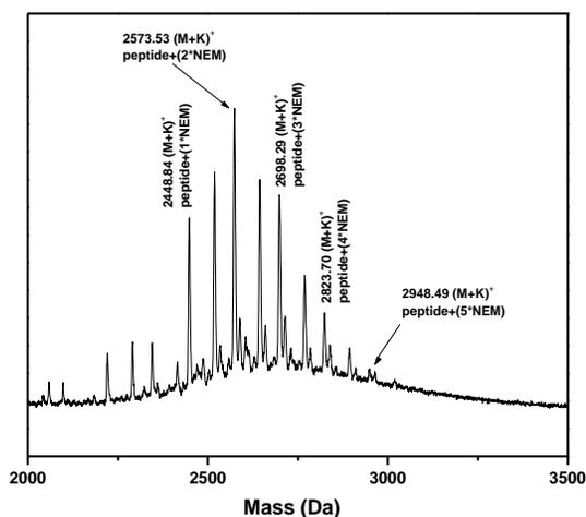
**Figure 26.** MALDI-TOF MS spectrum of the reaction products between *N*-ethylmaleimide (NEM) and peptide.
