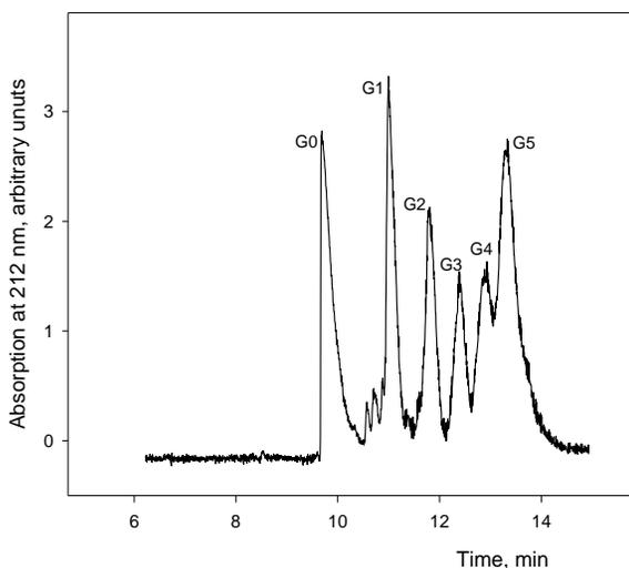
**Figure 8.** Electropherogram of the first six generations of EDA-core PAMAM dendrimers.
