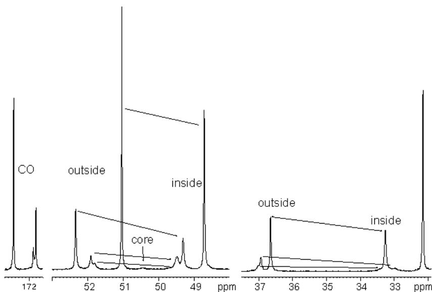
**Figure 9.** 125.77 MHz  $^{13}\text{C}$  NMR spectrum of EDA core based PAMAM G2.5 dendrimer in  $\text{CDCl}_3$ . Indicated by arrows are pairs of connected methylene carbons. Inside the carbons there are broad lines. The assignment of lines is given in [III, Table 1].
