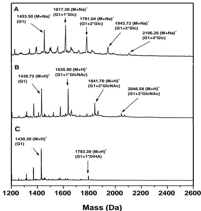
**Figure 17.** MALDI-TOF MS spectra of the crude products after the reduction of Schiff base between G1 dendrimer and various glycosides (**A** – Glc, **B** – GlcNAc, **C** – DiHA) with NaCNBH<sub>3</sub>.
