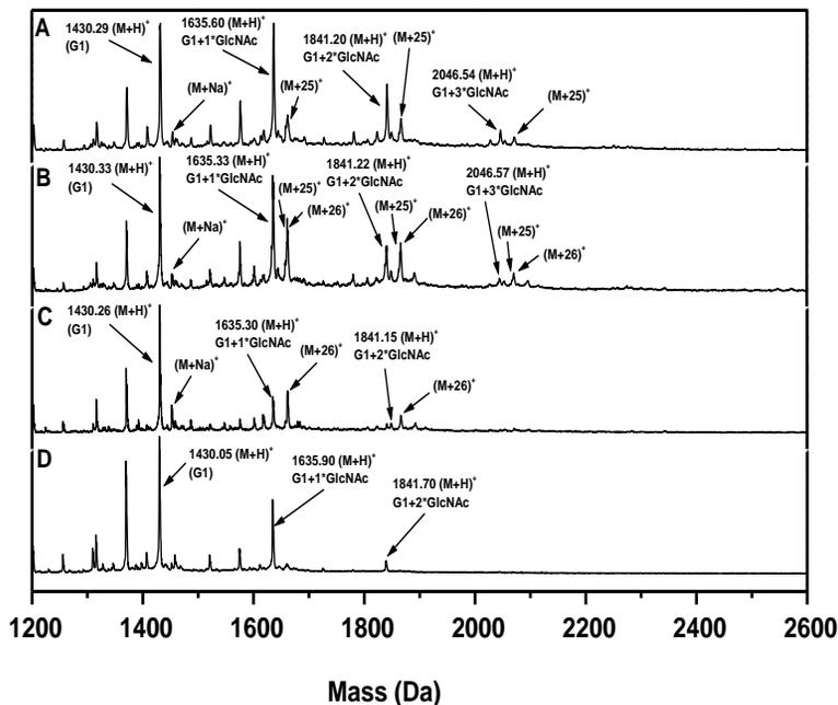
**Figure 16.** MALDI-TOF MS spectra characterizing the ratio between reaction products and impurities in the reaction mixture during the reduction of Schiff base between G1 and GlcNAc with NaCNBH<sub>3</sub>.
