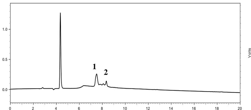
**Figure 21.** RP-HPLC chromatogram of a reaction mixture containing 16-mer oligosaccharide of HA (**1**), G1 dendrimer (including defective molecules) (**2**), corresponding modification of the conjugate of G1 dendrimer and oligosaccharide (**2**), modifications of G1 dendrimer and modifications of oligosaccharide (**2**) (Scheme 20 and 23). The eluent system was: **A** - 0.1% trifluoroacetic acid in water, **B** - acetonitrile. The linear gradient 0-50% of **B** in 20 min was used (1 ml/min).
