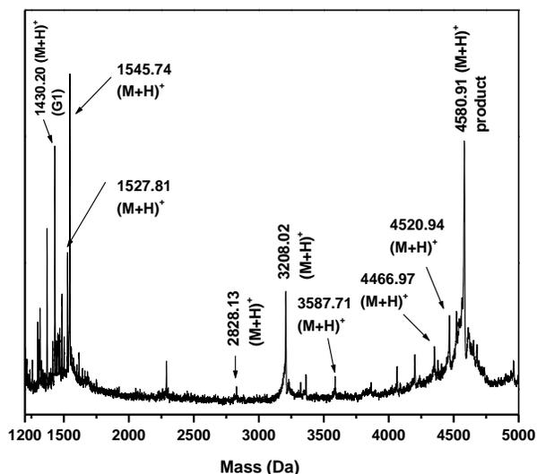
**Figure 22.** MALDI-TOF MS spectrum of the purified conjugate of G1 dendrimer and 16-mer oligosaccharide. The fraction contains various modifications of 16-mer oligosaccharide and G1 dendrimer as impurities (Scheme 20, 23).
