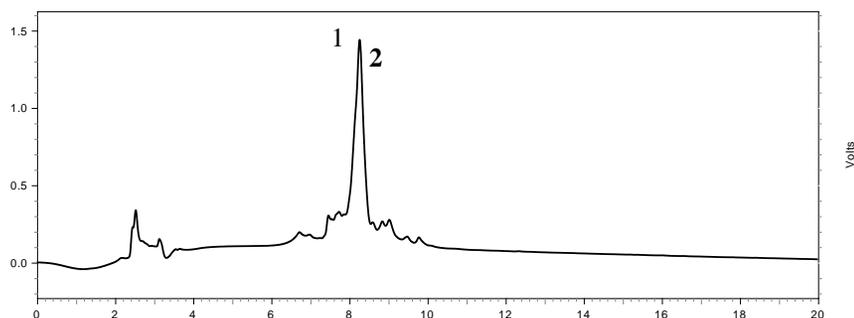
**Figure 18.** RP-HPLC chromatogram of the reaction mixture containing G1 dendrimer (including defective molecules) (**1**) and the corresponding conjugates of G1 dendrimer and GlcNAc (**2**). The eluent system was: **A** - 0.1% trifluoroacetic acid in water, **B** - acetonitrile. The linear gradient 0-50% of **B** in 20 min was used (1 ml/min).
