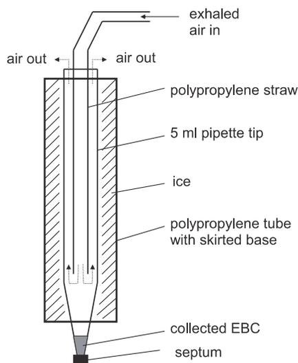
Fig. 1. Schematic of an in-house constructed EBC collection device.
