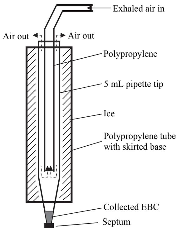
**Figure 4. Scheme of an in-house constructed EBC collection device.**
