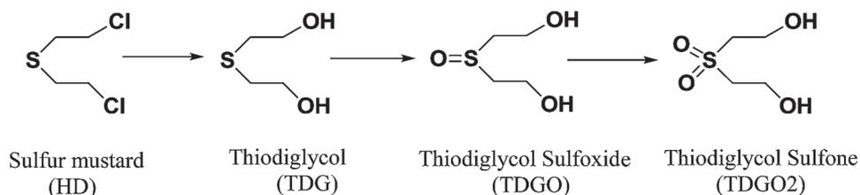
**Figure 2. Hydrolytic pathways of sulfur mustard**
