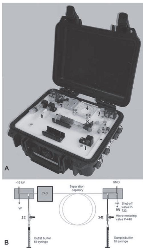
**Figure 1.** (A) A photo of the portable instrument (1) syringe socket, (2) shut off valve, (3) inlet end of the capillary, (4) the separation capillary, (5) outlet end of the capillary, (6) syringe socket, (7, 8) metering valve. (B) A schematic of the separation compartment of the portable instrument ("W" – output to waste, GND – grounding, S-I and S-II – interfaces, micro flow-metering valves (P-446)).
