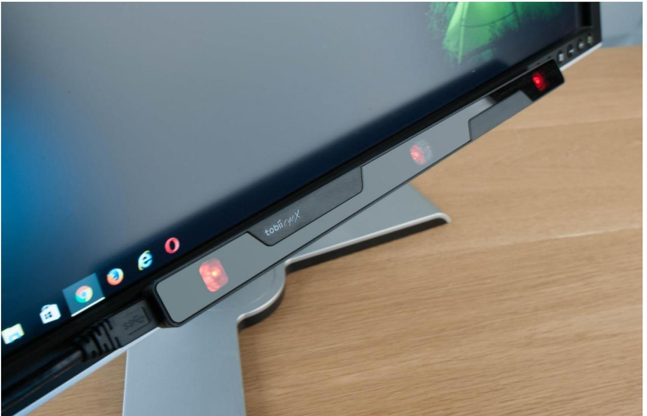
Figure 15 Mounting of the EyeX controller (Source: <http://www.pcworld.com/article/3014523/peripherals/tobii-eyex-review-the-eye-mouse-is-magical-but-just-not-for-everyone.html>)
