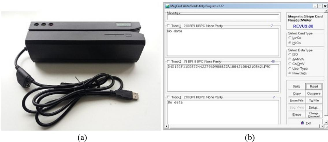
Figure 5. The MSR605 (a) and accompanying software (b)
