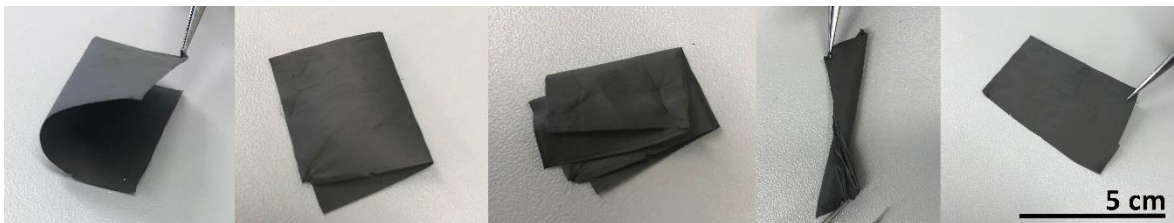
Figure 3.12. Bending, folding and twisting operations performed on SAN + IL + SiC method 2 membrane. The last photo was taken of the same sample after performing these operations, the scale bar corresponds to 5 cm on the last photo, thickness of the membrane was 40 \mu\text{m}
