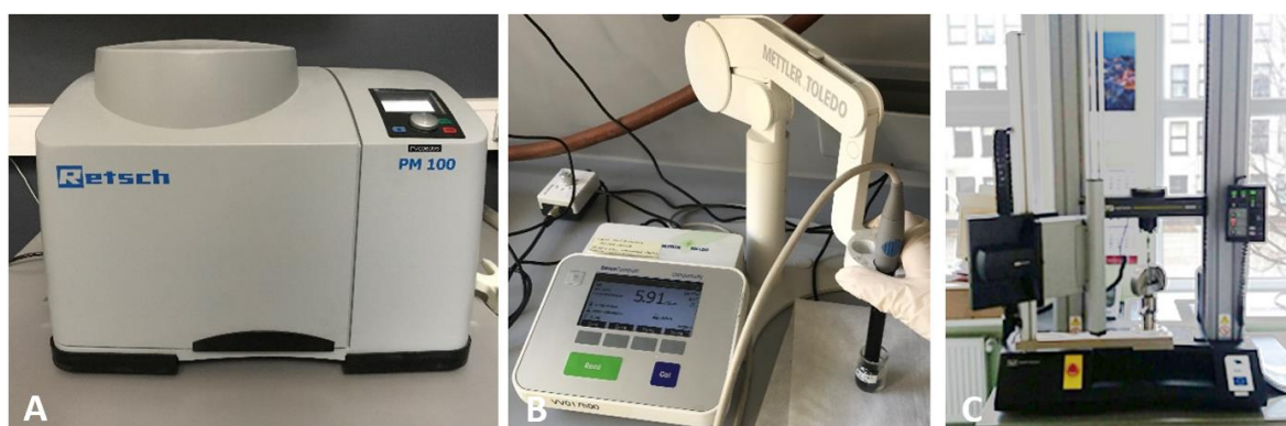
Figure 2.1. Used instruments: A – planetary ball mill, B – solution conductivity meter, C – tensile tester
