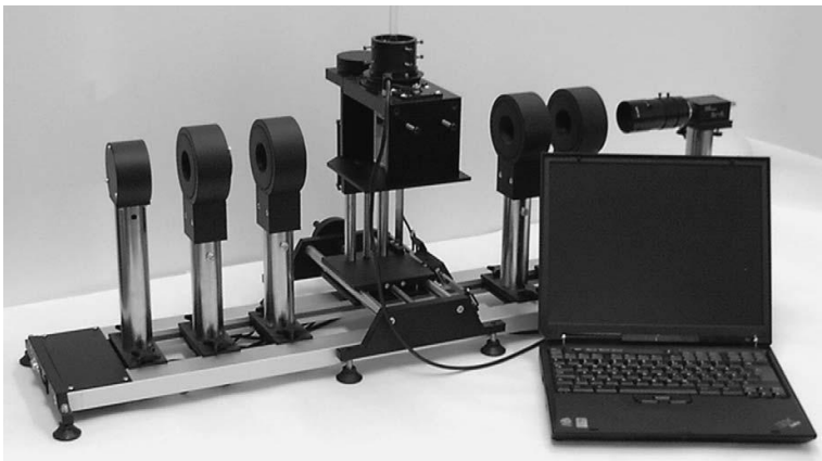
Fig. 2: Computer-controlled polariscope AP-04 SM. In the middle is the rotary stage with an optical fiber preform
