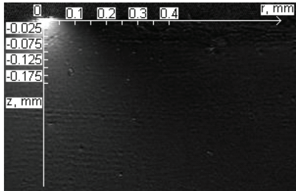
Fig. 22: Image of the soda-lime fibre under spherical indenter in a white-field circular polariscope.
