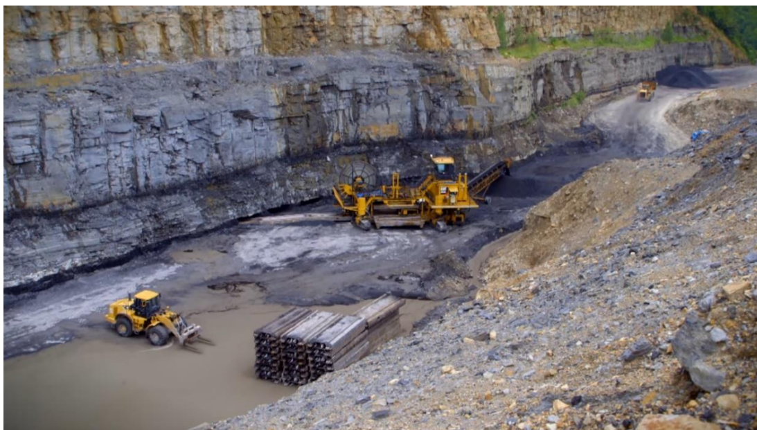
Joonis 9. Cat HW300-ga kiviõe raimamine. Allikas: https://www.youtube.com/watch?v=l6nlWxzRQ8o&t=173s
