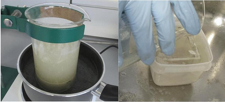
Figure 2.3 Manufacturing of gelatine based phantom material.
