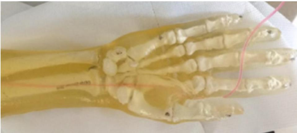
Figure 2.2 Forearm phantom prepared for EBI measurement [4].
