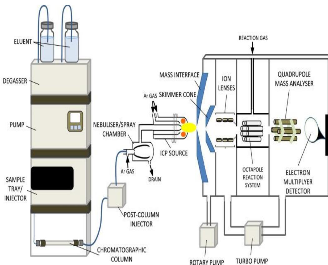
Figure 3. A Brief Overview of LC-ICP MS instrumentation (Delafiori, Ring et al. 2016).
