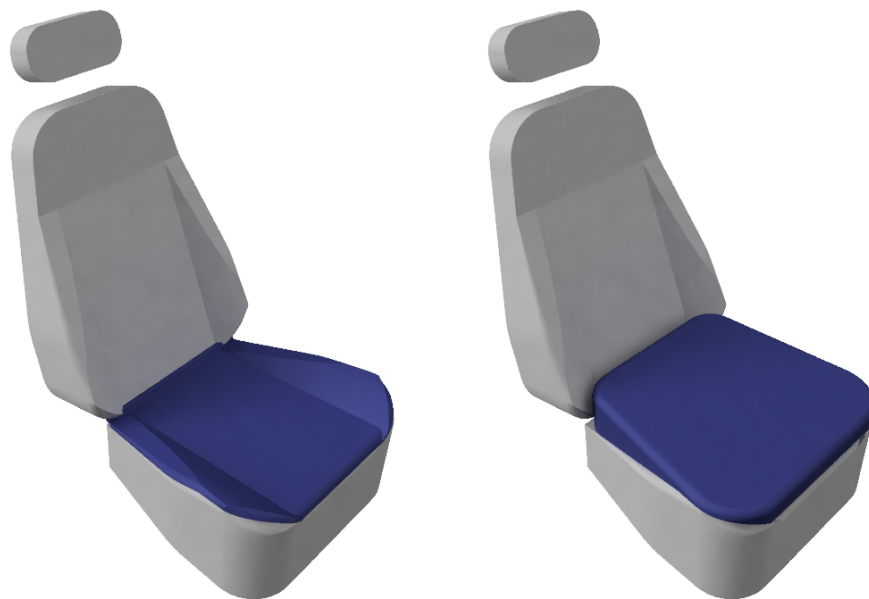
Figure 7.2: Lifting pillow in deflated and inflated states. (CAD drawing made and rendered with Autodesk Fusion)
