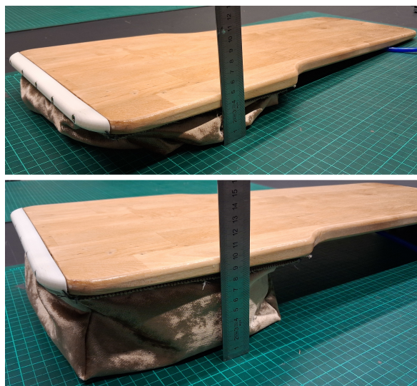
Figure A.6: Height of the device in deflated state is approximately 50 mm, in inflated state approximately 100 mm
