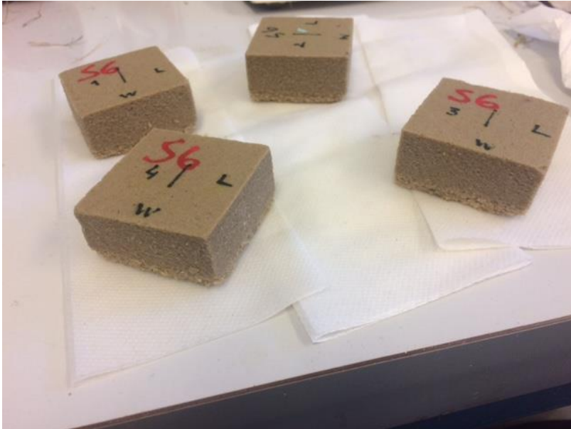
Figure 24. Specimens after immersion in water
