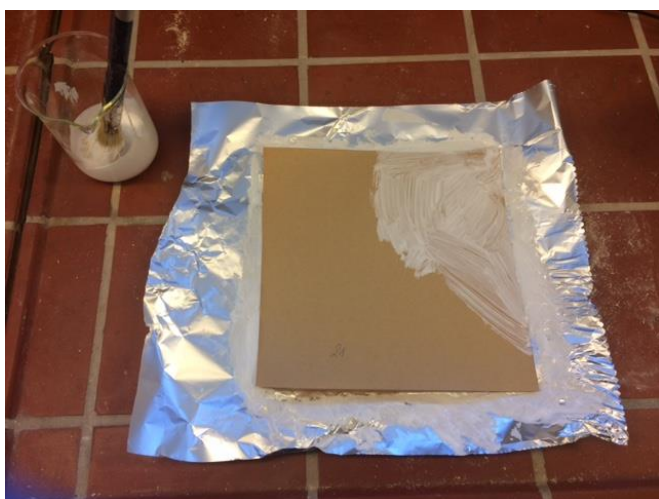
Figure 17. Adding PVA glue to kraft paper
