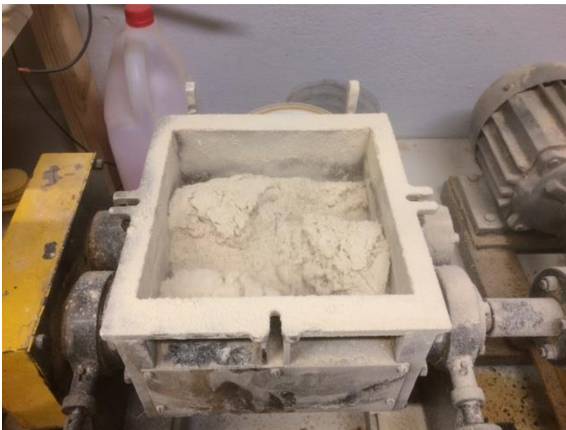
Figure 13. Mixing the hemp flour with adhesive
