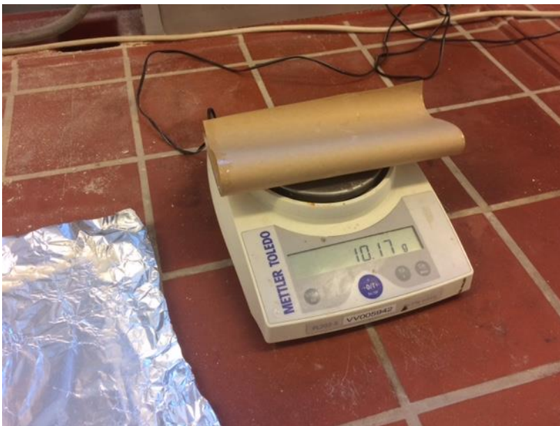
Figure 16. Weighting after gluing
