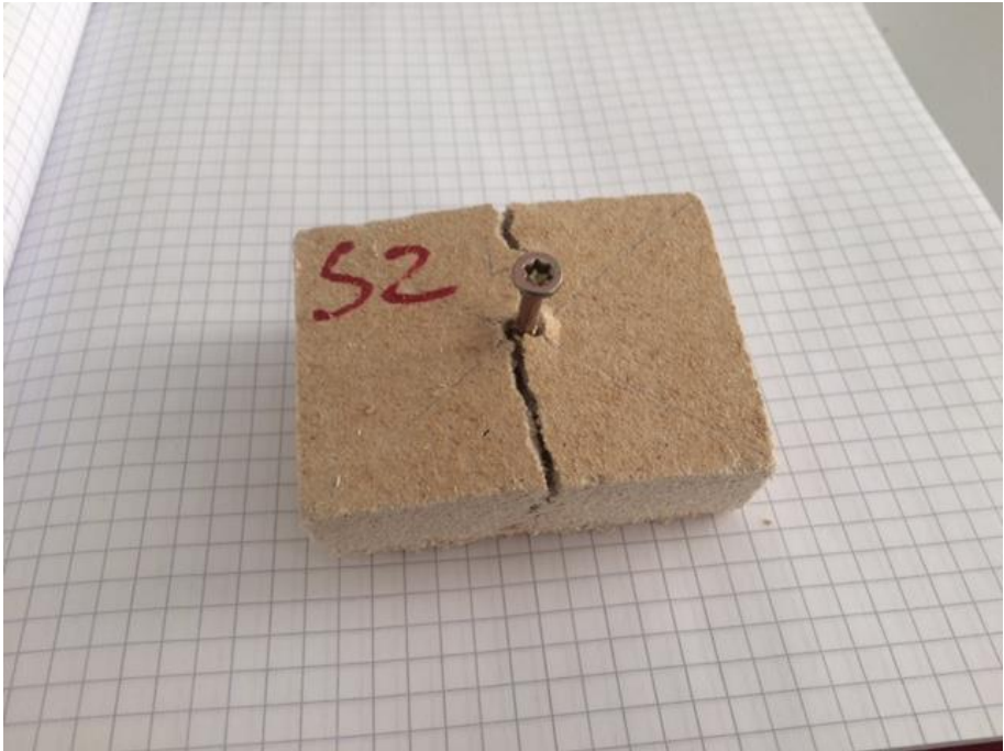
Figure 34. Sample made by wet method broke during the test
