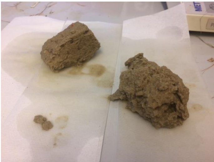
Figure 30. Hemp fiberboard made by dry method after soaking
