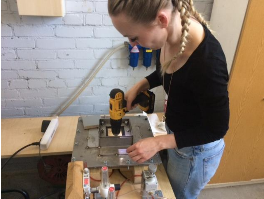
Figure 27. Fixing specimen into the rig
