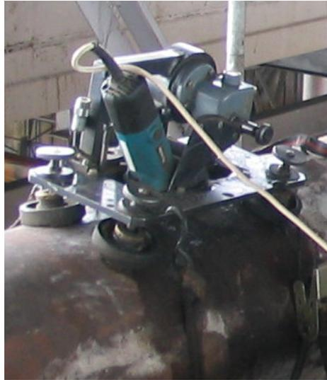
Figure 2.8. Device MSM-1 for sampling from external surface of power plant components
