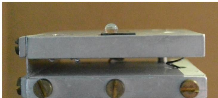
Figure 5.29 Hydrophobic properties of treated black silicon
