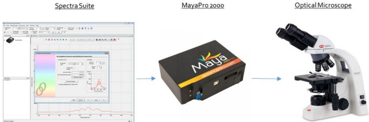
Figure 5.7 Reflectivity measurement setup
