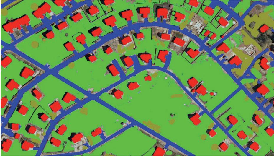
*Figure 14. Classified area from the outskirts (top) and the feature masks (bottom): red for buildings, blue for roads, green for grass and brown for debris*
