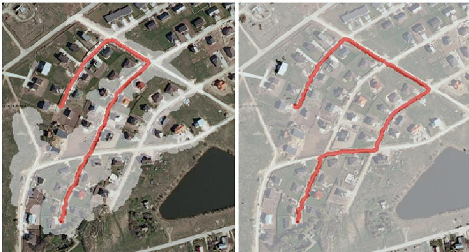
*Figure 32. Path planning in the outskirts – highlighted area marks the nodes used by the path planner. The path on the left image is produced using the well-trained classifier and the path on right image is produced using the under-trained classifier*
