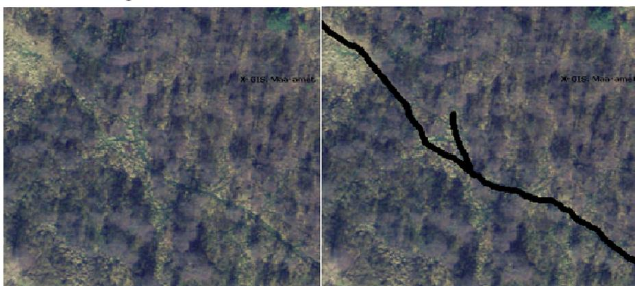
*Figure 29. Overlabeling of the fen: The barely visible track disappears on the harder surface, but manual labeling followed the road using extra clues from the gaps between the bushes, confusing the classifier*
