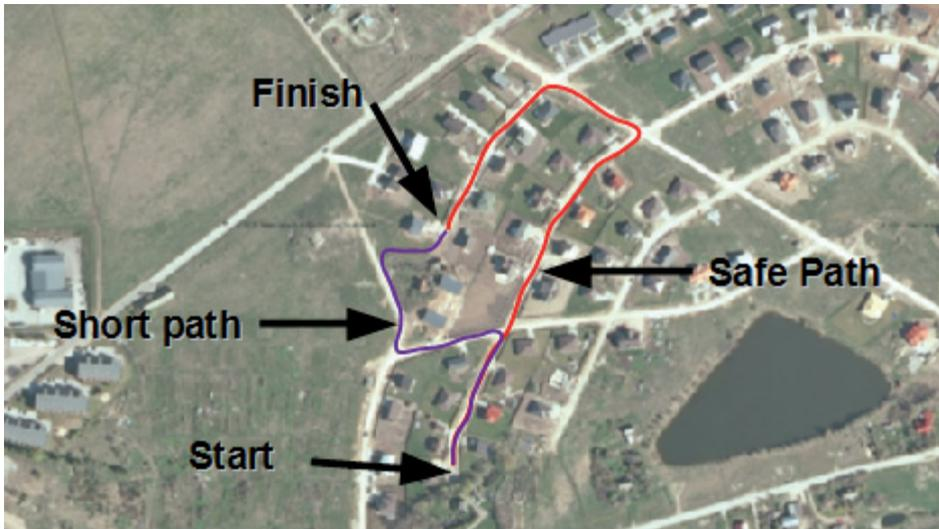
Figure 25. Outskirts test case – the path starts and ends at cul-de-sac. The objective is to generate a path from start location to finish avoiding obstacles and preferring roads. Either one of the hand drawn paths are desirable outputs for the path planner
