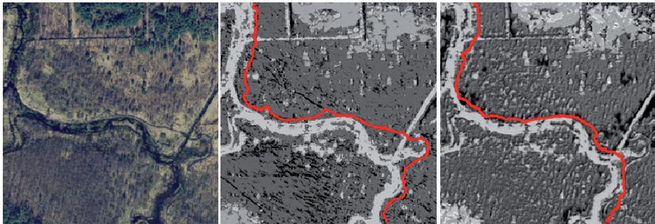
*Figure 31. Cost map generation and path planning in fen using classifier training Method B*
