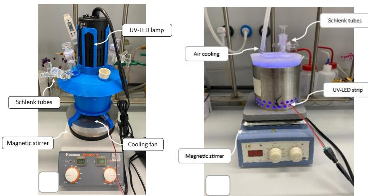
**Figure 4.** Photochemical reactors A and B used for reaction optimization.
