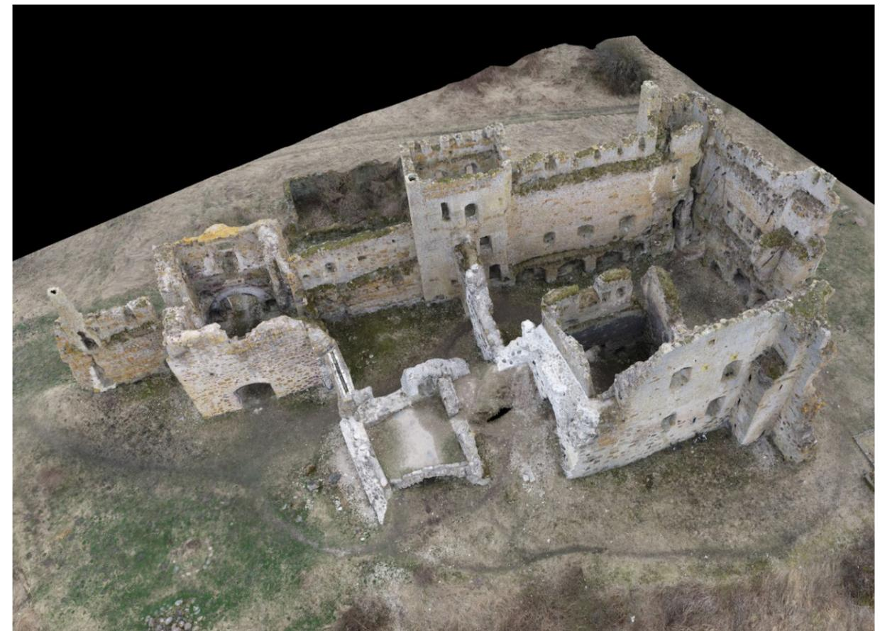
**Illustration 28** The model of the Toolse castle done with photogrammetry with dronedeploy software (by author)
