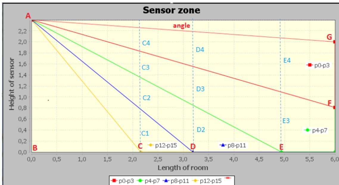
Figure 16 Sensor zones named C, D and E.
