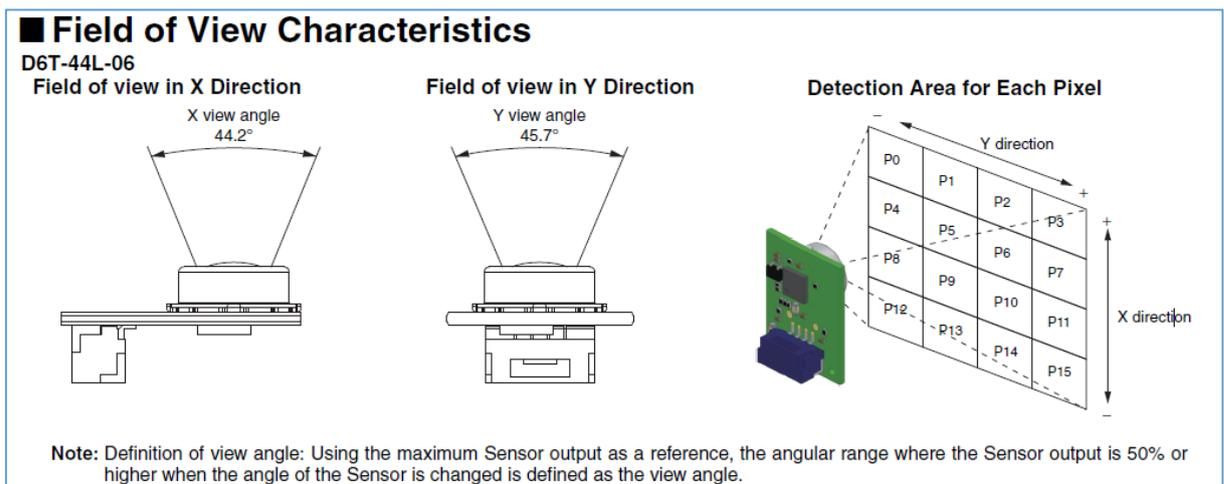
Figure 13 Field of View Characteristics [27].
