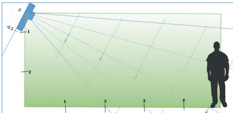
Room 2.4 meter x 4 meter and a person at 7 meter (sensor angle  $26.2^\circ$ )
