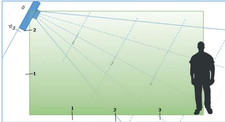
Room 2.4 meter x 3 meter and a person at 7 meter (sensor angle 26.2°)
