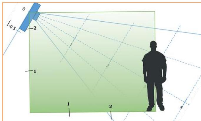
Room 2.4 meter x 2 meter and a person at 7 meter (sensor angle 26.2°)
