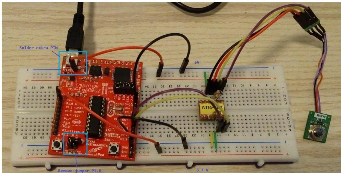
*Figure 4* Image of microcontroller connected to sensor.
