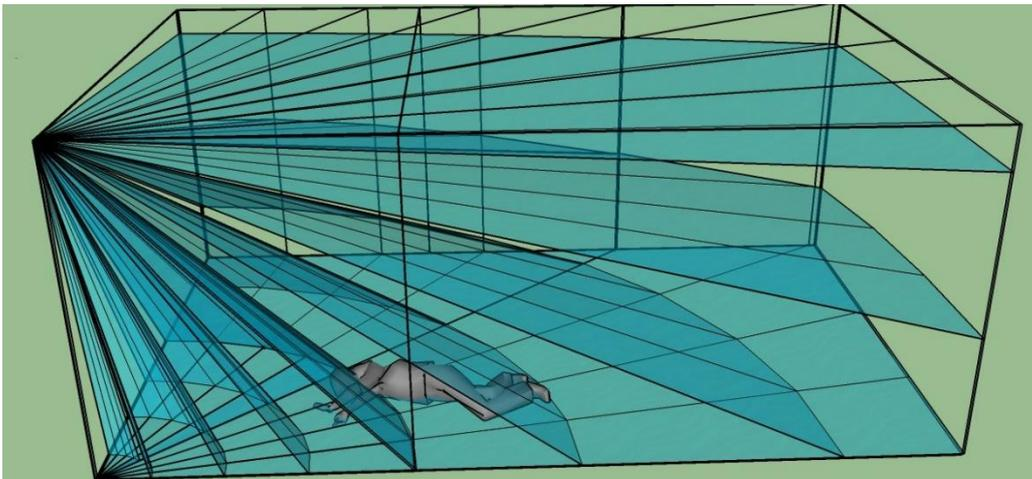
Figure 8 Four sensors covering one room.
