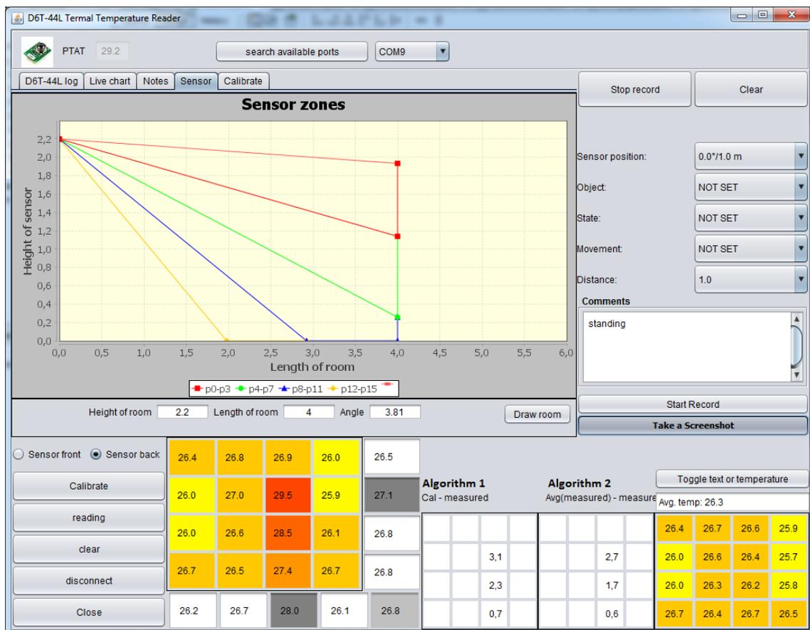
Figure 46 Comparing algorithms of a standing person
