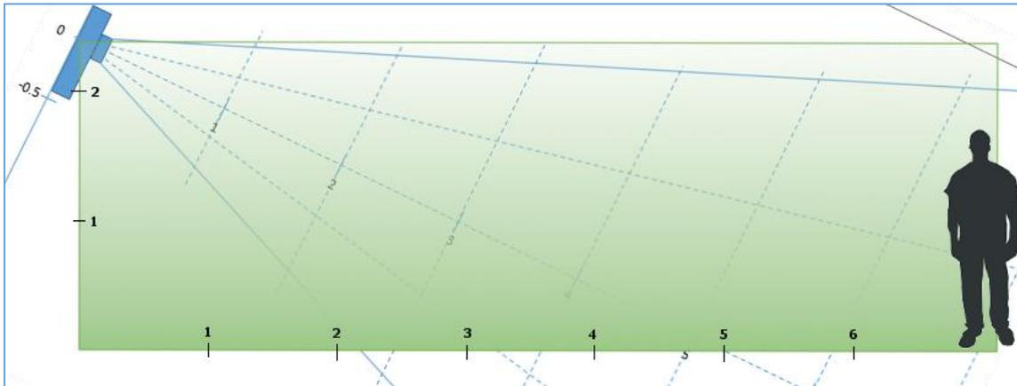
Room 2.4 meter x 6 meter and a person at 7 meter (sensor angle  $26.2^\circ$ )
