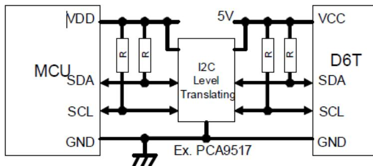
Figure 3 Using I2C logic level converting [29].
