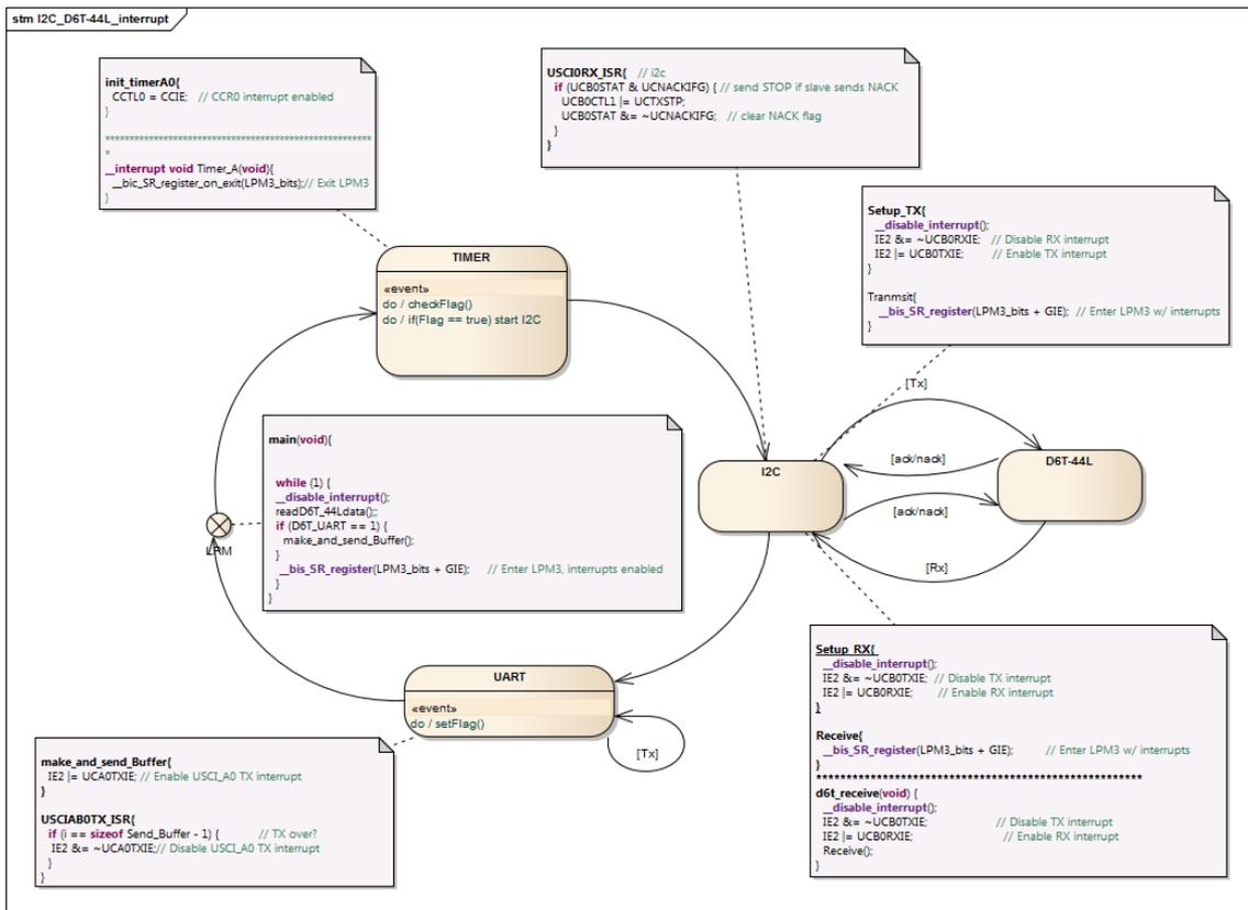
Figure 15 MSP430g2553 Interrupts, Timer, I2C, UART flow.
