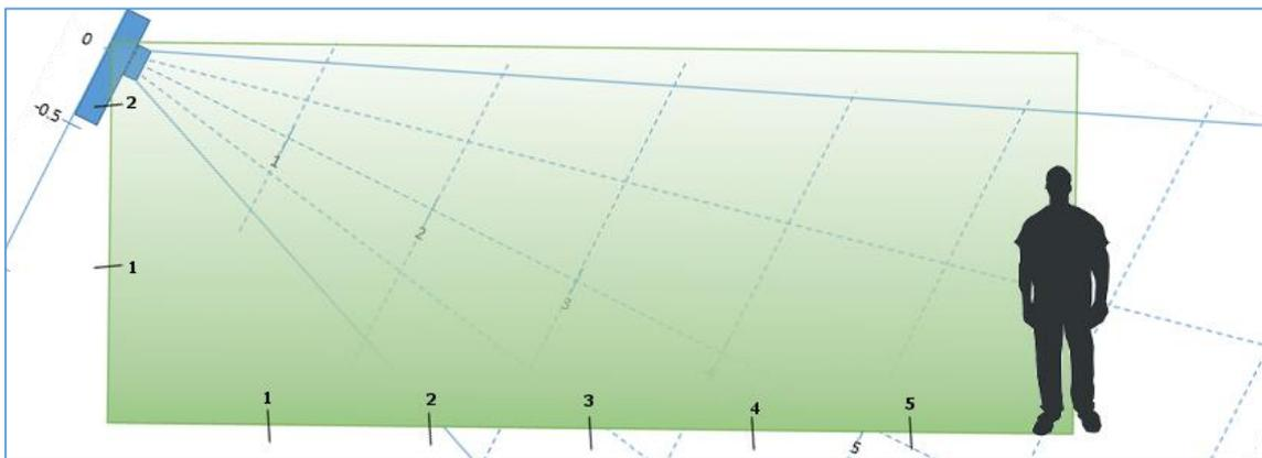
Room 2.4 meter x 5 meter and a person at 7 meter (sensor angle  $26.2^\circ$ )
