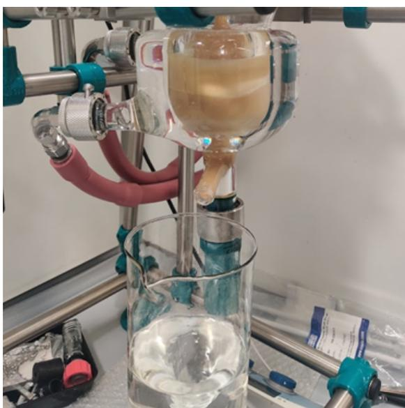
Photo 2.3.1.1 Photo of cellulose stearate stuck in reactor after synthesis, right before washing
