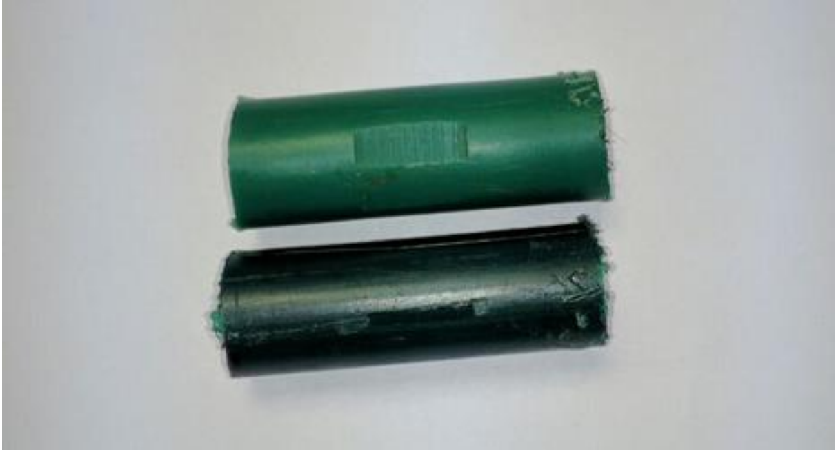
Figure 36. Sample 2 wear (upper) and 10 (lower) after rubbing against wet steel wheel, test duration 10 minutes, load 2.5 kg
