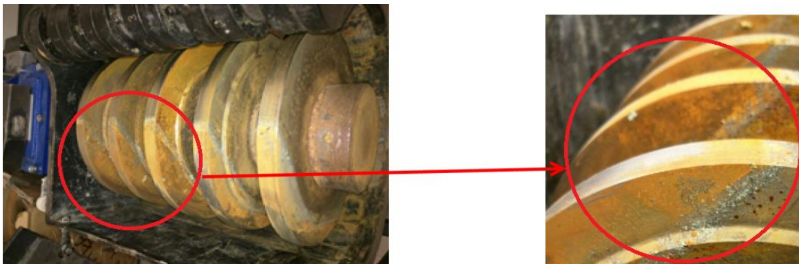
Figure 8. Rust film on steel wheel after wet tests
