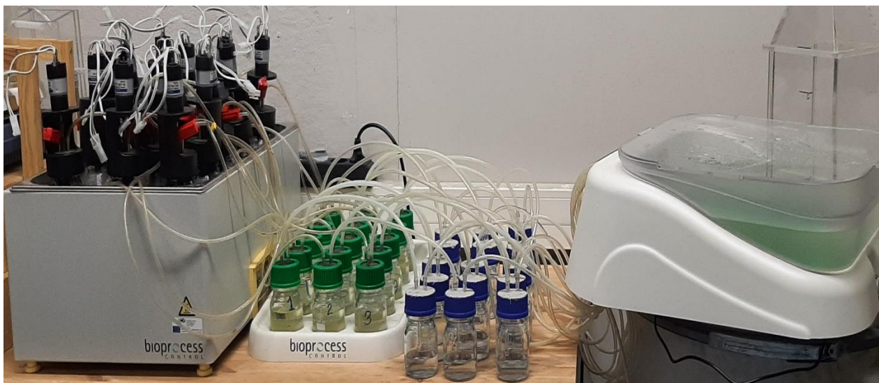
Figure 3.2 AMPTS II showing the incubation unit and the bottles containing alkaline solution.
