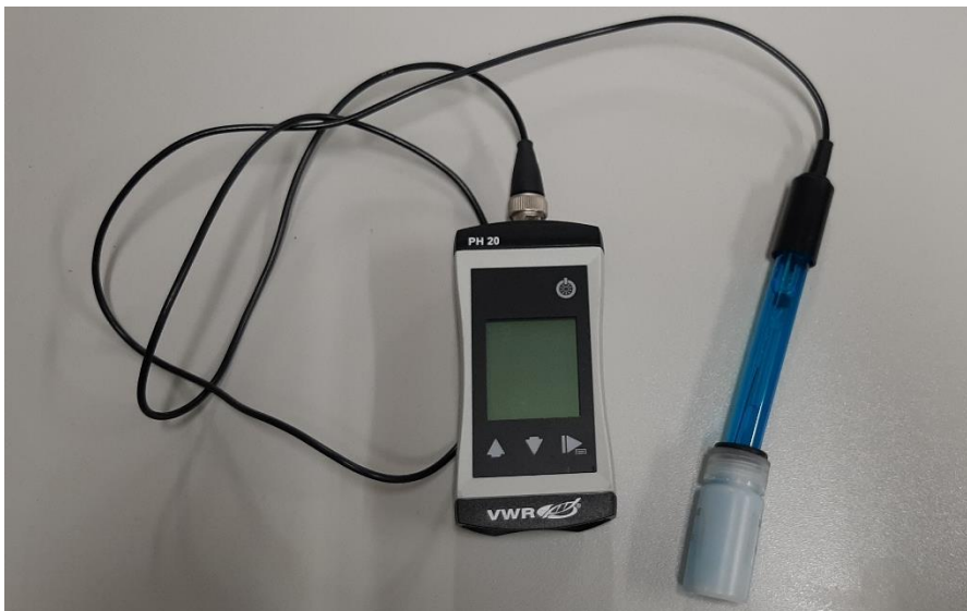
Figure 3.1 pH measuring instrument with electrode
