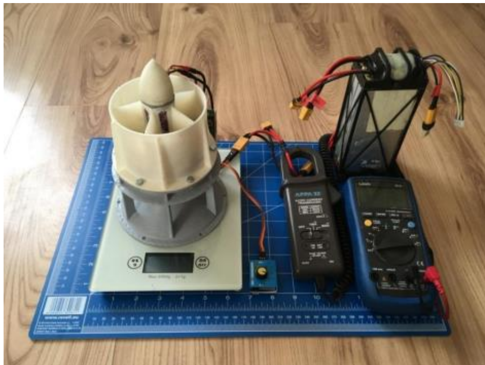
Figure 2.1 The first part of the test apparatus used to analyze engine parameters [2]
