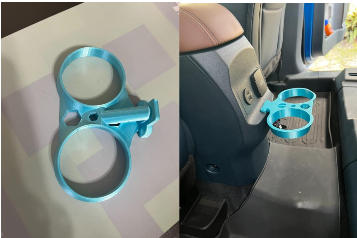
Figure 5.7 Ford Maverick 3D printed cupholder in use. (The Verge, 2023)
