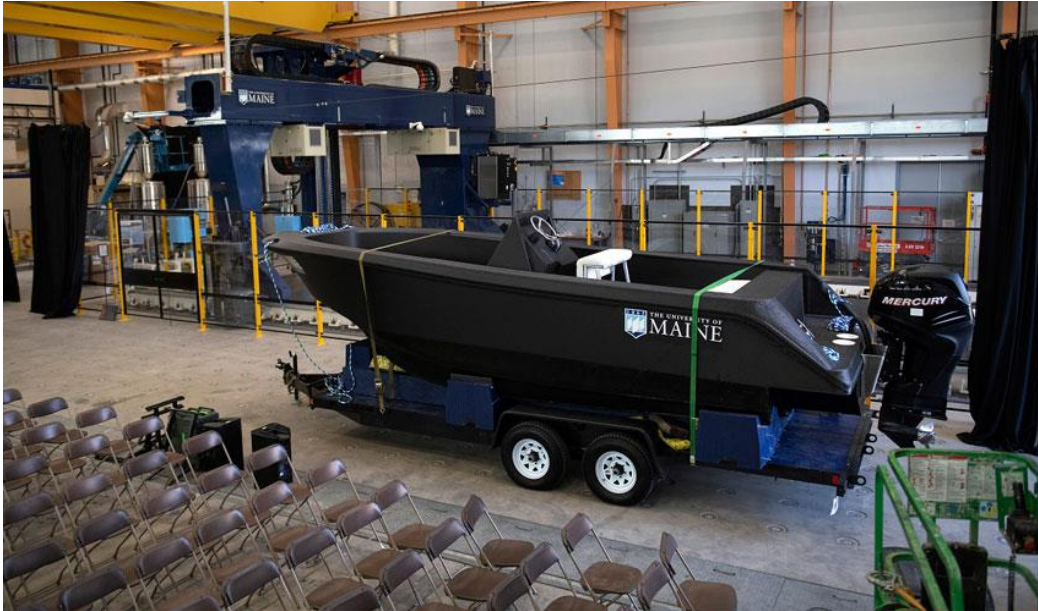
Figure 5.4 3Dirigo - a 3D printed boat; University of Maine. (Guinness World Records, 2023)
