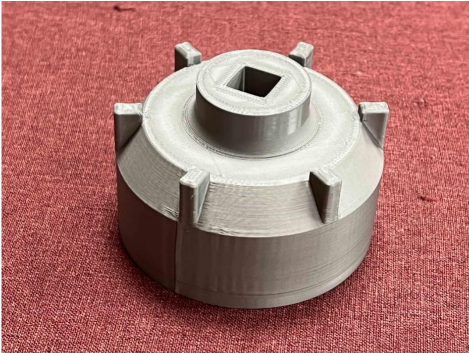
Figure 6.19 Completed 3D printed oil filter wrench (90mm). Picture by Author
