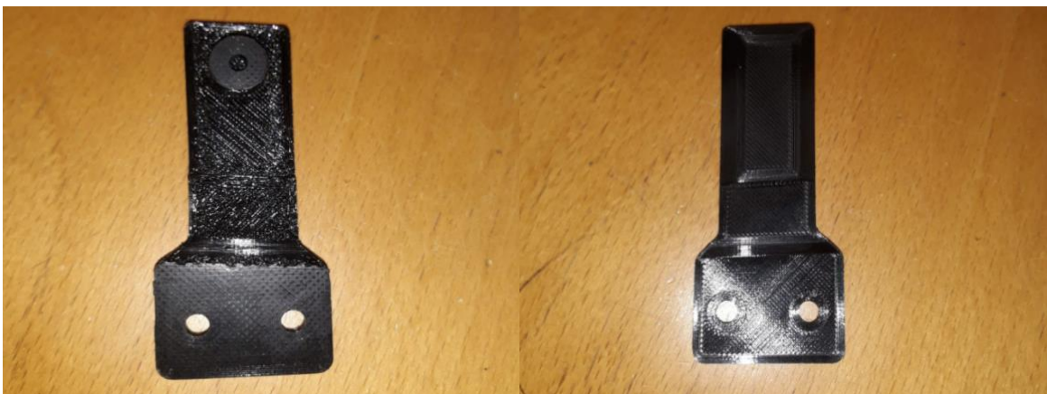
Figure 7.2 3D printed Seat Ibiza windshield clip. Picture by owner of the car
