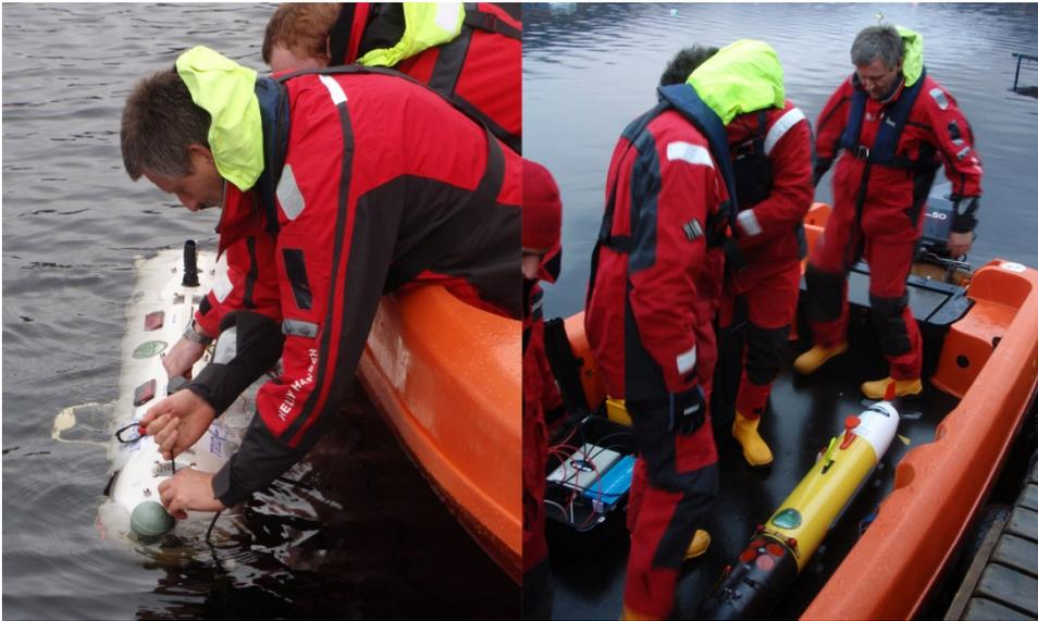
**Figure 1.2** – Left: NESSIE AUV developed by the Ocean Systems Laboratory of the Heriot-Watt University; Right: REMUS 100 AUV by Hydroid.
