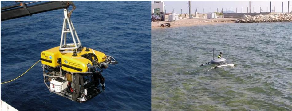
**Figure 1.1** – Left: Typical remotely operated underwater vehicle Hercules ROV being deployed for mission (Public domain, Wikimedia Commons); Right: Autonomous surface vehicle Sonobot designed by Evologics. <sup>1</sup>
