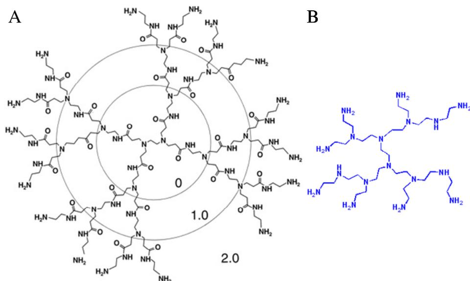
Figure 1.1. Schematic diagram of PAMAM dendrimer (A), generation 2.0, where the successive full generations are indicated by concentric circles (Supattapone et al., 1999), and the scheme of polyethylenimine (B).
