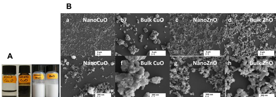
Figure 3.1. Stock solutions (A) and SEM images (B) of nano- and micro-sized CuO and ZnO. Panel A: stock solutions in MilliQ water at 40,000 mg/l. Panel B: images a, b, c and d:  $\times 2000$  magnification; e, f, g and h:  $\times 20\,000$  magnification.
