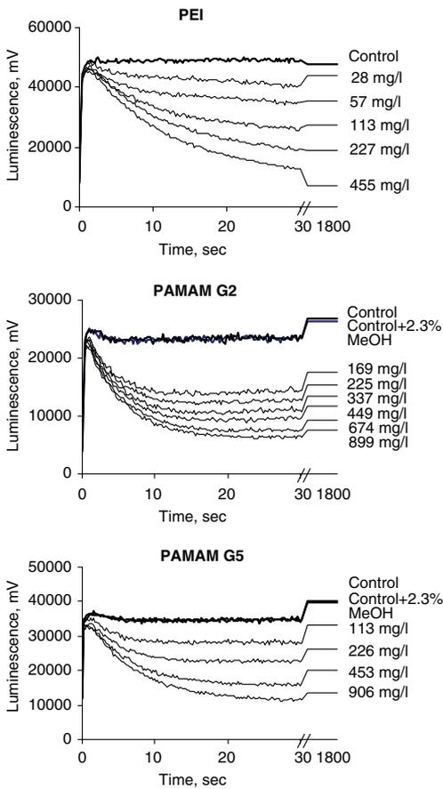
Fig. 2. Kinetics of luminescence of *Vibrio fischeri* exposed to suspensions of PEI, PAMAM G2 and G5 measured in microplate format of Flash Assay. NaCl (2%) served as a control and diluent for PEI and 2% NaCl + 2.3% methanol served as a control and diluent for PAMAM dendrimers.
