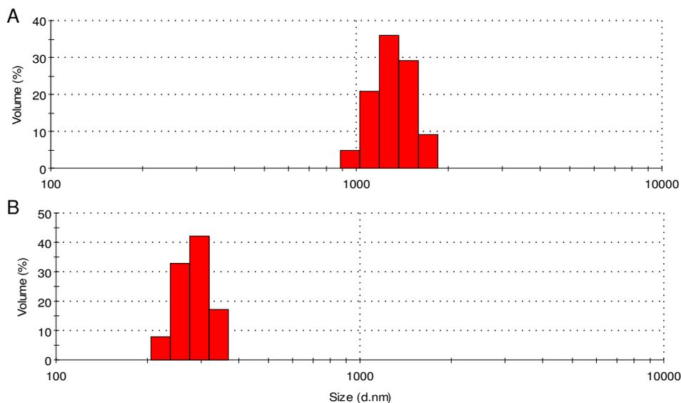
Figure 3.2. Size distribution of nanoCuO by dynamic light scattering. DLS measurement before (A) and after (B) removing the larger particles by centrifugation at 700×g for 5 min. The measurement was done at nanoCuO concentration of 100 mg/l in Osterhout's mineral medium.
