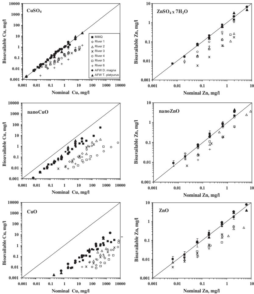
Fig. 1. Nominal (x-axis) versus bioavailable Cu and Zn ions (y-axis) in six natural waters and artificial freshwater (AFW). Dissolved bioavailable metals were quantified by recombinant *Escherichia coli* Cu-sensor (left panel) and Zn-sensor (right panel).
