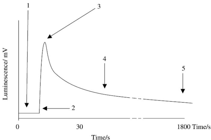
Figure 1.5. Scheme of the Flash Assay. 1 – start measuring and mixing; 2 – inject bacteria; 3 – record peak value from 0-5 s; 4 – record signal for 30 s; 5 – at 30 min, record signal. Modified from Lappalainen et al., 2001.
