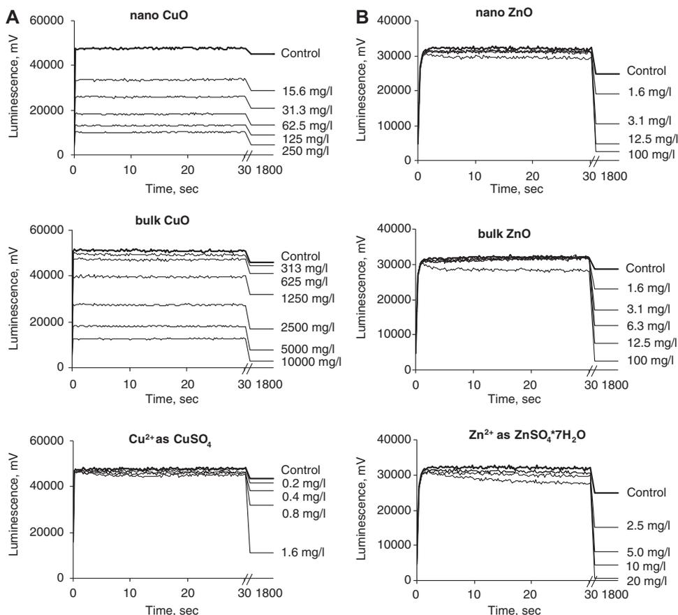
Fig. 1. Kinetics of luminescence of *Vibrio fischeri* exposed to suspensions of nano and bulk CuO and CuSO<sub>4</sub> (A), and nano and bulk ZnO and ZnSO<sub>4</sub> · 7H<sub>2</sub>O (B) measured in microplate format of Flash Assay. NaCl (2%) served as a control and diluent. Concentrations of nano and bulk metal oxides are nominal.
