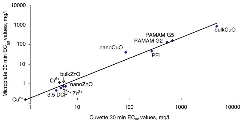
Fig. 3. 30-min  $EC_{50}$  values obtained in *Vibrio fischeri* Flash Assay: cuvette versus microplate format. Equation for the log-log regression line:  $y = 1.05x + 0.007$  and  $\log - \log R^2$  value 0.98.
