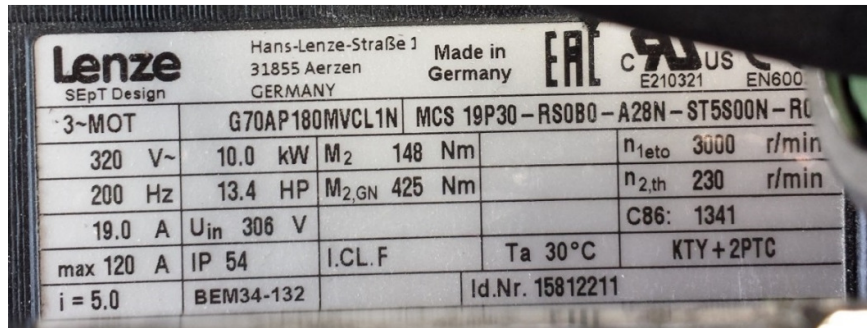
Figure 29, Motor name plate data.
