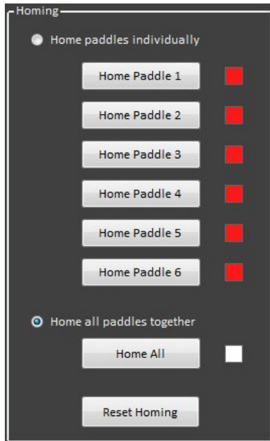
Figure 67. Wave Generator paddle homing command buttons
