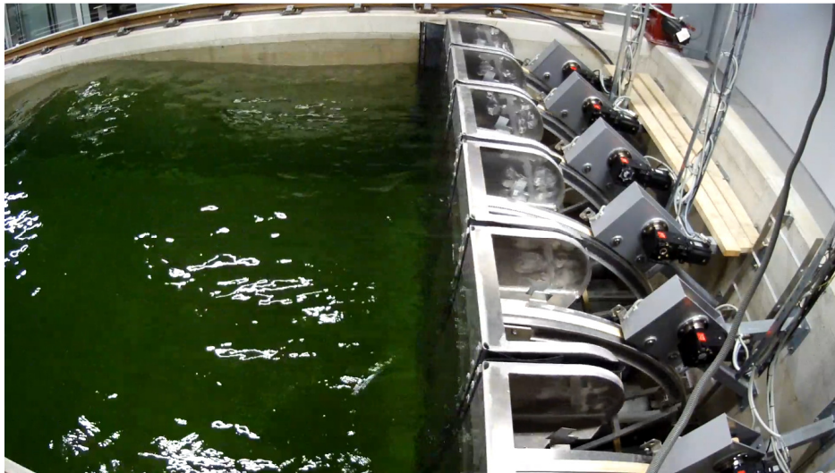
Figure 44. Wave generator at small craft competence centre.
