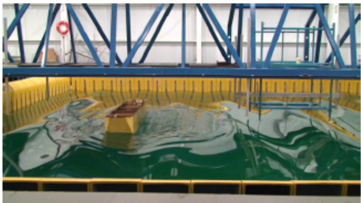
Figure 6. Wave test basin at University of Sao Paulo [18].
